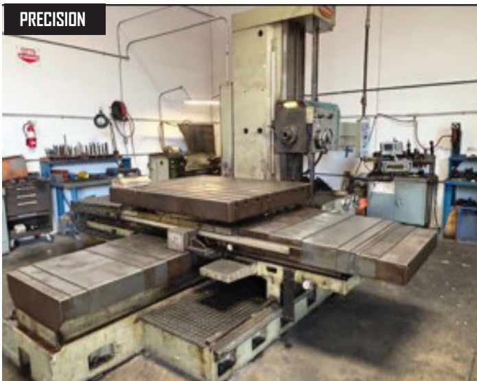
Shibaura BT-10B-R3PD Horizontal Boring Mill s/n 123451 w/ Acu-Rite DRO, 20-1000 RPM, 50-Taper 3.94" Spindle, 28" Z Travel, 55" x 63" Full Rotary Table, 59.1" x 70.9" Travels.
