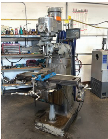
Bridgeport (Head) Alliant (Body) Vertical Mill s/n 75047235 w/ Newall DP-700 Programable DRO, 1.5Hp Motor, 60-4200 Dial Change RPM, Chrome Ways, Power Feed, 9" x 42" Table.
