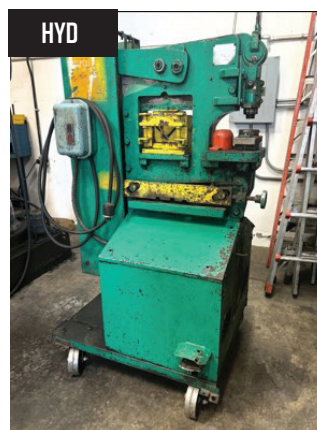
Uni-Hydro 42-14 42-Ton Hydraulic Iron Worker s/n 3P918 w/ Punch w/ 6" Throat, 3" x 3" x 5/16" Angle Shear, 3/8" x 14", 1/2" x 10", 5/8" x 6" Flat Shear.
