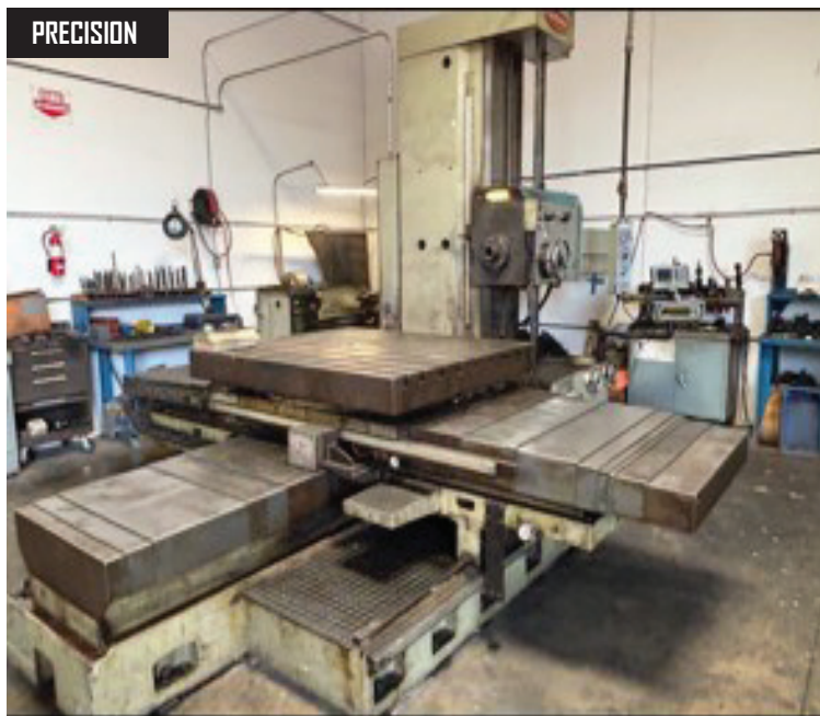
Shibaura BT-10B-R3PD Horizontal Boring Mill s/n 123451 w/ Acu-Rite DRO, 20-1000 RPM, 50-Taper 3.94" Spindle, 28" Z Travel. 55" x 63" Full Rotary Table, 59.1" x 70.9" Travels.
