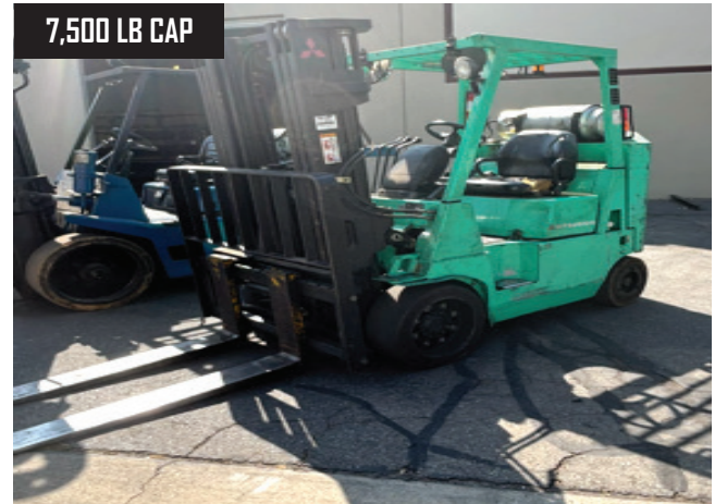
Mitsubishi FGC40KSTC 7500 Lb Cap LPG Forklift s/n AF8700597 w/ 3-Stage Mast, 163" Lift Height, Side Shift, Cushion Tires, 5490 Hours
