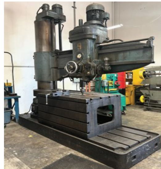
Archdale 18" Column x 60" Radial Arm Drill w/ 1500 Max RPM, Power Column and Feeds, 36" x 60" x 30" Tooling Fixture Block
