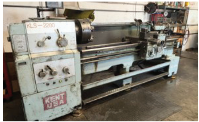
Kent KLS-2280 22" x 80" Geared Head - Gap Bed Lathe w/ Newall DP-700 Programmable DRO, 16-1600 RPM, Inch/mm Threading, 3 1/4" Thru Spindle Bore, Tailstock, Steady and Follow Rests, KDK Tool Post, 15" 6-Jaw Chuck, 16" 4-Jaw Chuck, 12" and 10" 3-Jaw Chucks.
