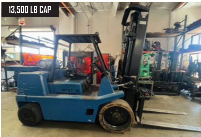
Hyster S135XL 13,500 Lb Cap LPG Forklift /s B024D02085M w/ 3-Stage Mast, 218" Lift Height, Monotrol Trans, Parker Accumulator, Cushion Tires, 4,382 Hours.
