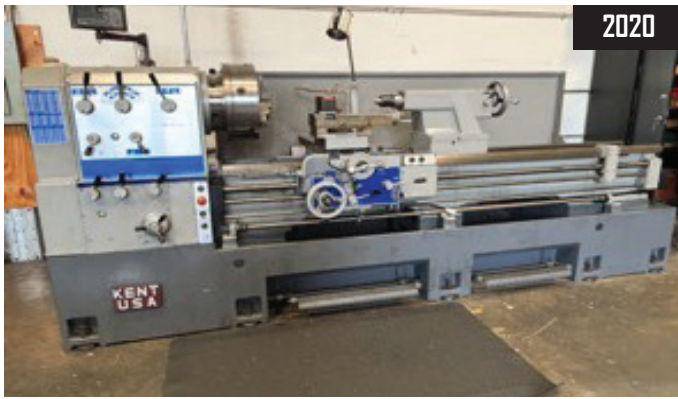
2020 Kent HW-2680 26" x 80" Geared Head - Gap Bed Lathe s/n 9010230 w/ Newall DP700 Programmable DRO, 10-1000 RPM, Inch/mm Threading, 4 1/2" Thru Spindle Bore, Tailstock, Steady and Follow Rests, KDK Tool Post, Indexing Tool Post, 16" 3-Jaw Chuck, Coolant
