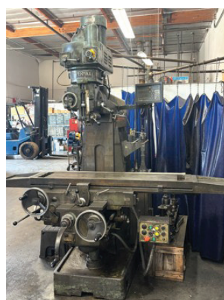
SuperMax Series 2 Vertical Mill w/ Newall DP-7—Programmable DRO, 75-4220 Dial RPM, 40-Taper Spindle, Box Ways, Power Feeds, 11" x 51" Table
