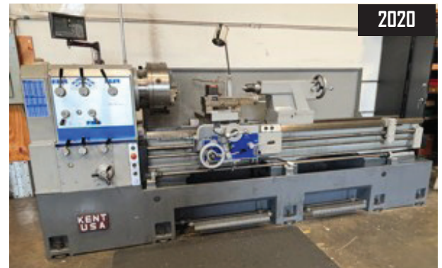
2020 Kent HW-2680 26" x 80" Geared Head – Gap Bed Lathe s/n 9010230 w/ Newall DP700 Programmable DRO, 10-1000 RPM, Inch/mm Threading, 4 1/2" Thru Spindle Bore, Tailstock, Steady and Follow Rests, KDK Tool Post, Indexing Tool Post, 16" 3-Jaw Chuck, Coolant
