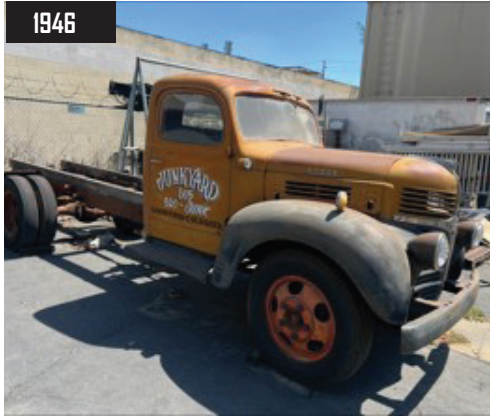
1946 Dodge Flat-Head 6 Grain Truck Lisc N15 764 w/ 4-Speed Trans, 2-Sped Drive Shaft.
