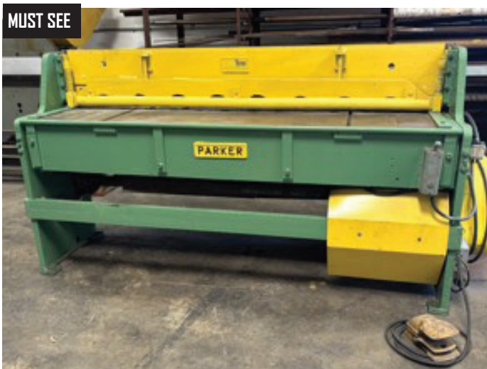
Parker mdl. 1472 14GA x 72" Power Shear s/n 138. Chicago size 250 6' Mechanical Press Brake s/n L2120 w/ Manual Back Gaging, 72" Bed Length, 6" Throat Depth, 49" Between Uprights.
