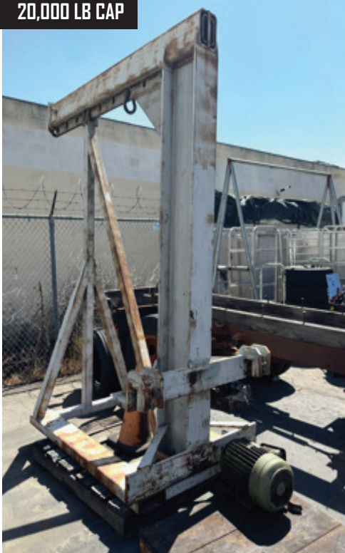
20,000 Lb Cap Forklift Boom Attachment.
