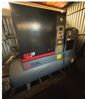
2006 Chicago Pneumatic QSR15 HPD 15Hp Rotary Air Compressor s/n CAI 201254 w/ Built-In Refrigerated Air Dryer, 120 Gallon Tank.
