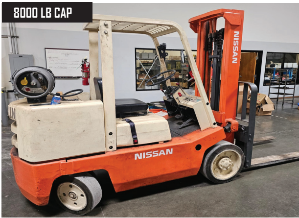
Nissan CHF03 8000# Capacity LPG Forklift, 2 Stage Mast, 60" Forks, Cushion Tires s/n CHF03-000124
