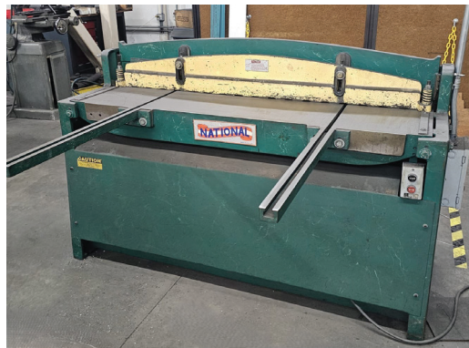
National Sheet Metal Machines NH5216 Hydraulic Shear, 52" X 16 Ga. Capacity, Manual Back gauge, Foot Control, s/n 529-394
