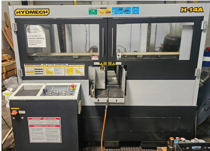
Hyd-Mech H-14A Fully Enclosed Automatic Horizontal Band Saw, 14"x14" Cutting Capacity, 13.6HP, 49-380 SFM Variable Speed, 15'2" x 1'25" Blade, Elevation TS 50 Controls, s/n 5-09-17-217-SB
