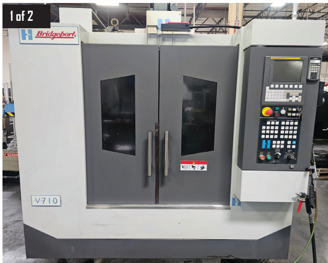
1 of 2) Hardinge / Bridgeport V710 3-Axis CNC Vertical Milling Machine, Travels 27"x15"x16" (XYZ), 31.5"x15" Table, 10HP, 10000RPM Max Spindle Speed, 20 ATC, Fanuc 0I-MF Controls
