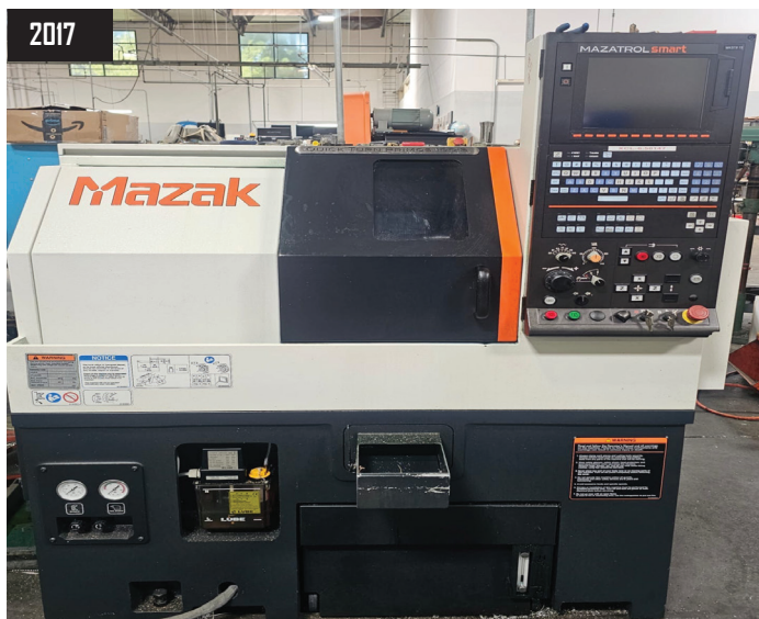
2017 Mazak Quick Turn Primos 100 S CNC Lathe, 5C Collet Spindle, 17.48" Max Swind, 7'87" Max Turning Length, Travels X-Axis 4.3" Z-Axis 9.4", 12HP, 5000 RPM Spindle Speed, 8 Position Turret, Tail Stock, s/n 282146, Mazatrol Smart Controls, w/ Bar Feed.
