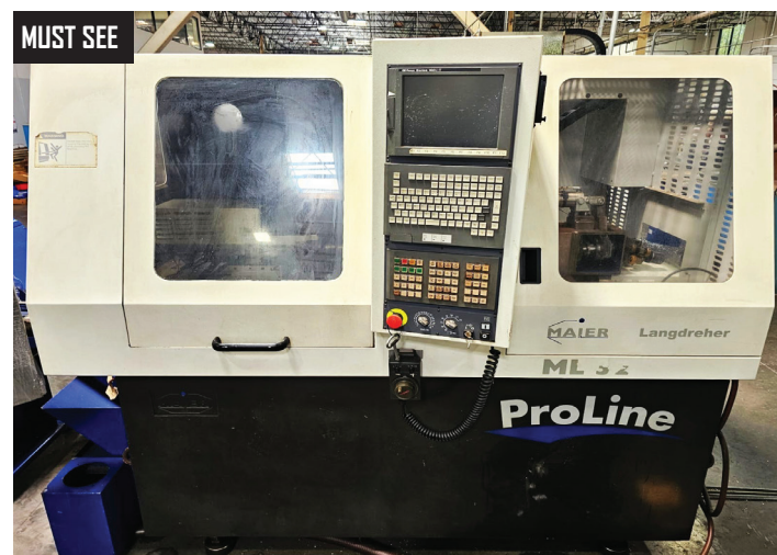
2002 Maier ML20 CNC Lathe, Twin Spindle Setup, Multi-Axis Configuration, Main Spindle; 0.787" Max Bar Capacity, 8000 RPM, Counter Spindle; 0.787" Max Bar Capacity, 8000 RPM, s/n 02 204, Fanuc 160i-T Controls, w/ Turbo Systems Chip Conveyor
