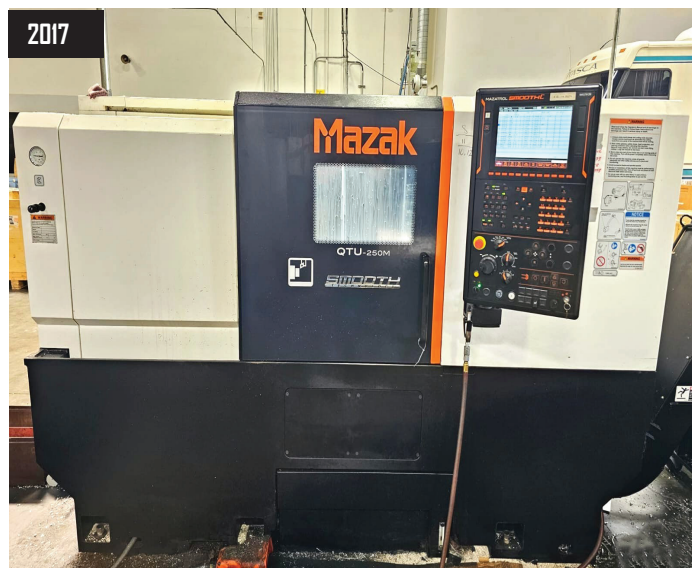
2017 Mazak Quick Turn Universal 250M CNC Lathe, 8" Chuck, 27.4" Max Swing, 13.6" Max Turning Length, 2.6" Bar Capacity, 20 HP, 4500 RPM Max Spindle Speed, 12 Position Live Tooling Turret, Tail Stock, s/n 279803, Mazatrol Smooth HC Control, Chip Conveyor, s/n A 170659-4
