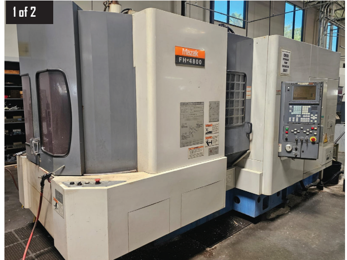
1 of 2 Mazak FH-4800 Horizontal Milling Machine, Travels 22"x24"x22" (XYZ), (2) 15.75" x 15.75" Pallets, 30HP, 12000RPM Max Spindle Speed, 40 ATC, CAT-40 Taper, s/n 142662, Mazatrol 640M Controls, w/ Chip Conveyor, s/n 99M5167
