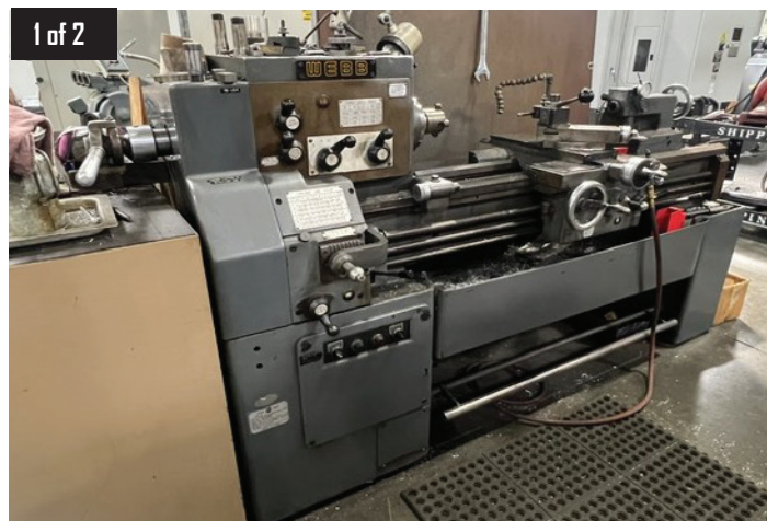
Webb 15X40 Engine Lathe, 10" 3-Jaw Chuck, Quick Change Tool Post, 5HP
