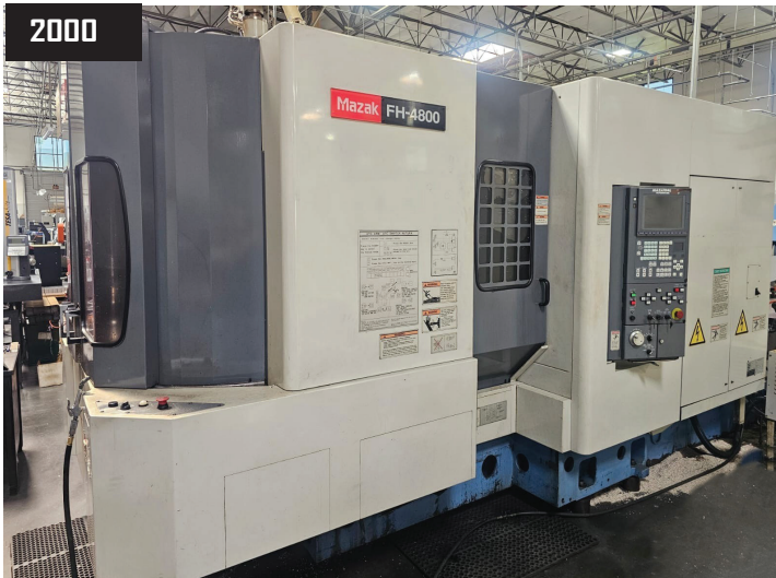
2000 Mazak FH-4800 Horizontal Milling Machine, Travels 22"x24"x22" (XYZ), (2) 15.75" x 15.75" Pallets, 30HP, 12000RPM Max Spindle Speed, 120 ATC, CAT-40 Taper, s/n 1509084, Mazatrol 640M Controls, w/ Barnes RDC-3-024H Chip Conveyor, s/n RD 1948 - 1 of 3
