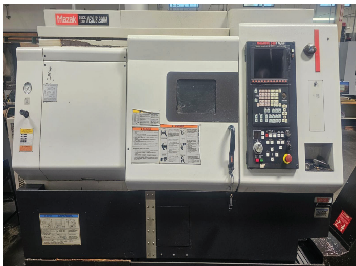
2003 Mazak Quick Turn Nexus 250M 3-Axis CNC Lathe, 10" Chuck, 26.5" Swing, Travels X-Axis 9" Z-Axis 22", 35HP, 4000RPM Max Spindle Speed, 12 Position Turret, Tail Stock, s/n 167034, Mazatrol 640T Nexus Controls, w/ Jorgensen Chip Conveyor s/n A031116-1
