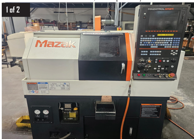
2017 Mazak Quick Turn Primos 100 S CNC Lathe, 5C Collet Spindle, 17.48" Max Swind, 7'87" Max Turning Length, Travels X-Axis 4.3" Z-Axis 9.4", 12HP, 5000 RPM Spindle Speed, 8 Position Turret, Tail Stock, s/n 282146, Mazatrol Smart Controls, w/ Bar Feed.
