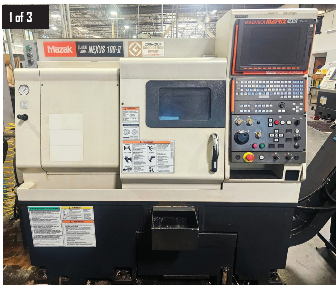
1 of 3) Mazak Quick Turn Nexus 100-II CNC Lathe, 6" Chuck, 21.6" Max Swing, 17.9" Max Turning Length, Travels Z-Axis 7.25" X-Axis 17.9", 15HP, 6000RPM Max Spindle Speed, 12 Position Turret, Tail Stock, Mazatrol Matrix Nexus Controls, w/ Chip Conveyor
