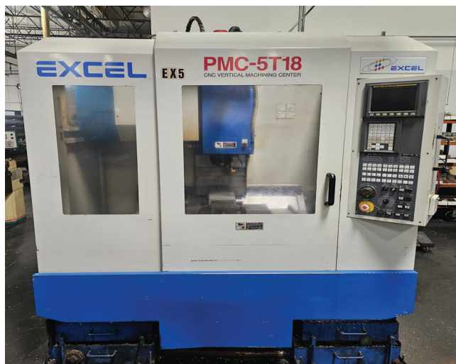
2000 Excel PMC-5T18 3-Axis CNC Vertical Milling Machine, Travels 20"x16"x18" (XYZ), 27.5" x 17" table, 7.5HP, 8000RPM Max Spindle Speed, 18 ATC, BT-40 Taper, s/n ES5T1610, Fanuc 21-M Controls
