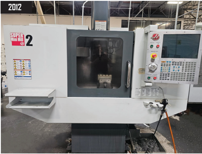
2012 Haas 3-Axis Vertical Milling Machine, Travels 20"x16"x14" (XYZ), 40" x 14" Table, 15HP, 10000RPM Max Spindle Speed, 10 ATC 40 Taper, s/n 1099209, Haas Controls
