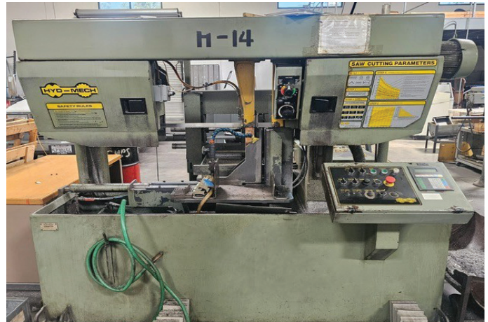
Hyd-Mech H-14 Horizontal Band Saw, 14"x14" Cutting Capacity, 5HP, 400 FPM Blade Speed, s/n 50599081
