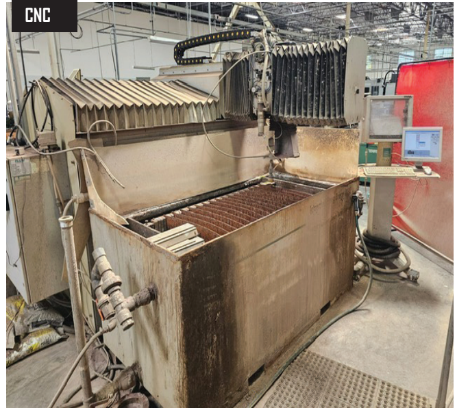
CNC 2004 Flow 713589-1 Compact 2' x 4' CNC Abrasive Waterjet Table, 48" X-Axis 24" Y-Axis, 55000 PSI, Flowmaster Flowcut Software, s/n 31589-1
