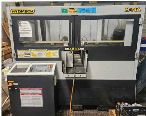
Hyd-Mech H-14A Fully Enclosed Automatic Horizontal Band Saw, 14”X14” Cutting Capacity, 13.6HP, 49-380 SFM Variable Speed, 15’2” x 1’25” Blade, Elevation TS 50 Controls, s/n 5-09-17-217-SB
