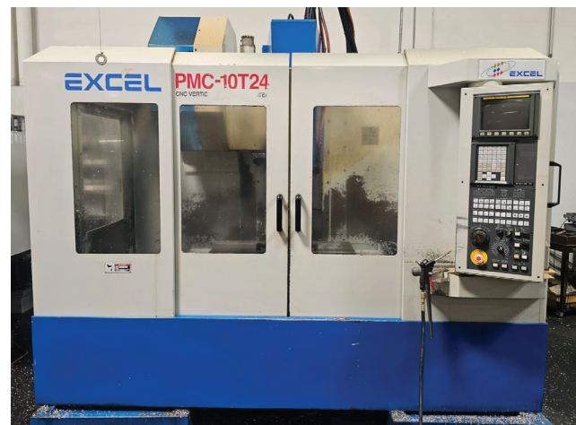
2000 Excel PMC-10T24 3-Axis CNC Vertical Milling Machine, Travels 40"x20"x24" (XYZ), 19"x40" Table, 14.7HP, 10000RPM Max Spindle Speed, 24 ATC, CAT-40 Taper, s/n ES10T2331, Fanuc 21-M Controls
