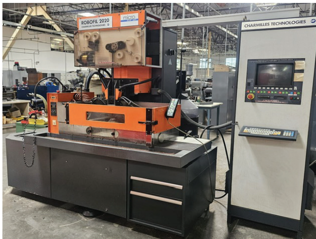
Charmilles Technologies Robofil 2020 CNC Wire EDM, 12"x8"x4.5" XYZ Travels, 39" X19"X10" Tank Size, 0.10 - 0.25 Wire Diameter Range, s/n 123008
