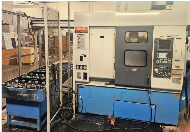
Mazak Quick Turn 250 HP CNC Lathe, 10' Chuck, 24" Max Swing, 13.78" - 14'96" Max Turning Diamenter, Travels X-Axis 8'5" Z-Axis 10" x 22", 35HP, 4000RPM Max Spindle Speed, 12 Position Turret, Tail Stock, s/n 148635, Mazatrol 640T Control, w/ Mazak Flex-GL50N Gantry Robotic Loader System s/n U9814, w/ Jorgensen Chip Conveyor s/n A-000991-1
