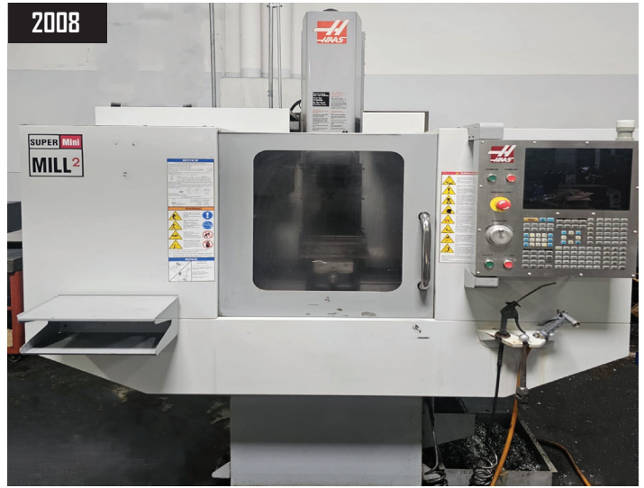
2008 Haas Super Mini Mill 2 4-Axis Compatible CNC Vertical Milling Machine, Travels 20"x16"x14" (XYZ), 40" x 14" Table, 15HP, 10000 RPM Max Spindle Speed, 10 ATC 40 Taper, w/ 4th Axis 5C Collet Indexer, s/n 1071623, Haas Controls
