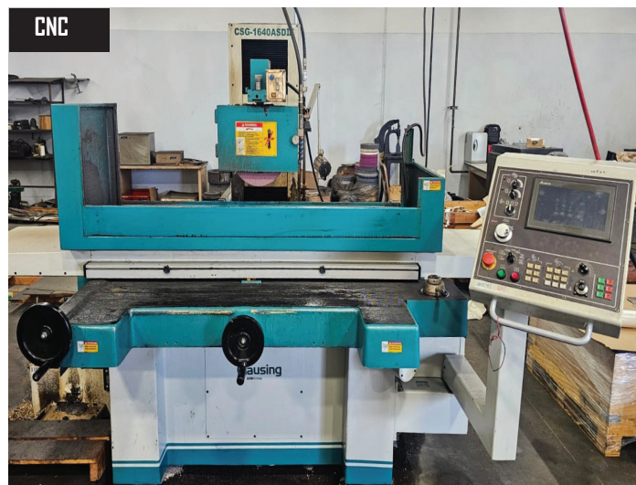
Clausing CGS-1640ASDII 3-Axis Automatic Surface Grinder, 16" x 40" Capacity, 7.5HP, 1750 RPM Spindle Speed, w/ 16" x 40" Magnetic Chuck
