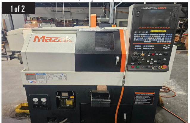
1 of 2) 2017 Mazak Quick Turn Primos 100 S CNC Lathe, 5C Collet Spindle, 17.48” Max Swind, 7’87 Max Turning Length, Travels X-Axis 4.3” Z-Axis 9.4”, 12HP, 5000 RPM Spindle Speed, 8 Position Turret, Tail Stock, s/n 282146, Mazatrol Smart Controls, w/ Bar Feed.
