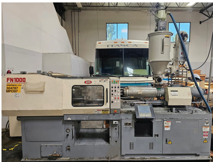
Neisei FN1000 Injection Molding Machine 90 Ton Injection Molding Machine, 3.2 Oz Shot, 21.4" x 21.4" Platen Size, 18.5" Clamp Stroke, s/n S08U126
