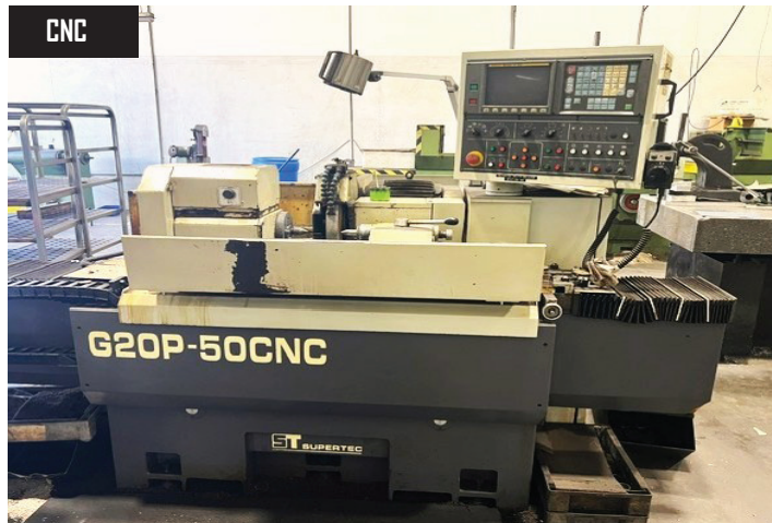
Supertec G20P-50CNC Universal Grinder, 8" Swing Over Table 20" Between Centers 8" Max Grinding Diameter, 5HP, 50-500 RPM Spindle Motor, MT3 Taper, s/n GCF10002
