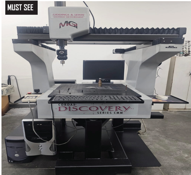
MUST SEE Giddings & Lewis Discovery D-8 Bridge Style CMM, Travels 20" x 24" x 16", Renishaw PH9 w/ TP6 Touch Trigger Probe, 22"x 26" Table, s/n P-0042-1297
