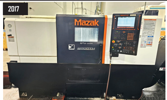
2017 Mazak Quick Turn Universal 250M CNC Lathe, 8” Chuck, 27.4” Max Swing, 13.6” Max Turning Length, 2.6” Bar Capacity, 20 HP, 4500 RPM Max Spindle Speed, 12 Position Live Tooling Turret, Tail Stock, s/n 279803, Mazatrol Smooth HC Control, Chip Conveyor, s/n A 170659-4
