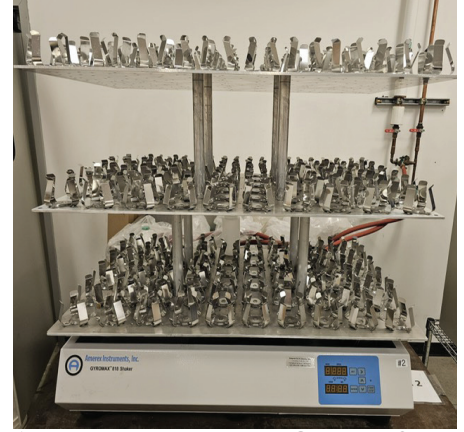
Amerex Instruments Inc. Gyromax SK-818 Open-Air Shaker, 24" x 38" Platform, 40-400 RPM, 25mm Orbital Motion, Microprocessor Controls, Digital Timer, s/n AI16113001-3.
