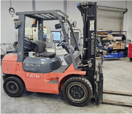
Toyota FG30 6000 lb. Capacity LPG Forklift, 3 Stage Mast, Side Shift, 48" Forks, Cushion Tires, s/n 67744.
