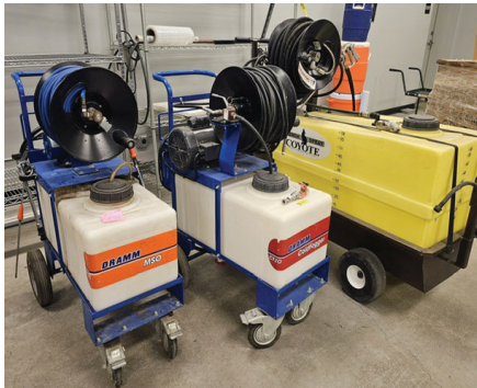
Dramm CF20 Coldfogger High Pressure Targeted Fogger, 20 Gallon Tank, 3000 PSI, s/n 180018.
