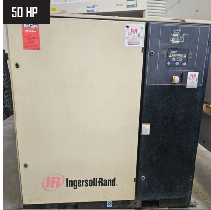
Ingersoll-Rand EP50-PE Rotary Screw Air Compressor, 205 CFM, 125 PSIG, 50HP, s/n PG1363U05034.
