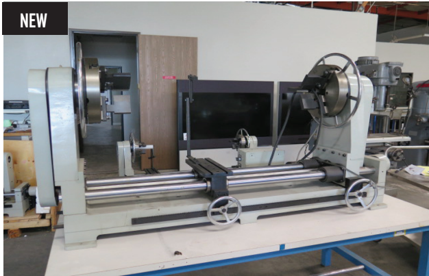
Import 100mm Glass Blowing Lathe w/ 100mm Thru Spindle Bores, 33" (Over Table) x 43", 0-187 RPM, Stepper Motor and Controller, 12" Chucks, 110 Volts
