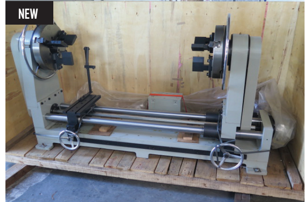
Import 100mm Glass Blowing Lathe w/ 100mm Thru Spindle Bores, 33" (Over Table) x 43", 0-187 RPM, Stepper Motor and Controller, 12" Chucks, 110 Volts
