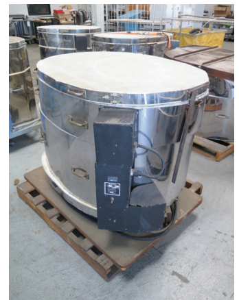
Aim Kilns PERS27 2000 Deg. F Electric Kiln w/ Digital Temp Control, 30" x 43" x 27" Cap
