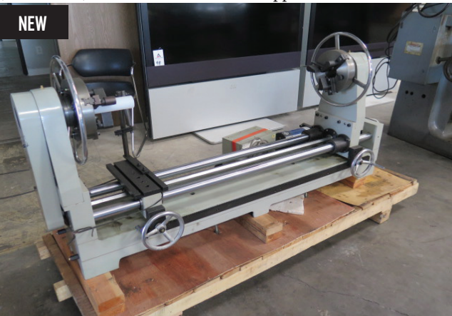
Import 65mm Glass Blowing Lathe w/ 65mm Thru Spindle Bores, 23" (Over Table) x 43 1/2", 0-187 RPM, Stepper Motor and Controller, 8" Chucks, 110 Volts
