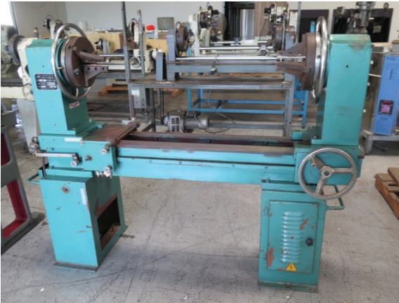
2011 Import CS125-390 125mm Glass Blowing Lathe w/ (NO MOTOR) 125mm Thru Spindle Bores, 28" (Over Table) x 43", 0-187 RPM, 10" Chucks
