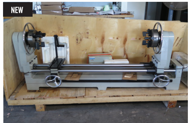
Import 65mm Glass Blowing Lathe w/ 65mm Thru Spindle Bores, 23" (Over Table) x 43 1/2", 0-187 RPM, Stepper Motor and Controller, 8" Chucks, 110 Volts 8105 inset w/ 8104
