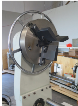
Import 100mm Glass Blowing Lathe w/ 100mm Thru Spindle Bores, 33" (Over Table) x 43", 0-187 RPM, Stepper Motor and Controller, 12" Chucks, 110 Volts
