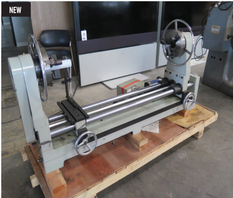
Import 65mm Glass Blowing Lathe w/ 65mm Thru Spindle Bores, 23" (Over Table) x 43 1/2", 0-187 RPM, Stepper Motor and Controller, 8" Chucks, 110 Volts
