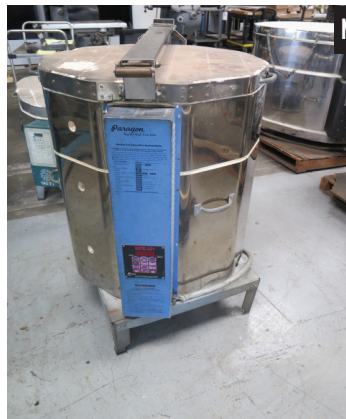
Paragon TNF24 2300 Deg. F Electric Kiln w/ Sentry 2.0 Digital Controls, 24" Dia x 29" Cap
