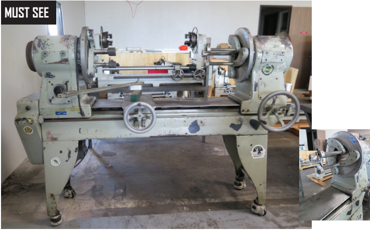
Bethlehem mdl. 8A 110mm Glass Blowing Lathe w/ 22" (Over Table) x 50.5", Motor and Controls, 11" Chucks
