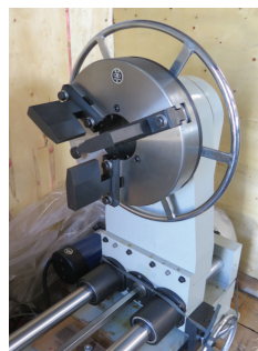
Import 65mm Glass Blowing Lathe w/ 65mm Thru Spindle Bores, 23" (Over Table) x 43 1/2", 0-187 RPM, Stepper Motor and Controller, 8" Chucks, 110 Volts
