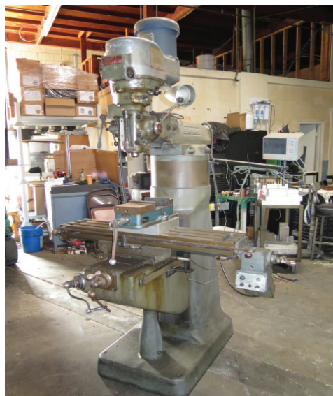
Bridgeport Vertical Mill w/ Mitutoyo DRO, Chrome Ways, Power Feed, 8" Riser
