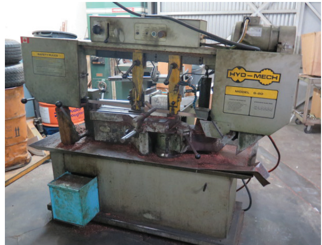
Hyd-Mech S-20 13" Horizontal Miter Band Saw w/ Hyd-Mech Controls, Work Stop
