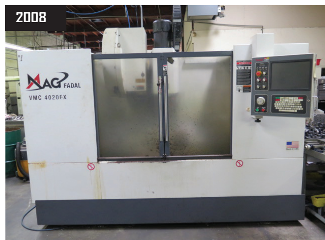
2008 Fadal VMC-4020 FXMP HT CNC VMC w/ Multi Processor CNC Controls, 24-Side Mount ATC, CAT-40, 10,000 RPM, Rigid Tapping, MM Ball Screws
