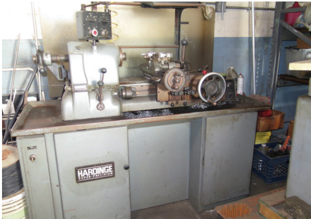
Hardinge HC Hand Chucker w/ 125-3000 RPM, 8-Station Turret, Power Feeds
