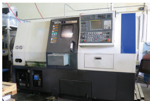
Hyundai WIA L210A CNC Turning Center w/ Fanuc I Series Controls, Tool Presetter, 12-Station Turret, Tailstock, Parts Catcher, 8" Power Chuck
