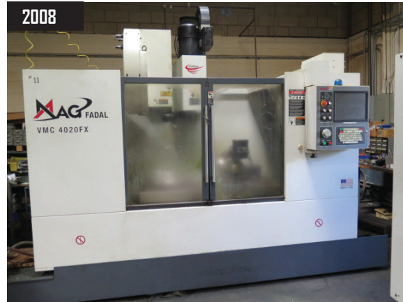
2008 Fadal VMC-4020 FXMP HT 5-Axis Capable CNC VMC w/ Fadal TR65 Multi-Axis Trunnion, Multi Processor CNC Controls, 24-Side Mount ATC, CAT-40, 10,000 RPM, 28" Extended "Z" Axis, Rigid Tapping, mm Ball Screws
