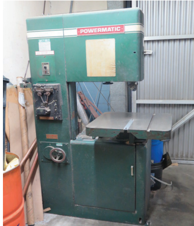
Powermatic mdl. 87 20" Vertical Band Saw w/ Blade Welder, Dial Change RPM
