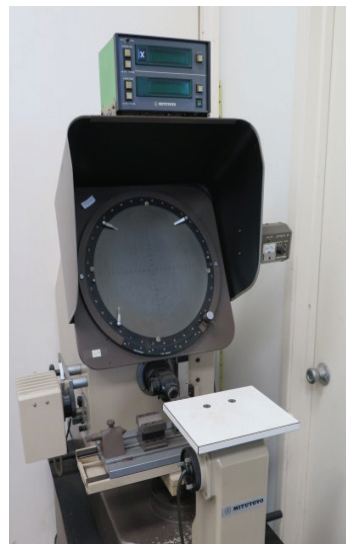
Mitutoyo PH350H 14" Optical Comparator w/ Mitutoyo DRO, Optoeye M1 Detection, Surface and Profile Illumination
