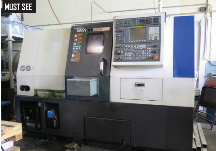
Hyundai WIA L210A CNC Turning Center w/ Fanuc I Series Controls, Tool Presetter, 12-Station Turret, Tailstock, Parts Catcher, 8" Power Chuck
