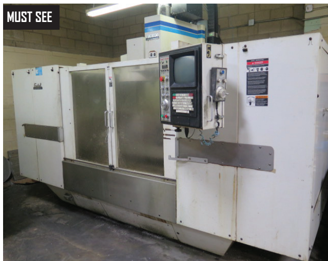
Fadal VMC6030 CNC VMC w/ CNC 88 HS Controls, Hand Wheel, 21-ATC, CAT-40 10,000 RPM, Rigid Tapping
