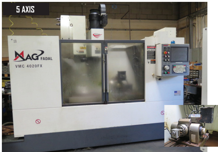
2008 Fadal VMC-4020 FXMP HT 5-Axis Capable CNC VMC w/ Fadal TR65 Multi-Axis Trunnion, Multi Processor CNC Controls, 24-Side Mount ATC, CAT-40, 10,000 RPM, 28" Extended "Z" Axis, Rigid Tapping, mm Ball Screws
