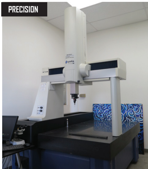
Mitutoyo 7106 Crysta-Plus M CMM Machine w/ Renishaw MH20 Probe Head, Mitutoyo MiCAT and Part Manager v3.0.R6 Software
