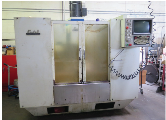
Fadal VMC40 4-Axis CNC VMC w/ CNC88 Controls, 21-ATC, CAT-40, 7500 RPM
