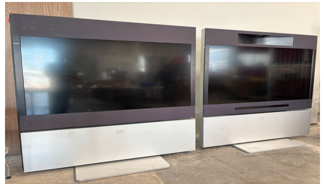
Cisco TelePresence MX800 Dual Screen Video Collaboration System w/ 70" High Definition Displays
