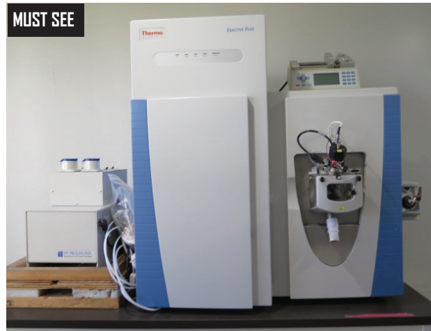
Thermo Scientific Exactive PLUS Mass Spectrometer
