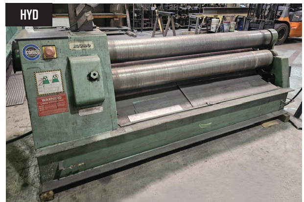
Roundo 72" x 3/8" Model PS-205 Hydraulic Double Pinch 3-Rolls Plate Bending Rolls.
