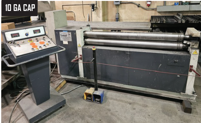
Famar 60" x 10Ga Model A312-15/3 Programmable Plate Bending Rolls.
