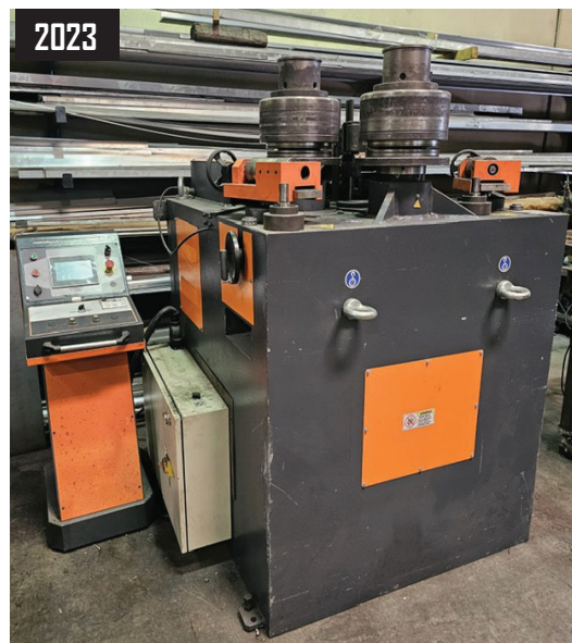
2023 KAAST PBH 100 NC Hydraulic Profile Roller, 3.9" Shaft Diameter, 12.5" Roll Diameter, 10HP, 275"/Minute Bending Speed, Weintek Controls & Foot Control, S/N 298536.
