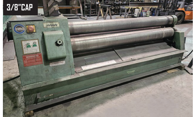
Roundo 72" x 3/8" Model PS-205 Hydraulic Double Pinch 3-Rolls Plate Bending Rolls.
