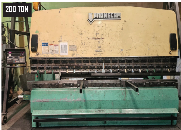
Promecam RG-204 14' 200 Ton Hydraulic Press Brake, 8.5" Stroke, 12' Between Columns W/ Hurco Autobend 6 CNC Backgauge Control System, S/N 33 20040 197
