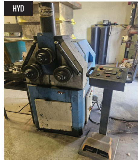
Baleigh R-H50-3-DR 3 Rolls Hydraulic Profile and Pipe Bending Rolls.
