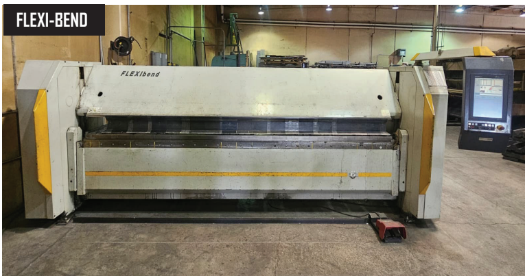
2005 RAS Flexibend 73.40 CNC Folding and Bending Machine, 160" x 13 GA. Capacity, 11.8" Upper Beam Max Strke, Folding Angle Brake 0-180°, 61" Backguage W/ System 6000 Touch & More Controls, S/N 39/10
