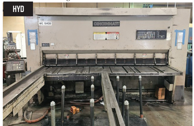
Cincinnati 500 Hydraulic Power Shear, 12 X 1/2" Capacity, 48" Backguage, 17-53 Strokes/Minute, 15 Hold Downs, 144" & 90" Front Arm Supports. S/N 47428
