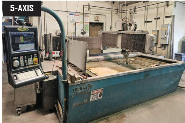
Techni TJ3000-X2 5 Axis CNC Waterjet Cutting System, 5'3" x 10'6" Table, 6" Thickness Cutting Capacity, Techni CNC Controls S/N TW146-US W/ KMT Streamline SL-V 50R Plus 50HP High Pressure Intensifier Waterjet Pump
