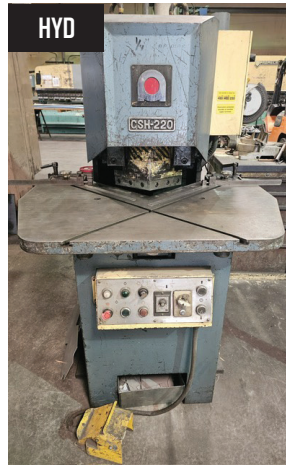
Amada CSH-220 Hydraulic Corner Notcher, .25" x 8" x 8" Capacity.
