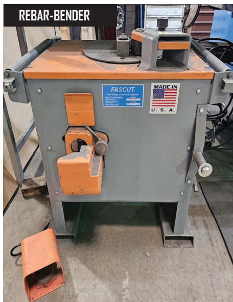
Fascut FR 800 C Rotary Rebar Bender / Cutter, Foot Controls S/N 19817
