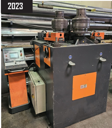
2023 KAAST PBH 100 NC Hydraulic Profile Roller, 3.9" Shaft Diameter, 12.5" Roll Diameter, 10HP, 275"/Minute Bending Speed, Weintek Controls & Foot Control, S/N 298536.
