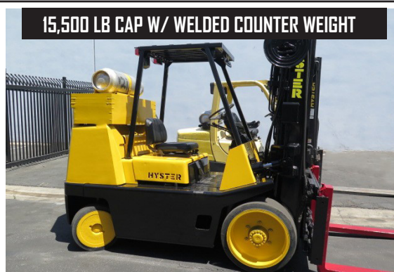
15,500 LB CAP W/ WELDED COUNTER WEIGHT Hyster S155XL2 15,500 Lb Cap LPG Forklift w/ 3-Stage Mast, 181” Lift Height, Side Shift, Welded Counterweight, 8’ Forks
