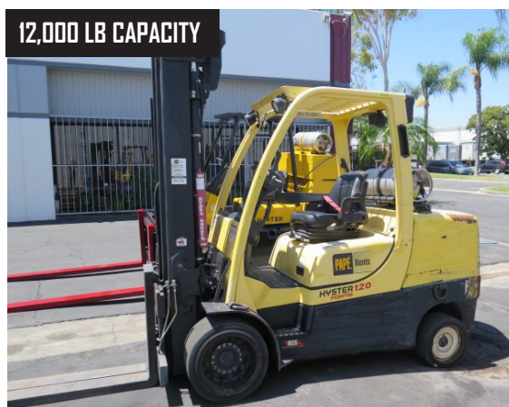
12,000 LB CAPACITY Hyster S120FT 12,000 Lb Cap LPG Forklift w/ Finger- Tip Controls, 3-Stage Mast, 208” Lift Height, Dura Match Trans, Hydra-Smooth Load Dampener
