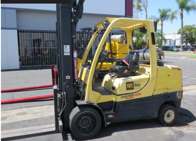
Hyster S120FT 12,000 Lb Cap LPG Forklift w/ Finger-Tip Controls, 3-Stage Mast, 208" Lift Height, Dura Match Trans, Hydra-Smooth Load Dampener
