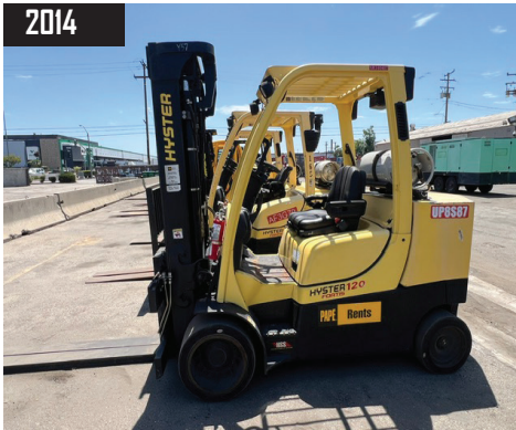
2014 Hyster S120FTS, 12,000 185/92, 3STG, LPG, 4X4, COWL, LEVER H004V02860M Cushion 3 Stage 185" LP, 9000 hrs, side shift.
