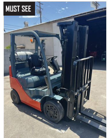
2009 Toyota 8FGCU25 5000 lb Cushion Tire Forklift Serial No: 24539 Meter Reads: 13707 Hours Comes With: 3 Stage Mast, 189 in Max Lift Height, 83 in Lowered Mast Height, 40 in Forks, Side Shift, 2009 US EPA Label, Toyota 4 Cylinder 2.2 L LPG Engine.
