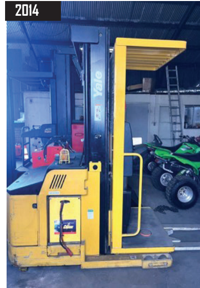
2014 Yale MODEL #: OS030EEN24TE093/ 3000 Lb Capacity Electric Order Picker, Three Stage MAST HEIGHT 95 / 213 in, SIDE SHIFTER, HOUR METER:3299.
