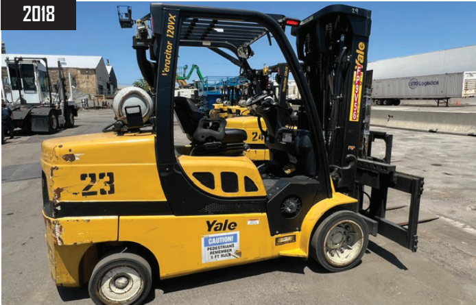
2018 Yale GLC120VX three-stage mast, s/s, 12000 capacity, cushion tires, mono, LPG, wide carriage
