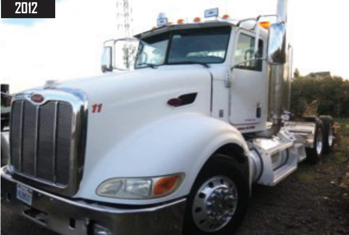
2012 Peterbilt Day Cab Semi Tractor w/ Diesel Engine, Eaton / Fuller 10 Speed Transmission, Cruise Control, 435,436 Miles, Vin # 1XPHDP9X1CD141624.
