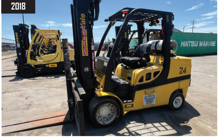
2018 Yale GLC120VX three-stage mast, s/s, 12000 capacity, cushion tires, mono, LPG.
