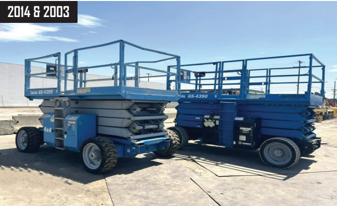
2014 and 2003 Genie GS-4390 4x4 Dual Fuel Scissor Lift, Serial number, 43 ft Max Platform Height, 1500 lb Max Weight Capacity, Platform Extension, Power to Platform, Upper Control Box, 2014 US EPA Label, 4 Cylinder 64.3 kW 2.5 L Dual Fuel Engine.
