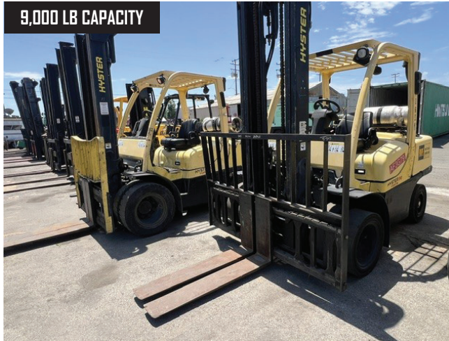
Hyster h90ft 9000 LBS Forklift, two-stage side shift, dual pneumatic tires, propane engine.
