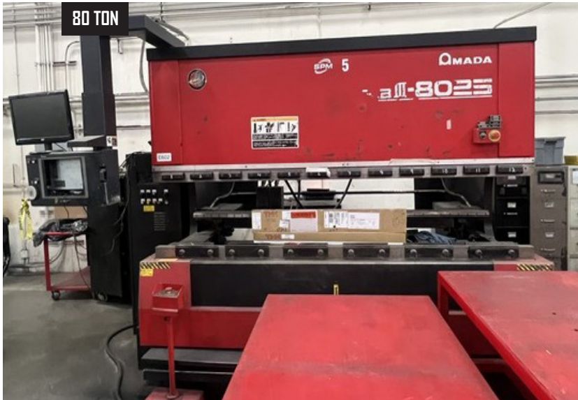
Amada 8025NT, 98.4" x 80 Ton CNC Hydraulic Press Brake, w/ Multi Axis CNC NT Controls.
