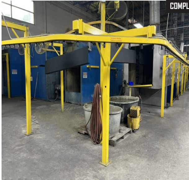
Complete Continuous Automated Powder Coating System 3 Stage Wash, Gas Fired Ovens, Powder Coating Guns and Conveyor System.
