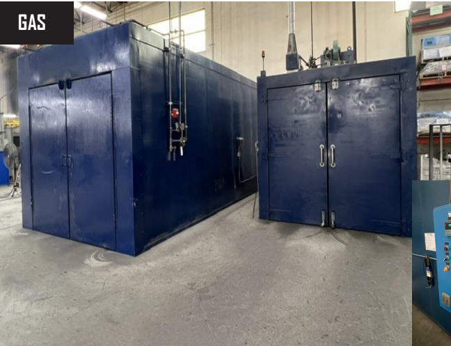
Gas-Fired Batch Walk-In Ovens for Powder Coating, 8' x 12' x 8' and 8' x 20' x 8' (WLH)
