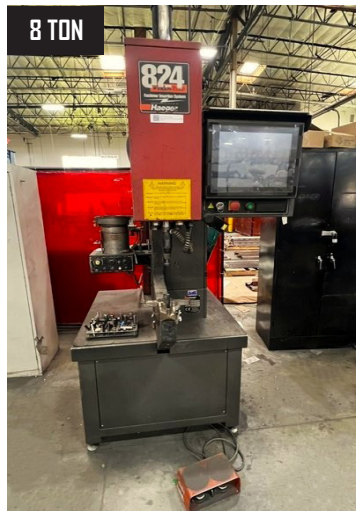
Haeger 824, 8 Ton x 24" Throat Hydraulic Insertion Press w/ Touch Screen Controls.
