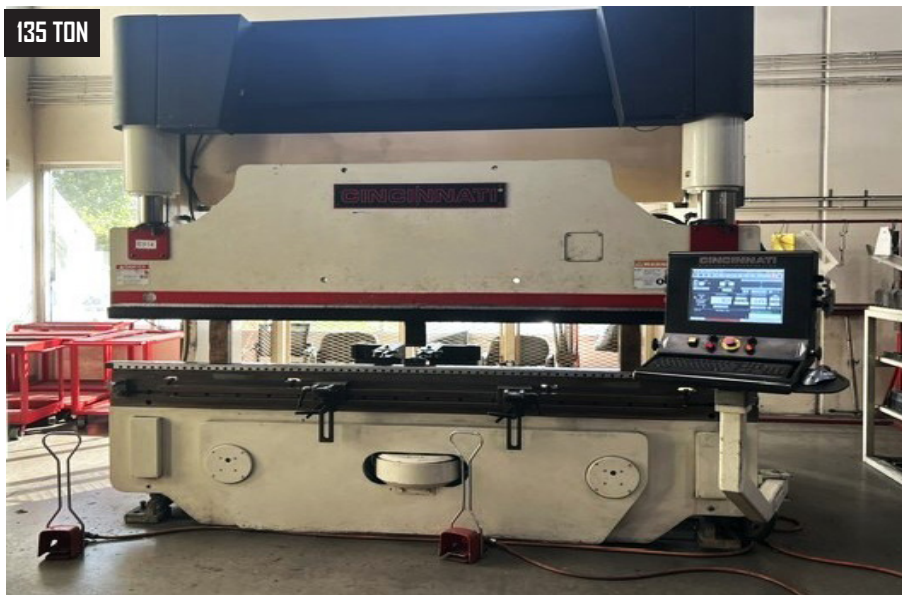
Cincinnati Maxform 135MX x 8 FT, 10' x 135 Ton CNC Press Brake, w/ Auto Crowning, PC Graphics, Multi Axis Controls, s/n 54789.
