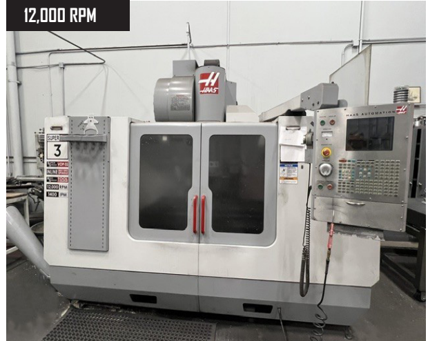
Haas VF-3 SS CNC VMC, 12,000 RPM, 24 ATC, CAT 40 Taper, 40" x 20" x 25" (XYZ Travels).
