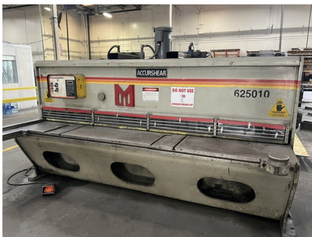
Accur Shear 625010, 10Ft x .25" Hydraulic Power Shear w/ Squaring Arm, FOPBG.
