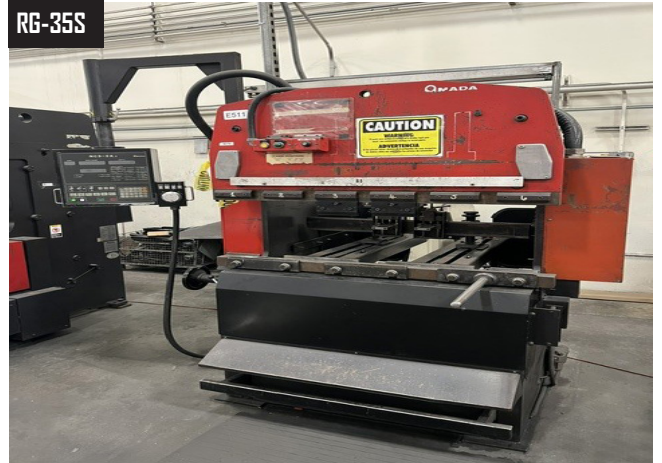
Amada RG-35S, 4Ft x 35 Ton CNC Hydraulic Press Brake, w/ 3 Axis NC9EXii Controls
