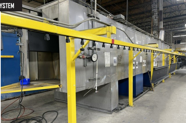
Complete Continuous Automated Powder Coating System 3 Stage Wash, Gas Fired Ovens, Powder Coating Guns and Conveyor System.
