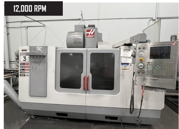
Haas VF-3 SS CNC VMC, 12,000 RPM, 24 ATC, CAT 40 Taper, 40” x 20” x 25” (XYZ Travels).
