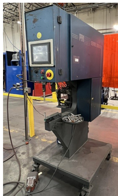
Pem Sert Series 2000 Hydraulic Insertion Press w/ CRT Controls.
