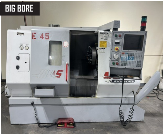
Haas SL20TB, CNC Lathe w/ Big Bore 2.5" Bar Capacity, 20" Max Turning Length, 3400 Spindle RPM.
