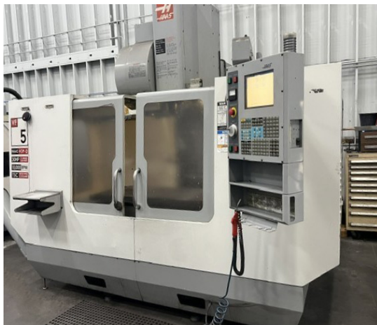
Haas VF-5 CNC VMC, 40 Taper, 50" x 26" x 25" (XYZ Travels), 10,000 RPM, 30 HP, 2 Speed Gear Driven, 24 ATC.
