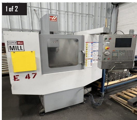
1 of 2) Haas Super Mini Mill, 40 Taper, 10,000 RPM, 10 ATC, 16" x 12" x 12" (XYZ Travels).
