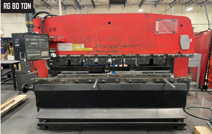
Amada RG-80, 94.6" x 80 Ton CNC Press Brake w/ 3 Axis NC9EXii Controls.
