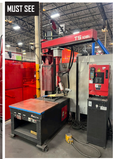
Amada TS108i, 80 KVA Inverter Spot Welder e/ 180 KVA Max Welding Power.
