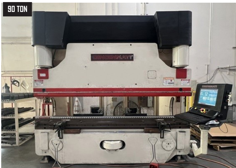
Cincinnati Maxform 90MX x 8 FT, 10' x 90 Ton CNC Press Brake, w/ Auto Crowning, PC Graphics, Multi Axis Controls, s/n 54788.
