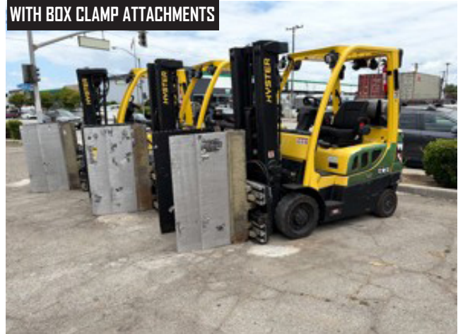
3 Hyster S50FT 5000 LPG Forklift with Hydraulic Box Clamp Attachments
