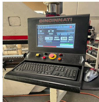
Cincinnati Maxform 135MX x 8 FT, 10' x 135 Ton CNC Press Brake, w/ Auto Crowning, PC Graphics, Multi Axis Controls, s/n 54789.
