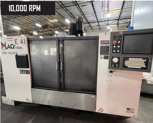
2008 Fadal-MAG VMC 4020FXMP-HT CNC VMC, 40 Taper, 40" x 20" x 20" (XYZ Travels), 10,000 RPM, 21 ATC.
