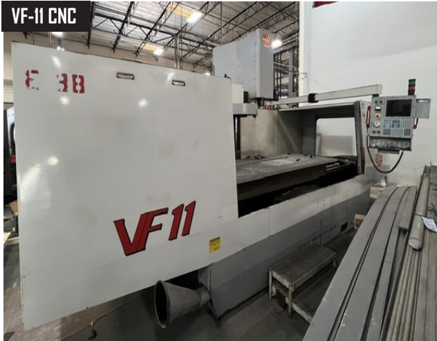
2000 Haas VF-11 CNC VMC, 3 Axis, 120" x 40" x 30" (XYZ Travels), CAT-40 Spindle, 20 ATC
