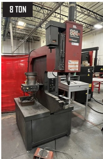
Haeger 824, 8 Ton x 24" Throat Hydraulic Insertion Press w/ CNC Controls.
