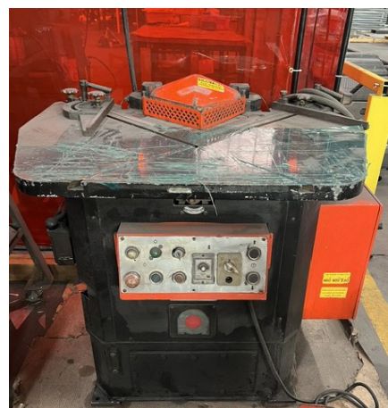
Amada CS-220, 10 Gauge Hydraulic Corner Notcher.
