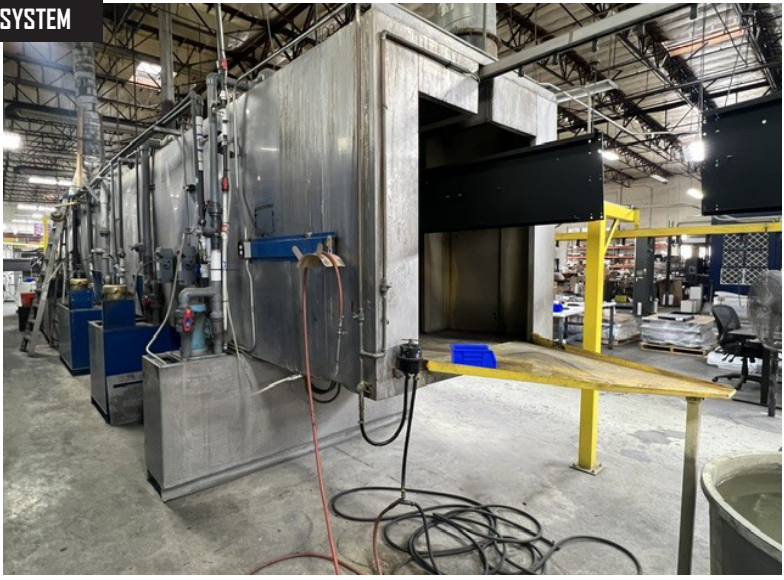
Complete Continuous Automated Powder Coating System 3 Stage Wash, Gas Fired Ovens, Powder Coating Guns and Conveyor System.
