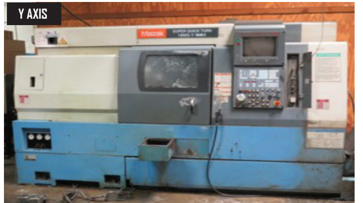
Mazak Super Quick Turn 18MS-Y MARK II Y-Axis Twin Spindle Live Turret CNC Turning Center w/ Mazatrol T-Plus Controls, Tool Presetter, Y-Axis, Sub Spindle, 12-Station Live Turret
