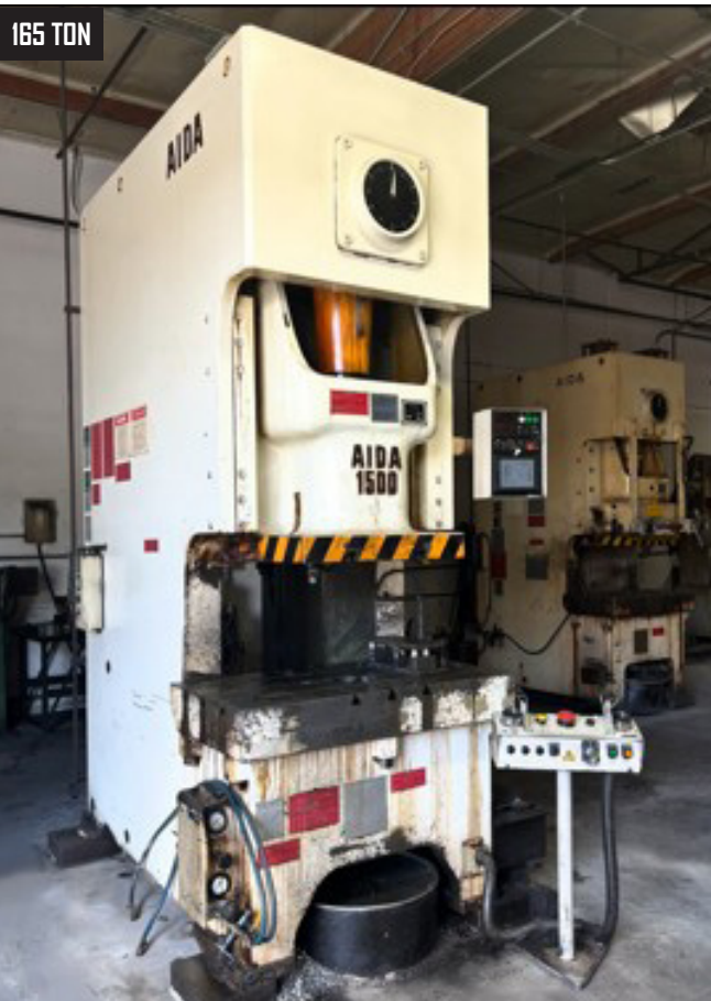
Aida 1500 mdl. NC1-1500(1)E 165 Ton Gap Frame Stamping Press w/ Aida Touch Screen Controls, 132 Ton Blanking Cap, 5.11” Stroke, 40-85 Strokes/Min
