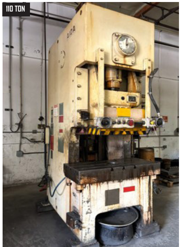
110 TON Aida mdl. NC1-11(1) 110 Ton Gap Frame Stamping Press w/ Aida Controls, 88 Ton Blanking Cap, 4.3" Stroke, 70 Strokes/Min, 12.5" Open Height
