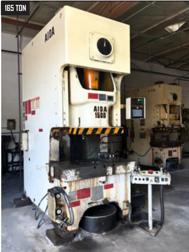
165 TON Aida 1500 mdl. NC1-1500(1)E 165 Ton Gap Frame Stamping Press w/ Aida Touch Screen Controls, 132 Ton Blanking Cap, 5.11" Stroke, 40-85 Strokes/Min
