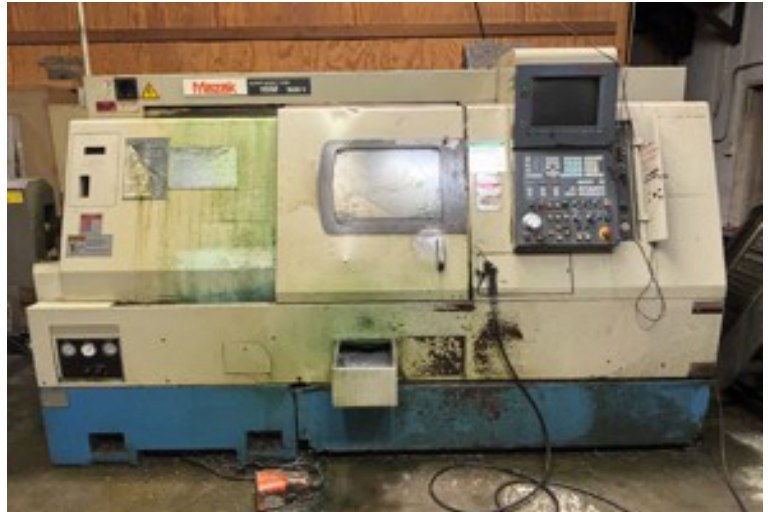
Mazak Super Quick Turn 15M MARK II Live Turret CNC Turning Center w/ Mazatrol T-Plus Controls, Tool Presetter, 12-Station Live Turret, Hydraulic Tailstock
