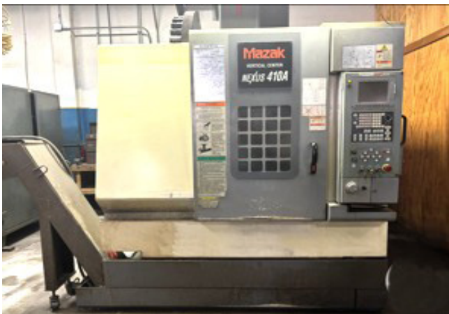
Mazak Nexus 410A CNC VMC w/ Mazatrol PC-Fusion-CNC 640M Nexus Controls, Tool Presetting Probe, 30-ATC, CAT-40 LNS Quick Load Bar Loader / Feeder
