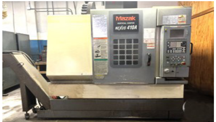
Mazak Nexus 410A CNC VMC w/ Mazatrol PC-Fusion-CNC 640M Nexus Controls, Tool Presetting Probe, 30-ATC, CAT-40
