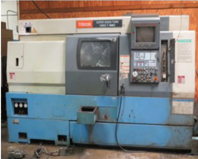
Mazak Super Quick Turn 18MS-Y MARK II Y-Axis Twin Spindle Live Turret CNC Turning Center w/ Mazatrol T-Plus Controls, Tool Presetter, Y-Axis, Sub Spindle, 12-Station Live Turret
