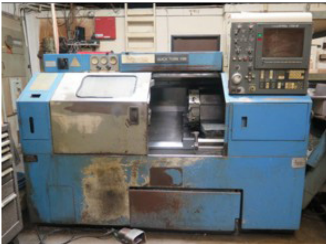
Mazak Quick Turn 15N CNC Turning Center w/ Mazatrol T-Plus Controls, Tool Presetter, 12-Station Turret, Hydraulic Tailstock
