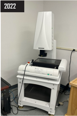
2022 Micro-Vu Vertex 261 Multisensor Vision Measuring Machine (VMM), 250 mm x 160 mm x 160 mm (XYZ), w/ Inspec Software, s/n M2840U0001.
