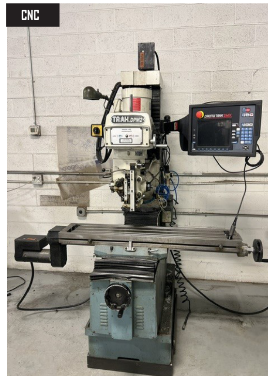
Southwestern Industries Trak DPMSX2 CNC Bed Mill w/ Proto Trak SMX Controls, 49" x 9" Table, 31" x 16" x 22" (XYZ).
