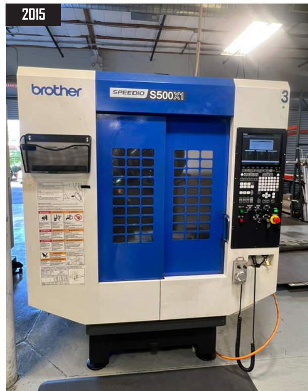
1/2015 Brother Speedio S500X1 CNC High-Speed VMC, BT-30 Taper, 14 ATC, 19.7" x 15.7" x 11.9" (XYZ), 10,000 RPM, s/n 128343.
