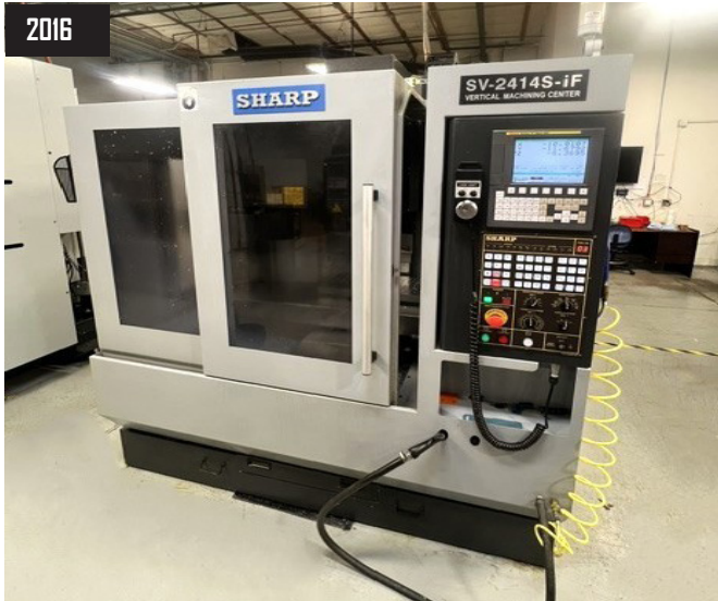
2016 Sharp SV-2414S-iF CNC VMC, w/ Fanuc Oi Control, 10,000 RPM, 24" x 14" x 18" (XYZ), Cat 40, 16 ATC, s/n 6072.
