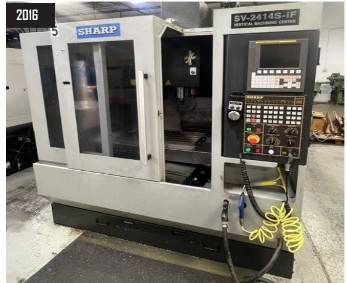
2016 Sharp SV-2414S-iF CNC VMC, w/ Fanuc Oi Control, 10,000 RPM, 24" x 14" x 18" (XYZ), Cat 40, 16 ATC, s/n 6071.
