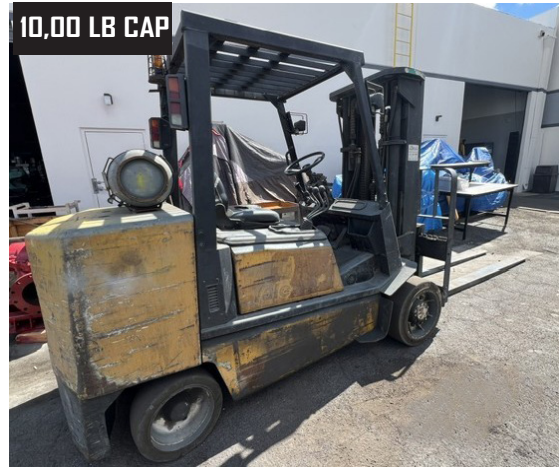
Yale GLV100MG 10,000 Lb Cap LPG Forklift w/ 3-Stage Mast, 178" Lift Height, Side Shift, 4 th Actuator Lever, 8' Forks, Cushion Tires.
