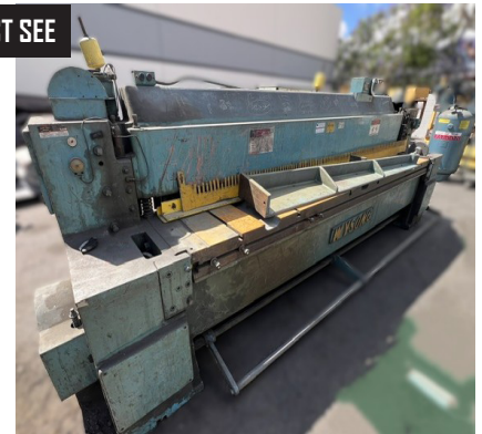
Wysong 1010-HD 10Ga x 10' Cap Power Shear s/n P8-453 w/ Dial Back Gauge, Squaring Arm, Front Support
