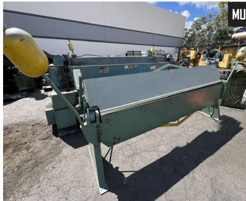
2019 Bolton Tools W2.0X3050A9120") 10' Box and Pan Finger Brake s/n A19111621.
