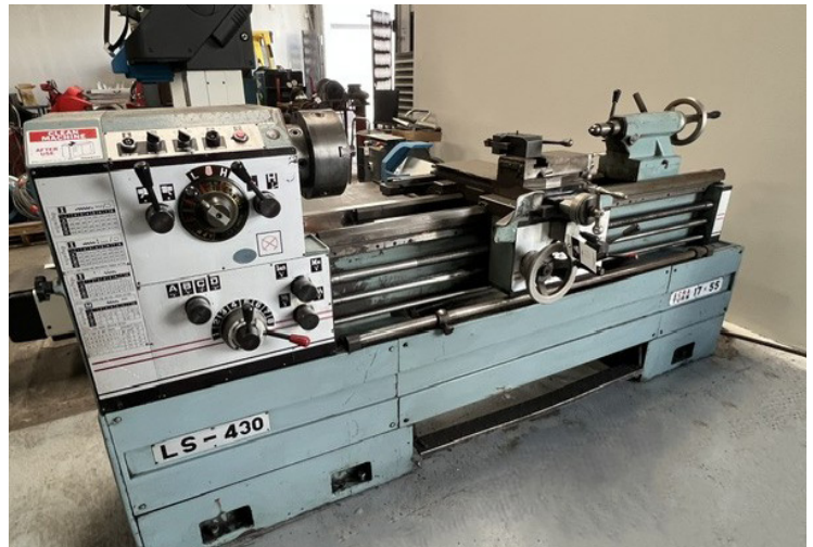
Acra Turn LS-430 17" x 55" Geared Head - Gap Bed Lathe w/ 31-1520 RPM, Taper Attachment, Inch/mm Threading, Tailstock, Tool Post, 10" 3-Jaw Chuck, Coolant.
