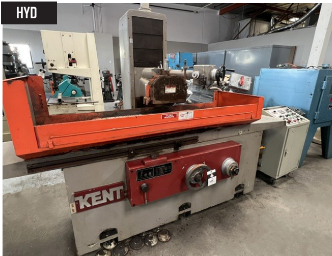
Kent KGS-410AHD 15 3/4" x 39" Automatic Hydraulic Surface Grinder s/n 890572-2 w/ Kent Controls, Wheel Dresser, Electromagnetic Chuck, Coolant.
