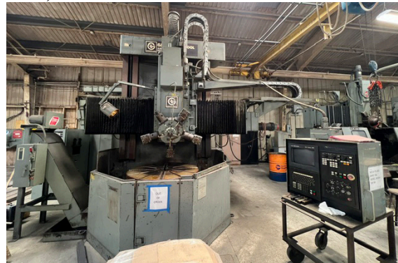
Giddings & Lewis CNC Vertical Turret Lathe, w/ Mark Century 2000 Controls, 4 Jaw Chuck, s/n 512-263-87.
