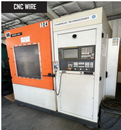
Charmilles Robofill 330F CNC Wire EDM, w/ Fanuc Controls, 15.75" x 11.81" x 75" Travels.
