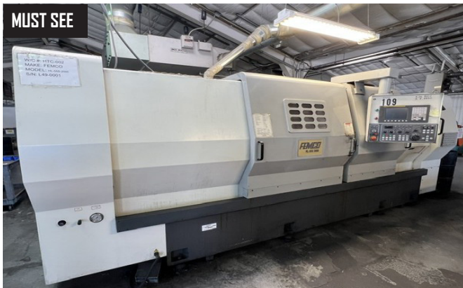
2009 Femco HL-55S-2000 CNC Lathe, 28.6” Swing Over Bed, 78.7” Between Centers, Tail Stock, 4.5” Bar Capacity, 12 Station Turret, Fanuc Oi-TD Controls. Control, 43.3” Chuck, 55.1” Swing.
