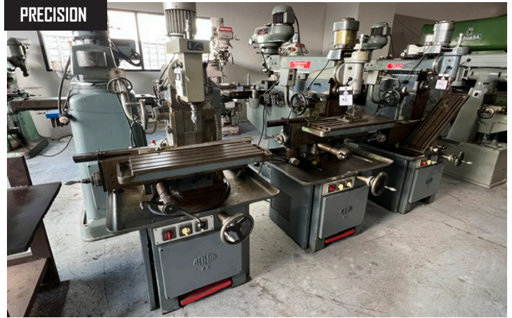
(3) Aciera F3 Horizontal Mill w/ Vertical Milling Attachment, 120-2400 RPM, 8x 24 Pivoting Table, Power Feed Unit, Coolant.
