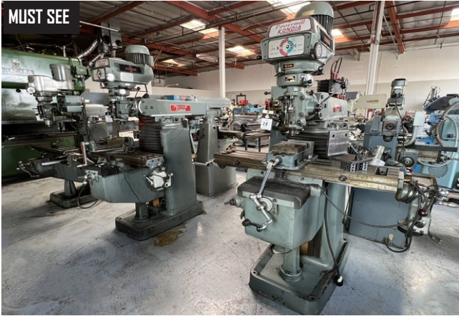
3) Kondia "Powermill" FV-1 Vertical Mill s/n M636 w/ 60-4000 Dial RPM, Power Feed, 9" x 42" Table.
