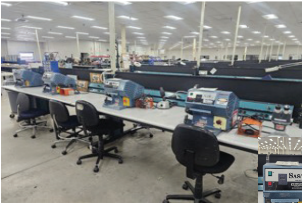
SAS/2 Model SAS 2-20 Autosplice Semi Automatic Solderless Crimp Connection Machines for Wire and Components.
