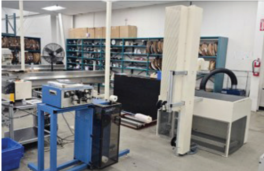
Komax 34 Precision Wire Cutting and Stripping Machine with Coiling Assembly.
