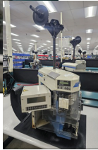
Amp-O-Lectric Model G Terminal Crimping Machine with Model 1320420 2-G w/Crimp Quality Monitor.
