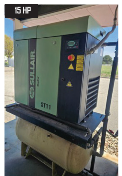
Sullair ST 1109AC, 15 HP Rotary Air Compressor and Sullair SRB15 Air Dryer.
