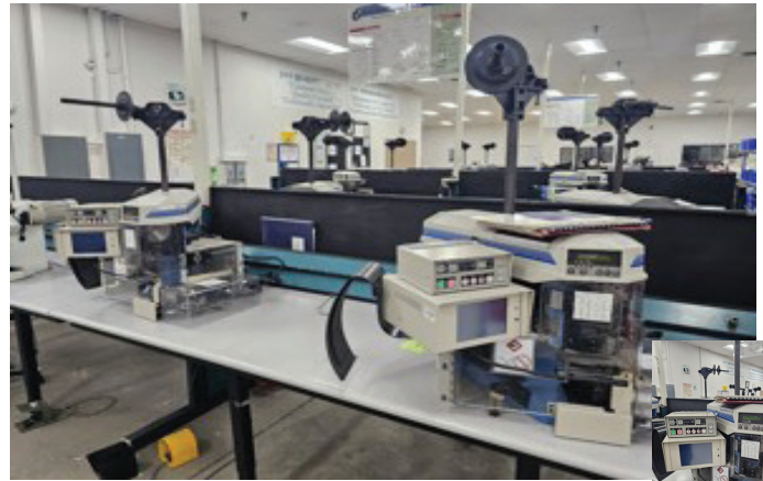
Amp-O-Lectric Model G Terminal Crimping Machine with Model 1320420 2-G w/Crimp Quality Monitor.
