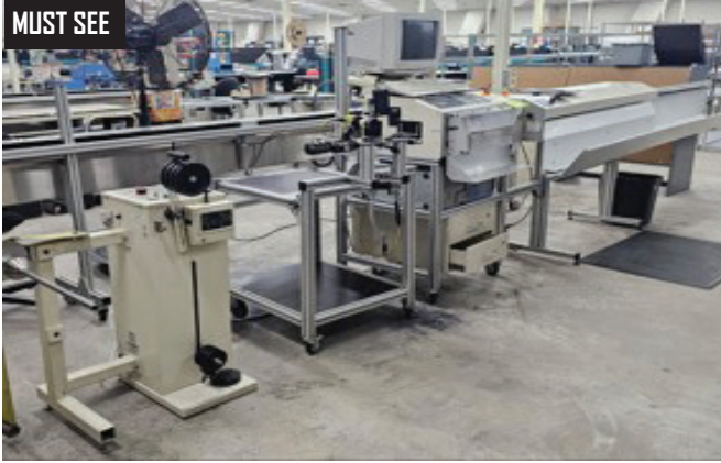
MUST SEE Schleuniger Model OC 3950 Automatic Wire and Cable Cutting Machine for up to 15 mm O.D. Equipped with Coil Line assemble, 50-1200 mm/sec Cutting Speed.
