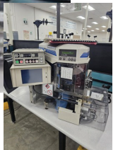
Amp-O-Lectric Model G Terminal Crimping Machine with Model 1320420 2-G w/Crimp Quality Monitor.
