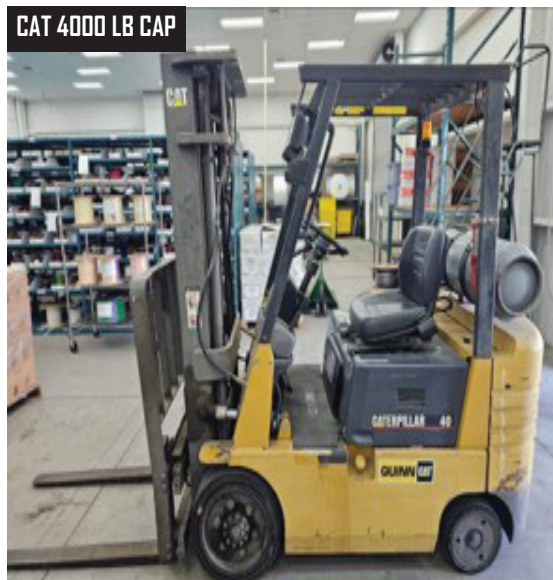
CAT 4000 LB Capacity LPG Forklift, Model GC-20.
