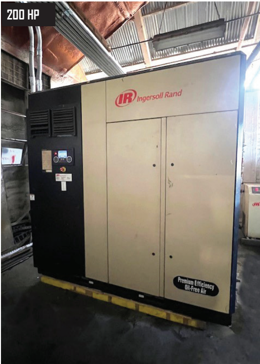
Ingersoll Rand IRN200H-OF 200 HP Rotary Air Compressor w/ Max 155 PSIG Discharge Pressure.
