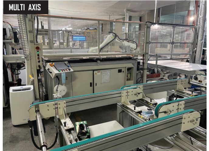
2016 Komax Xcell 3000 Stringer Solar Cell Production Machine w/ Kawasaki Multi Axis Robotics and Lay Up Station w/ Allen Bradley Controls.
