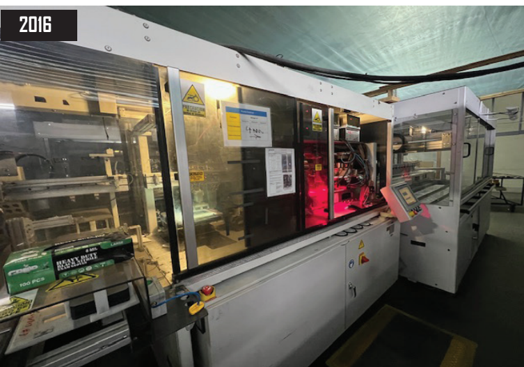
2016 Komax Xcell 3000 Stringer High Efficiency Solar Cell Production Machine w/ Allen Bradley Panel View Controls.
