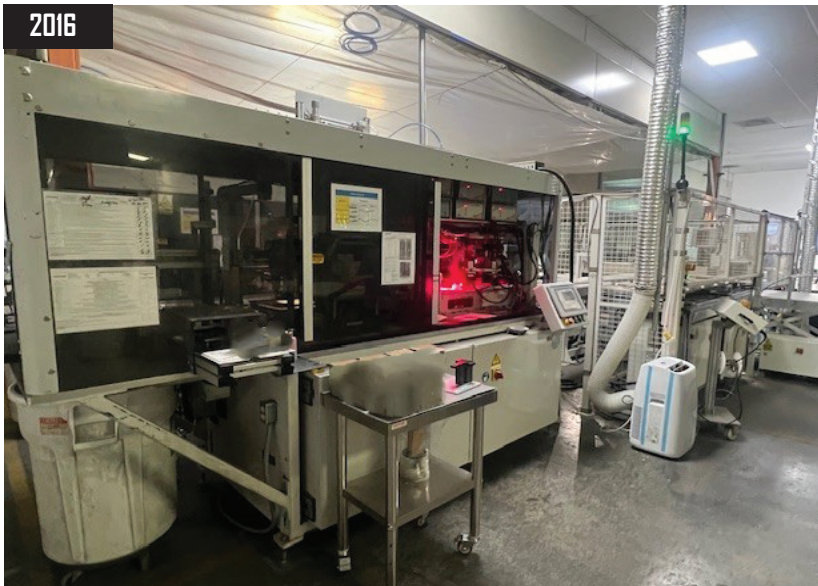
2016 Komax Xcell 3000 Stringer Solar Cell Production Machine w/ Kawasaki Multi Axis Robotics and Lay Up Station w/ Allen Bradley Controls.
