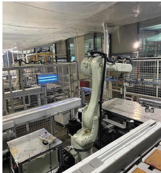
2016 Komax Xcell 3000 Stringer Solar Cell Production Machine w/ Kawasaki Multi Axis Robotics and Lay Up Station w/ Allen Bradley Controls.
