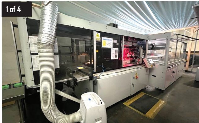
2016 Komax Xcell 3000 Stringer High Efficiency Solar Cell Production Machine w/ Allen Bradley Panel View Controls.
