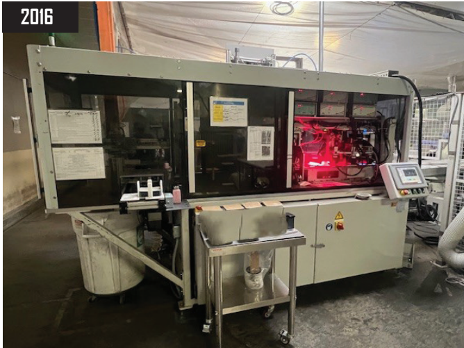
2016 Komax Xcell 3000 Stringer Solar Cell Production Machine w/ Kawasaki Multi Axis Robotics and Lay Up Station w/ Allen Bradley Controls.
