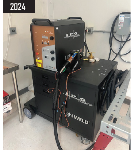
2024 IPG Light Weld 1500XR Model LHW-1500-XR-10 Fiber Laser Welding System w/ Laser Welding Wire Feeder.
