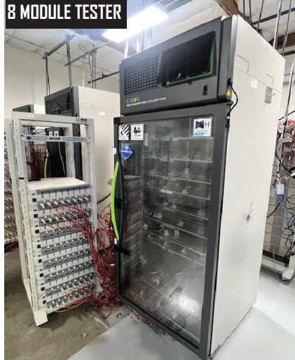
Neware 8 Module Battery Test System model 425W CT-4008T-5V6A-S1 and Caron 6041 Refrigerated Incubator.
