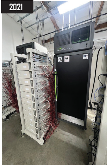
2021 Neware 14 Module Battery Test System model 425W CT4008T-5V6A-S1 and Caron 6041 Refrigerated Incubator.
