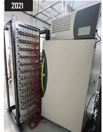
2021 Neware 13 Module Battery Test System model 425W CT4008T-5V6A-S1 and Caron Refrigerated Incubator.
