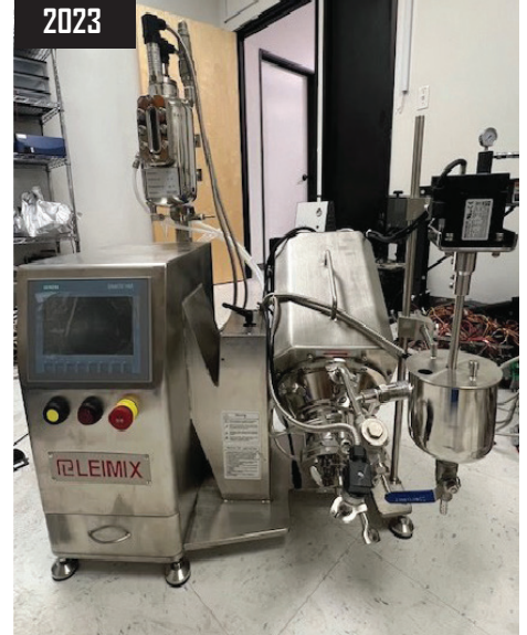
2023 Puhler/Leimix Labstar 0.3CE Universal Laboratory Agitator Bead mill.
