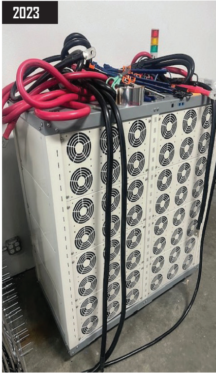
2023 Neware CT-40025V1000A-NTA, 17KW Battery Test System.
