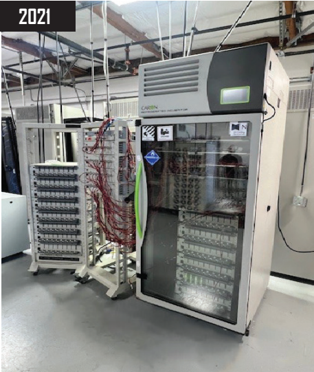
2021 Neware 13 Module Battery Test System model 425W CT-4008T-5V6A-S1 and Caron Refrigerated Incubator.
