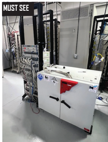
Binder Drying and Heating Oven w/ Gravity Convection and Neware 7 Module Battery Test System.
