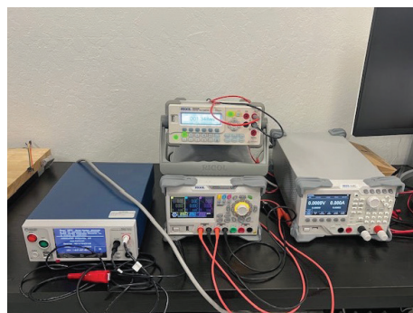
Rigol DL3021 DC Electronic Load, DM3058E Digital Multimeter, and DP932U Programmable DC Power Supply.
