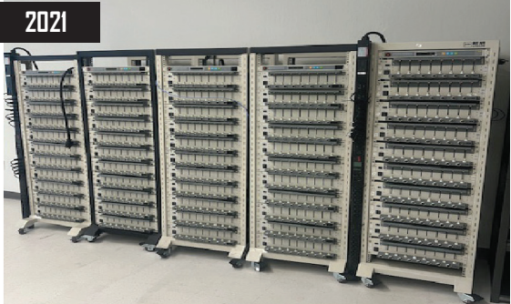
2021 Neware 10 and 11 Module Battery Test System model 425W CT-4008T-5V6A-S1
