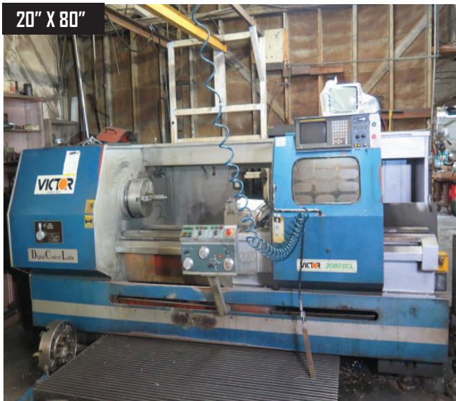
Victor 2080 DCL 20" x 80" CNC Lathe w/ Fanuc 20T Controls, Tailstock, Steady Rest, 12" 3-Jaw Chuck
