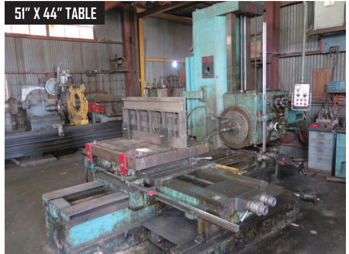
Cervit AC100 Horizontal Boring Mill w/ Acu-Rite Master Mill 3-Axis DRO, 12-1200 PM, 4" Spindle, 51" x 44" Table
