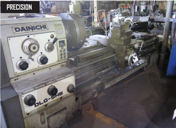
Dianichi DLG-SBH Geared Head Lathe w/ 18-1600 RPM, 3 1/2" Thru Bore, Taper Attach, Inch/mm Threading, Tailstock, 19 1/2" Chuck
