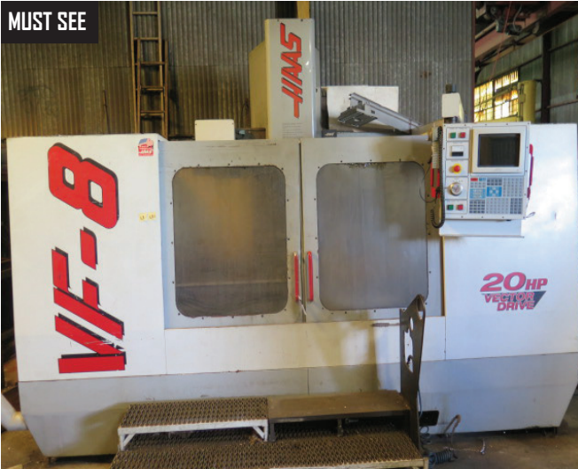
Haas VF-8 CNC VMC w/ 20-Station ATC, CAT-40, 10,000 RPM, Rigid Tapping, Programmable Coolant
