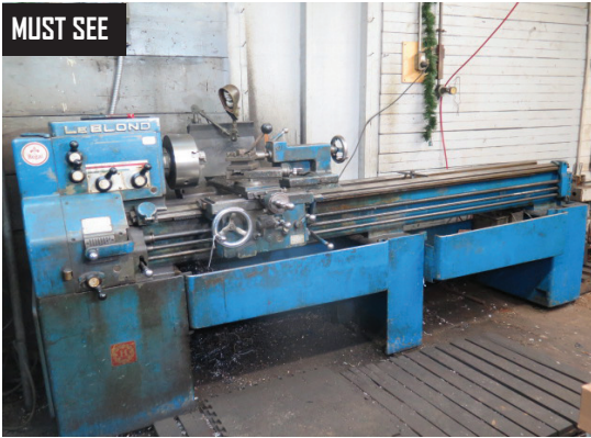
LeBlond Regal 15 1/2" x 80" Geared Head Lathe w/ 45-1800 RPM, Inch Threading, Tailstock, 10" 3-Jaw Chuck
