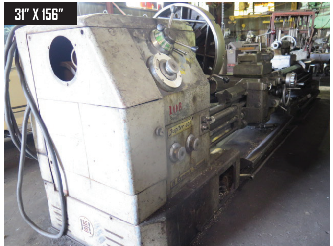
HES Jupiter 830 31" x 156" Gap Bed Lathe w/ 25-1600 RPM, 40" Swing @ Opening, Inch/mm Threading, Tailstock, 28" Chuck
