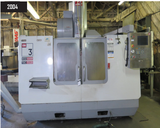
2004 Haas VM-2 Mold Makers 5-Axis Capable CNC VMC w/ 24-Station ATC, CAT-40, 12,000 RPM, Rigid Tapping, Thru Spindle Coolant
