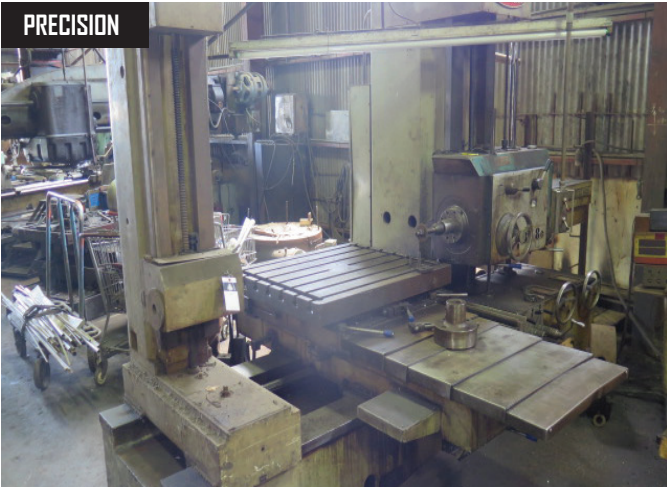
Shibaura BT-8c Horizontal Boring Mill w/ Pathfinder DRO, 20-1000 RPM, 3 1/4" Spindle, 35 1/2" x 41 1/2" Table
