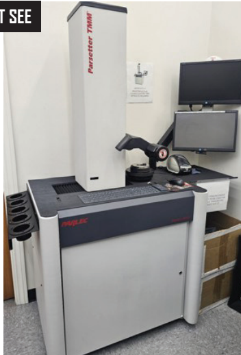
Parlec Parsetter TMM Series 1850, Tool Presetter; Up to 420mm Diameters, w/ Controls.
