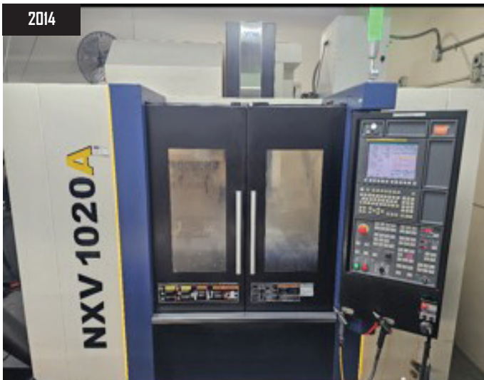
2014 YCM NXV1020A CNC VMC, 12,000 RPM, Fanuc MXP-200FA Control, Cat 40 Taper, 40.16" x 20.47" x 21.26" (XYZ), 24 ATC, s/n 0371
