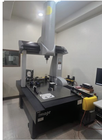
2002 Brown & Sharpe Global Image 7107 CMM, 27.6" x 39.4" x 23.6" Measuring Range, PH10MQ Probe Head, s/n 0602-1415.
