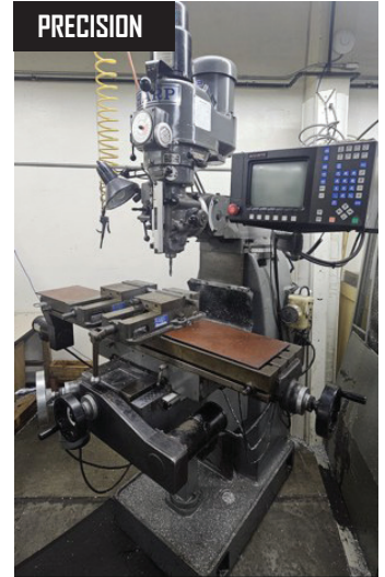
Sharp Vertical Milling Machine with Acu Rite CNC Controls, Chrome Ways, Variable Speed.
