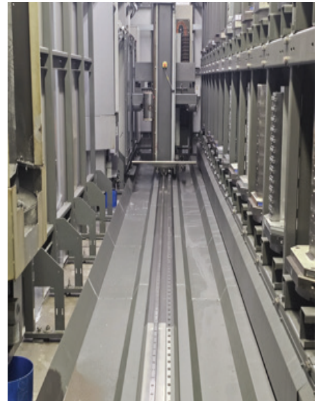
2) Toyoda FH 450 S Horizontal Machining Centers w/ Cell System, 17.7" x 17.7" Pallets, 23.62" x 23.62" x 23.62" (XYZ), w/ Fanuc 31i Model A Controls, 30 Pallets, 15K RPM, Cat 40 Tool, 494 ATC .
