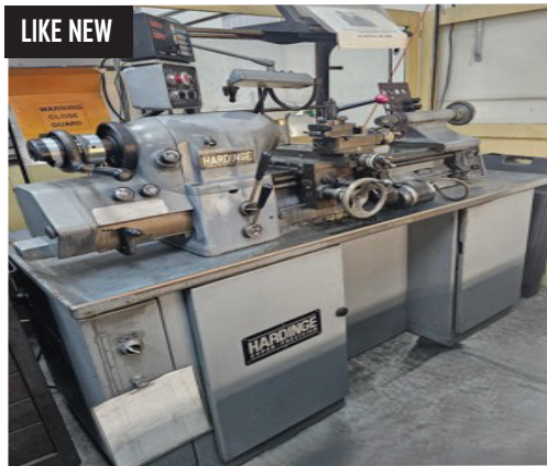
Hardinge HLV-H-EM Super Precision Tool Room Lathe, 11" x 18" Travels, Inch and Metric Threading, 3000 RPM, 1.25" Spindle Bore, DRO
