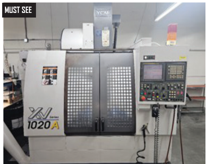
YVM XV-1020A CNC VMC, 40.16" X 20.47" X 21.26" (XYZ), 24ATC, W/ FANUC MXP-2001 CONTROLS, S/N 05010869
