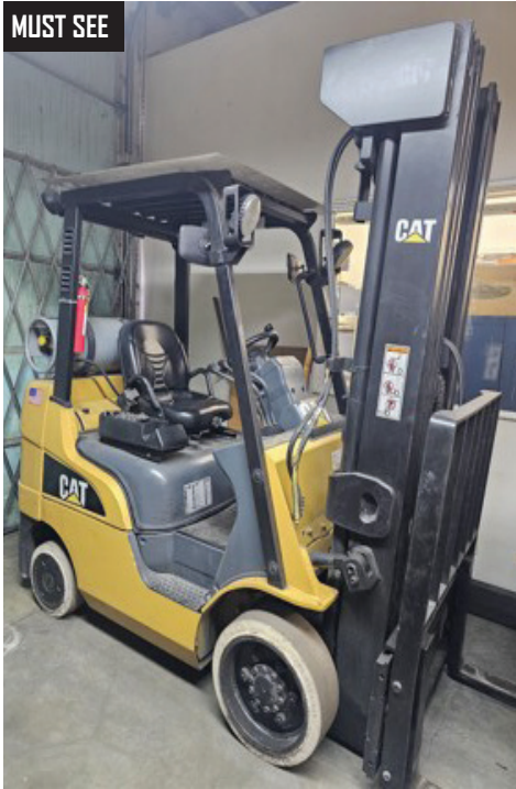
Caterpillar C5000, 5000 lb Capacity Forklift, LPG, 3 Stage Mast, Side Shift, s/n AT9020945
