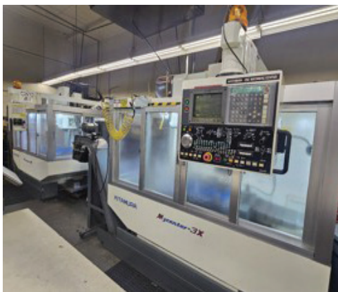
2) Kitamura Mycenter 3X CNC VMC's, 10,000 RPM, 30" x 18" x 18" (XYZ), 40 Taper, Yasnac Controls, Side Mount Tool Changer.
