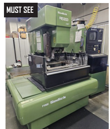
Sodick A530D CNC Wire EDM, 4 Axis, 19.6" x 12" x 10.6" (XYZ), AWT Automatic Wire Threading, Submerged System, w/ Sodick EX21 Controls.
