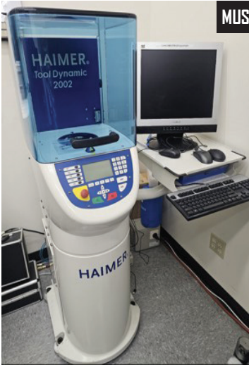
Haimer Tool Dynamics 2002 Vertical Balancing Machine, 14.96" Max Tool Diameter, 15.7" Max Navigation.
