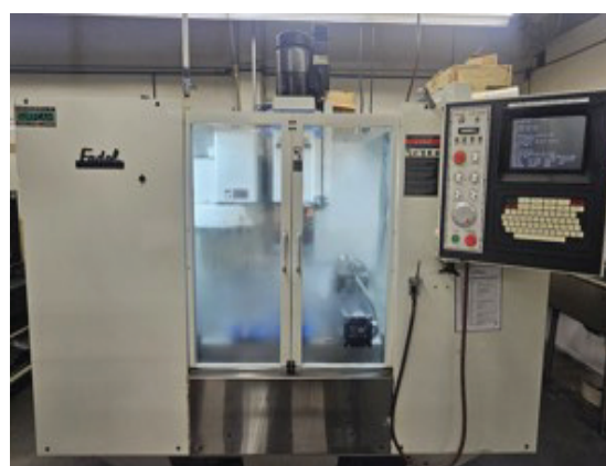
1994 Fadal VMC 3016 Machining Center, 40 Taper, 21 ATC, 30" x 16" x 20" (XYZ), s/n 9402724.
