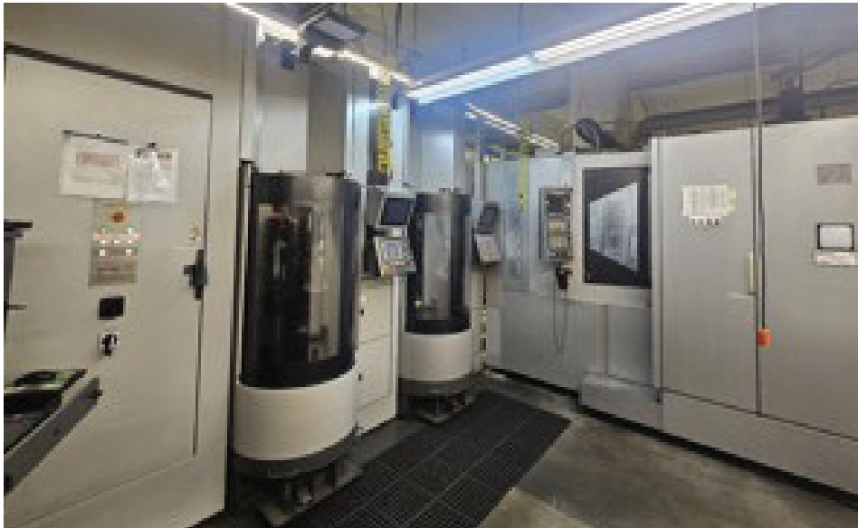
2) Toyoda FH 450 S Horizontal Machining Centers w/ Cell System, 17.7" x 17.7" Pallets, 23.62" x 23.62" x 23.62" (XYZ), w/ Fanuc 31i Model A Controls, 30 Pallets, 15K RPM, Cat 40 Tool, 494 ATC .
