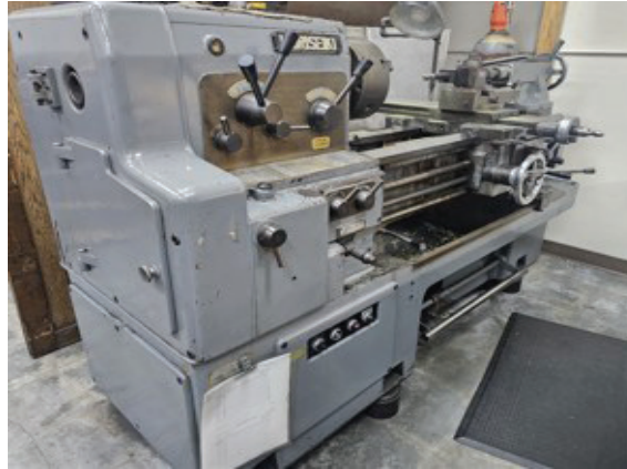
Mori Seiki MS- 850, 17"X33' Engine Lathe.
