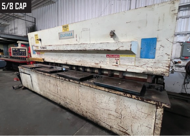
2001 DURMA AHGM 4016, 13FT X 5/8" CAPACITY HYDRAULIC SWING BEAM SHEAR, W/ POWERED BACK GAGE, S/N 622501042.
