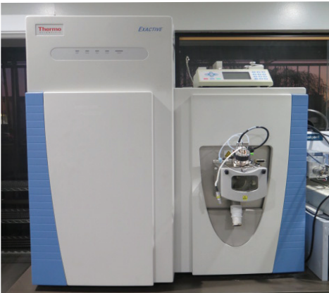
THERMO SCIENTIFIC EXACTIVE MASS SPECTROMETER W/ PUMP AND VACUUM PUMP
