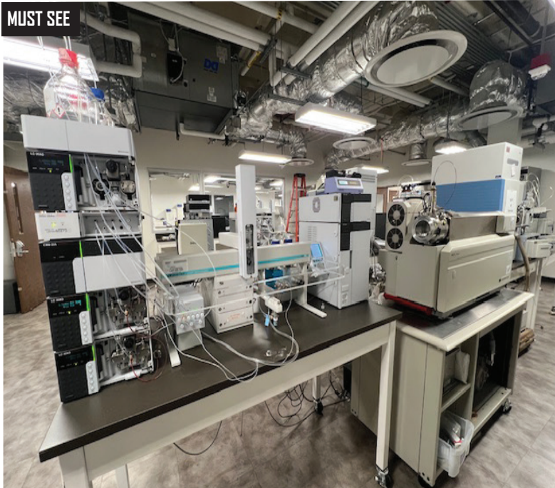
CTC ANALYTICS LEAP TECHNOLOGIES HTS PAL ROBOTIC AUTO SAMPLER LIQUID HANDLER / AND APPLIED BIOSYSTEMS MDS SCIEX 4000 QTRAP LC/MS/MS LIQUID CHROMATOGRAPH MASS SPECTROMETER SYSTEM.
