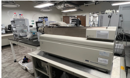
CTC ANALYTICS LEAP TECHNOLOGIES HTS PAL ROBOTIC AUTO SAMPLER LIQUID HANDLER / AND APPLIED BIOSYSTEMS MDS SCIEX 4000 QTRAP LC/MS/MS LIQUID CHROMATOGRAPH MASS SPECTROMETER SYSTEM.
