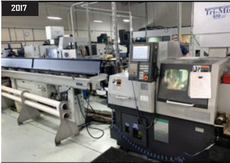
2017 Tsugami BO126-III CNC Swiss Screw Machine, w/ Live Tooling, Milling, C Axis, Y Axis, 12,000 RPM, 25 Position Turret and 8 Live Tool Position, 6 Axis, Edge Scout Barfeeder.
