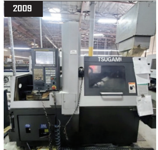
2009 Tsugami SS20 CNC Swiss Screw Machine, 10,000 RPM, w/ Live Tooling, 20mm Capacity, Live Milling, 10 Position Tool Positions, and Barfeeder 4564) Over 20 Aciera Swiss Model F3 Universal Toolmaker's Milling Machines.
