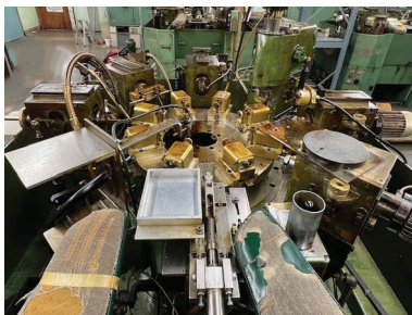
8 TOTAL (8) Mikron Haesler Model 50-8 and 59-8 Horizontal Table Transfer Machines, 8 Station Table, Vertical Units Including Cross Milling, Horizontal Milling, and Counter Boring. For Complex High Precision Simultaneous Drilling, Tapping, Reaming and Milling.
