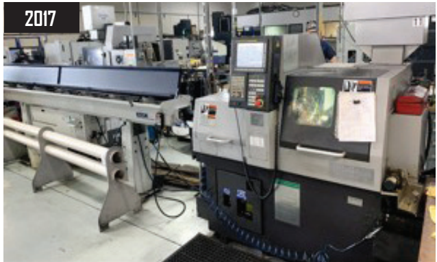
2017 2017 Tsugami BO126-III CNC Swiss Screw Machine, w/ Live Tooling, Milling, C Axis, Y Axis, 12,000 RPM, 25 Position Turret and 8 Live Tool Position, 6 Axis, Edge Scout Barfeeder.
