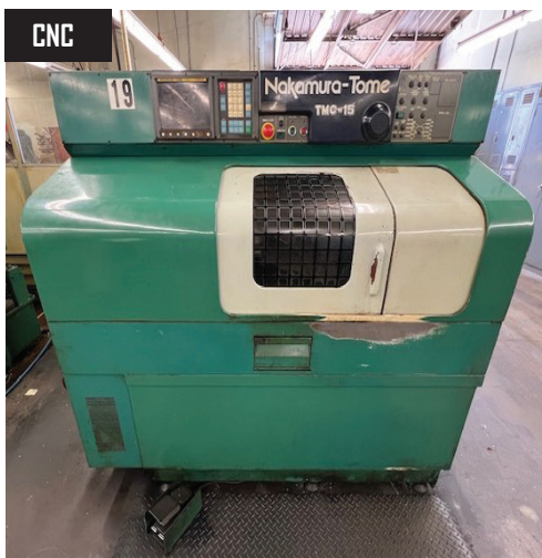
Nakamura Tome TMC-15 CNC Lathe, w/ Fanuc Control.
