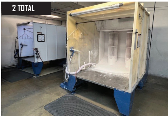
2) Nordson Model 18077 - 02 Powder Coating Booths with Nordson Encore Powder Coating Guns and Dust Collection System.
