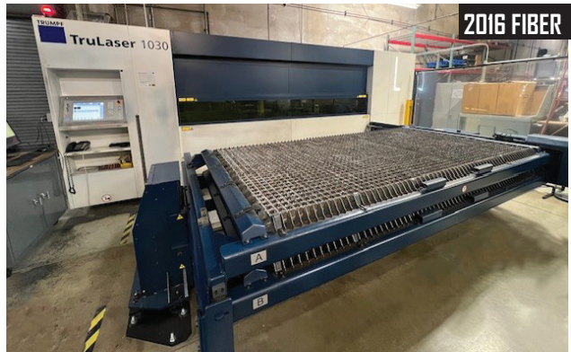
2016 Trumpf TruLaser 1030 Laser Cutting Machine, 2000 W Capacity, 60” x120” Cutting Area, TruDisk 2001 Resonator (Shared with Welder), s/n A0216L0155.
