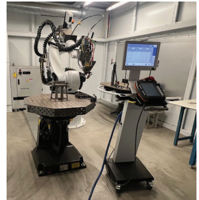
2016 Trumpf TruLaser Robot 5020, KRC4 Fiber Welding Cell, 3000 W Capacity, s/n A0455C0254, W/ 2016 Kuka KR 30 HA High Accuracy Robotic Welder, Dual Station Shuttle Table, Magnetic Coupling, 30 Meter Fiber Optic Laser Cable, s/n 701865.
