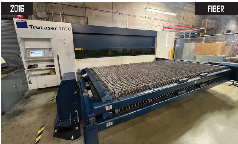
2016 Trumpf TruLaser 1030 Laser Cutting Machine, 2000 W Capacity, 60'' x 120'' Cutting Area, TruDisk 2001 Resonator (Shared with Welder), s/n A0216L0155.
