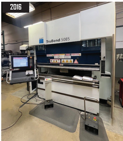
2016 Trumpf TruBend 5085 87'' x 95 Ton CNC Hydraulic Press Brake, 6 Axis Controls, Laser Safety Light Curtain, s/n B0502A0935.
