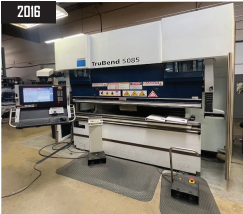
2016 Trumpf TruBend 5085 87” x 95 Ton CNC Hydraulic Press Brake, 6 Axis Controls, Laser Safety Light Curtain, s/n B0502A0935.
