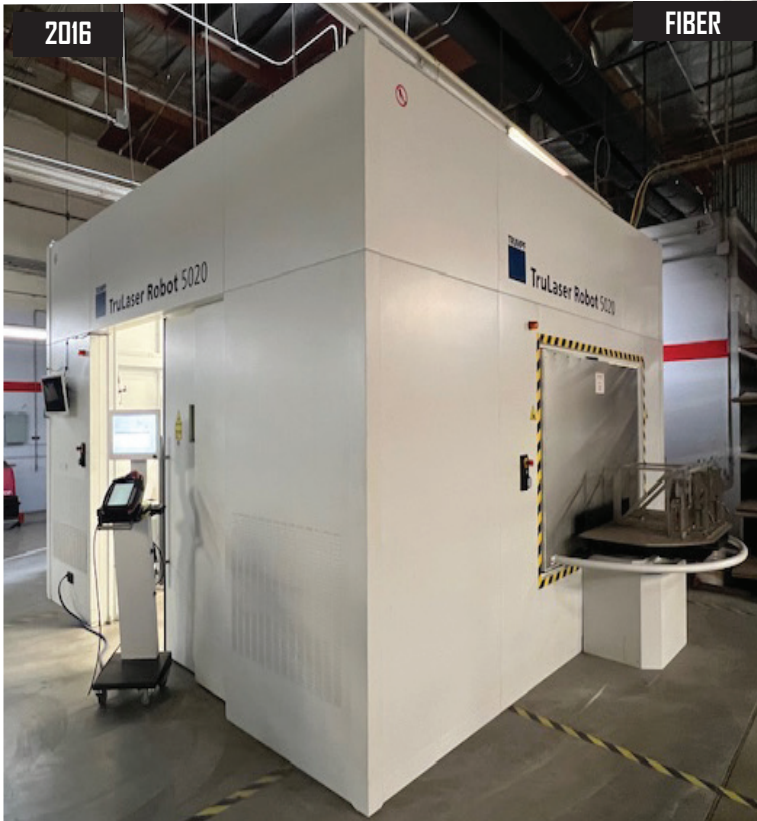
2016 Trumpf TruLaser Robot 5020, KRC4 Fiber Welding Cell, 3000 W Capacity, s/n A0455C0254, W/ 2016 Kuka KR 30 HA High Accuracy Robotic Welder, Dual Station Shuttle Table, Magnetic Coupling, 30 Meter Fiber Optic Laser Cable, s/n 701865.
