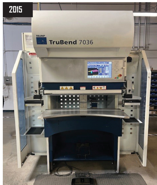
2015 Trumpf TruBend 7036 40'' x 40 Ton CNC Hydraulic Press Brake, 6 Axis Controls, TASC 6000 Control with 3D Graphics, Motorized Swivel Mounted Controls, 15'' Touch Screen, Laser Safety System, Hydraulic Tool Clamping, s/n B0702A1607
