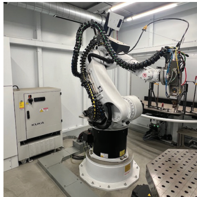
2016 Kuka KR 30 HA High Accuracy Robotic Welder, Dual Station Shuttle Table, Magnetic Coupling, 30 Meter Fiber Optic Laser Cable, s/n 701865.
