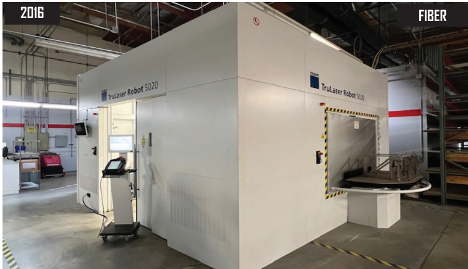
2016 Trumpf TruLaser Robot 5020, KRC4 Fiber Welding Cell, 3000 W Capacity, s/n A0455C0254, W/ 2016 Kuka KR 30 HA High Accuracy Robotic Welder, Dual Station Shuttle Table, Magnetic Coupling, 30 Meter Fiber Optic Laser Cable, s/n 701865.
