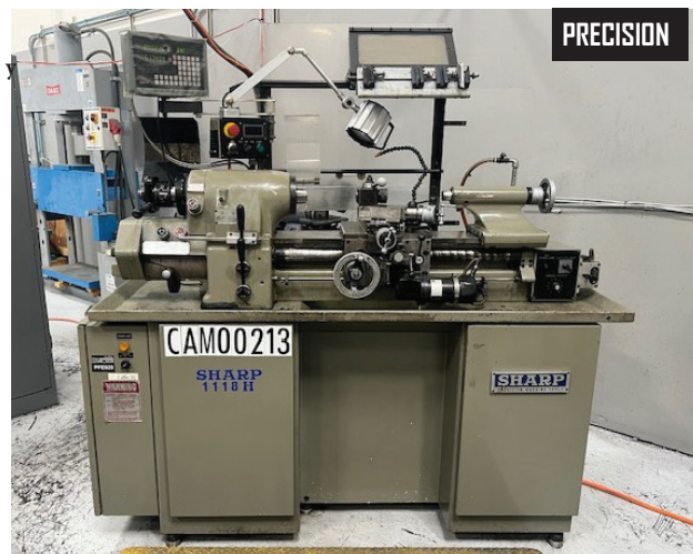
Sharp 1118H Wide-Bed Tool Room Lathe s/n CTL-1470 w/ Shars SDS6-2V Programmable DRO, Inch/mm Threading, Change Gears, Tailstock, Aloris Tool Post, Power Feeds, 5C Spindle, 6" 3-Jaw Chuck, 6" 4-Jaw Chuck.
