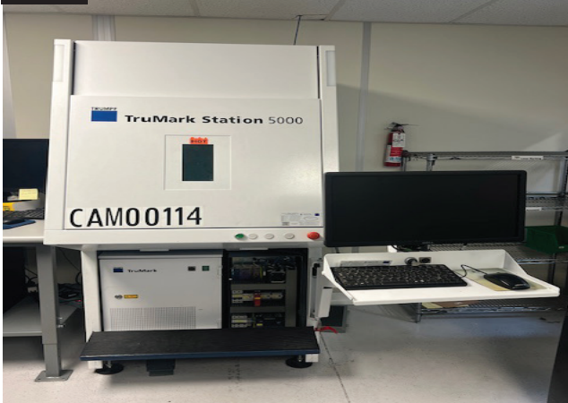
2014 Trumpf TruMark Station 5000 with TruMark 6000 Laser Marking System s/n L0160E1031 w/ Class 1 Laser, Travels X=11.8", Y=11.8", Z=15/19.7"; Vacuum System, Full Enclosure, Computer and Acces.
