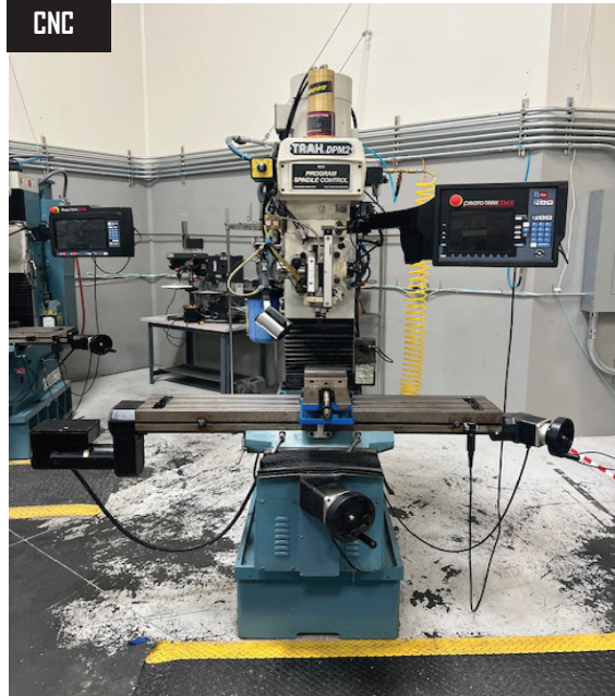
Trak DPM RX2 3-Axis CNC Vertical Mill s/n 202EA464 w/ Proto Trak RMX Controls, 3Hp Motor, 30-Taper Spindle, 40-5000 Controlled RPM, Torque-Rite Power Draw-Bar, Chrome Ways, 9' x 49' Table.
