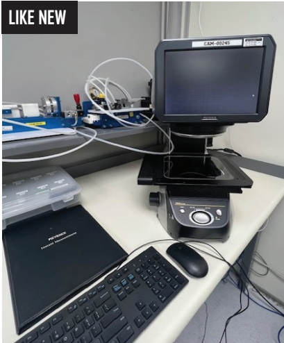
Keyence IM-7020 mage Dimension Measuring System s/n AC901322 w/ Keyence Software, 7.87" x 7.87" Wide Field Measurement Area, 4.92" x 4.92" High Precision Measurement Mode, 3.54" x 3.54" Light Probe Measurement Area.
