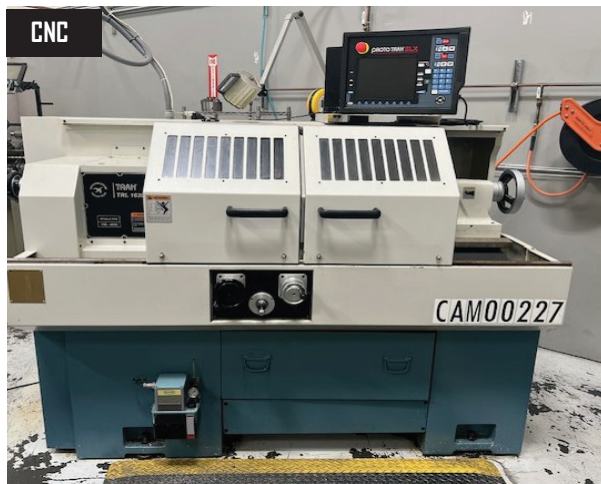
Trak TRL 1630 SX CNC Lathe s/n 181DG167 w/ Proto Trak SLX Controls, 15-0-4000 RPM, Tailstock, Dorian Tool Post, 6 1/2" 3-Jaw Chuck, 5C Spindle Nose.
