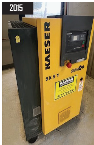
2015 Kaeser SX5T 5Hp Rotary Air Compressor s/n 1138 w/ Sigma Controls, 21 CFM @ 125 PSIG.
