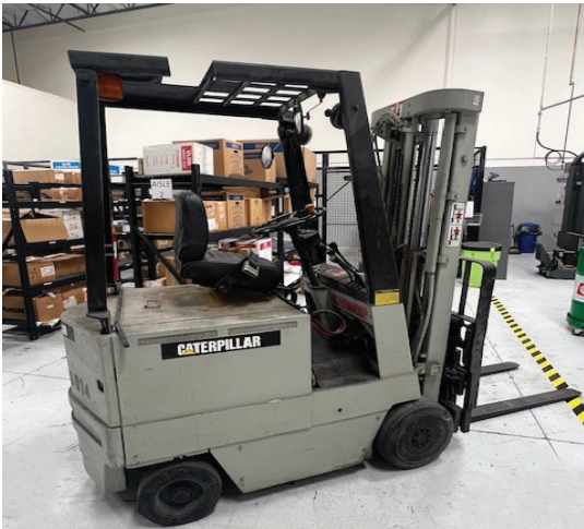
Caterpillar MC30 3000 Lb Cap Electric Forklift s/n 41W02235 w/ 3-Stager Mast, 156" Lift Height, Side Shift, Cushion Tires, Charger.
