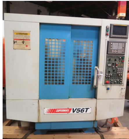
SUPERMAX V56T CNC VERTICAL MACHINING CENTER W/ FANUC SERIES 18-M CONTROLS
