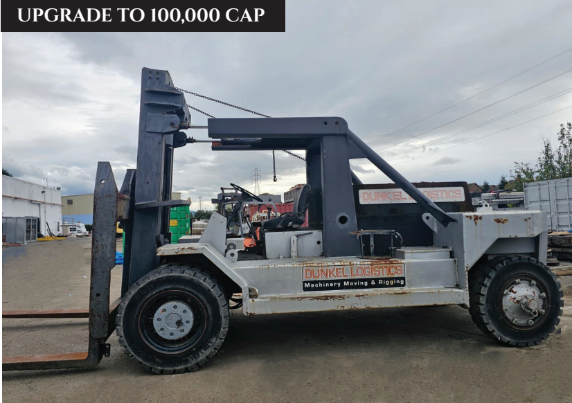
TAYLOR 40/60 40,000-60,000 LB CAP FORKLIFT IN RETROFIT CONDITION W/ 100,000 LB CYLINDER AND MISC.
