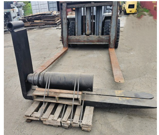
TAYLOR 40/60 40,000-60,000 LB CAP FORKLIFT IN RETROFIT CONDITION W/ 100,000 LB CYLINDER AND MISC.
