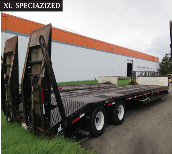
XL SPECIALIZED TRAILERS XL90SD DROP DECK SEMI TRAILER W/ HYDRAULIC RAMPS
