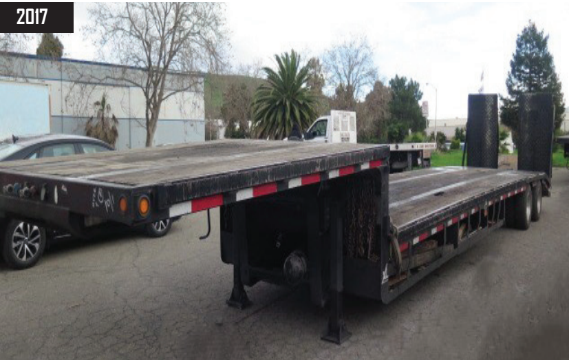
2017 XL SPECIALIZED TRAILERS XL90SD DROP DECK SEMI TRAILER W/ 105,645 GVWR, 22,700 GAWR, HYDRAULIC RAMPS
