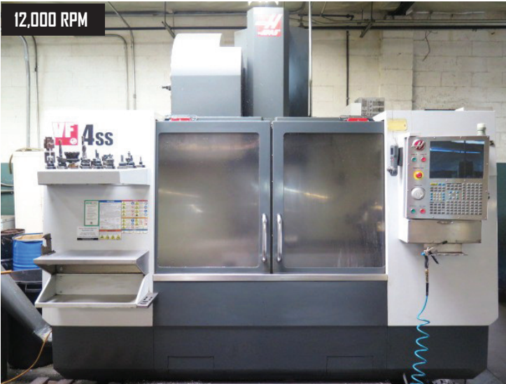
2011 Haas VF-4SS 4-Axis CNC VMC w/ Haas Controls, Hand Wheel. 40-Station Side Mount ATC, CAT-40 Taper Spindle, Renishaw Wireless System
