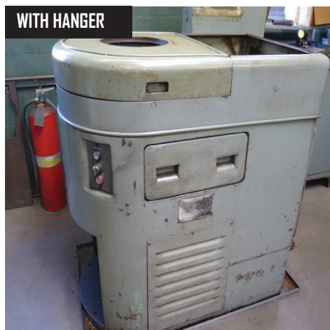
Reed Thread Rolling Machine w/ Hanger.
