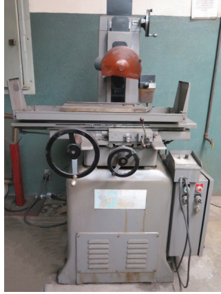
Boyar Schultz Challenger 2A 6" x 18" Automatic Surface Grinder
