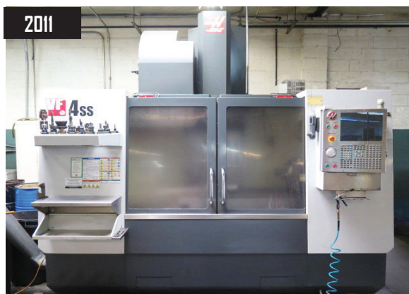
2011 Haas VF-4SS 4-Axis CNC VMC w/ Haas Controls, Hand Wheel. 40-Station Side Mount ATC, CAT-40 Taper Spindle, Renishaw Wireless System
