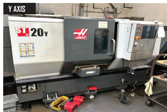
2013 Haas ST-20Y “Y” Axis – Live Turret CNC Turning Center s/n 3097730 w/ Haas Controls, Tool Presetter, 12-Station 6-Live Position Turret
