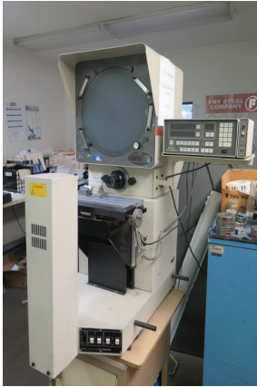
Mitutoyo PH-3500 15" Optical Comparator w/ Micropak 2 Programmable DRO
