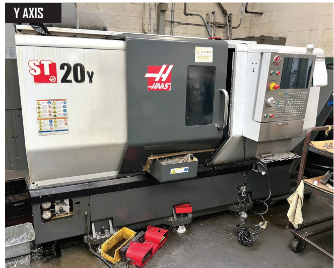
2013 Haas ST-20Y "Y" Axis - Live Turret CNC Turning Center s/n 3097730 w/ Haas controls, Tool Presetter, 12-Station 6-Live Position Turret, Tailstock, 4000 RPM, "C"Axis, Rigid Tapping, M19 Spindle Orientation, Quick Code, Haas Vector Drive, 8" 3-Jaw power Chuck, Chip Conveyor, Coolant, LNS Hydrobar Hydraulic Bar Feed.
