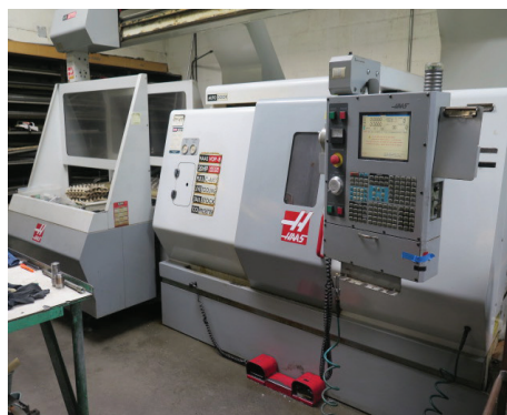
2002 Haas SL-20 TAPL CNC Live Turret Turning Center w/ APL Automatic Parts Loader, Tool Presetter, 10-Station Live Turret, Tailstock, 4000 RPM
