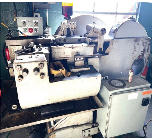
Waterbury Farrel #30 Thread Rolling Machine
