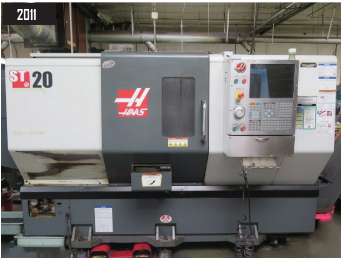
2011 Haas ST-20 CNC Turning Center s/n 3088929 w/ Haas Controls, Tool Presetter, 12-Station Turret, Tailstock, Brown & Sharpe Colletted Spindle Nose, Coolant, LNS Hydrobar Hydraulic Bar Feed.
