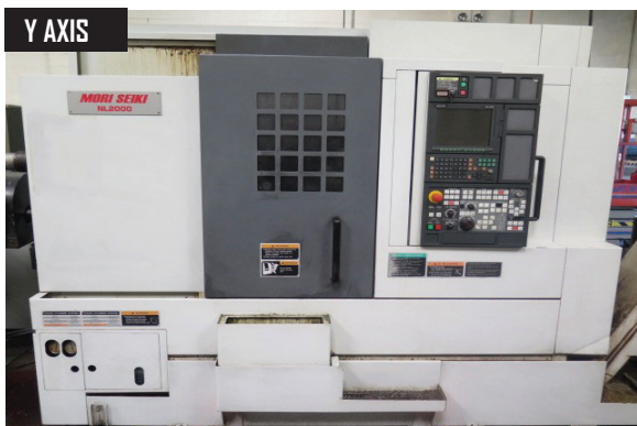
2009 Mori Seiki NL2000SY / 500 Twin Spindle – Live Turret CNC Turning Center w/Mori Seiki MSX-850 III Controls, Tool Presetters, 12-Station Live Turret, “C” Axis, Synchronized Spindles, 8” 3-Jaw Main Power Chuck, 6 ½” 3-Jaw Sub Power Chuck, Hardinge Colleted Main Spindle Nose, Chip Conveyor, Coolant, LNS Hydrobar BarFeeder.
