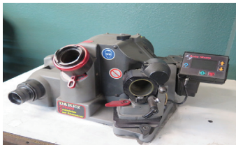
Darex TX-3000 Expandable Tool Sharpener w/ Auto-Sharp Control
