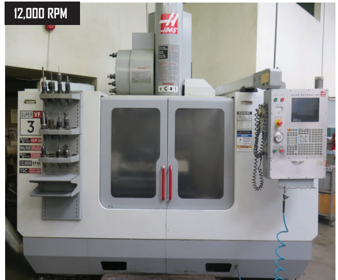
2004 Haas VF-3SS 5-Axis Trunnion VMC w/ Haas 4 th /5 th Axis 6" Trunnion Rotary, 24-Station Side-Mount ATC, CAT-40 Spindle, 12,000 RPM
