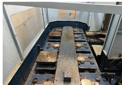
Matsuura H. Plus 300 PC 11 CNC HMC w/ 11 Pallet System, 300 mm Pallets, 240 ATC, CT 40, Matsuura G Tech 30i Control, 4 Axis.
