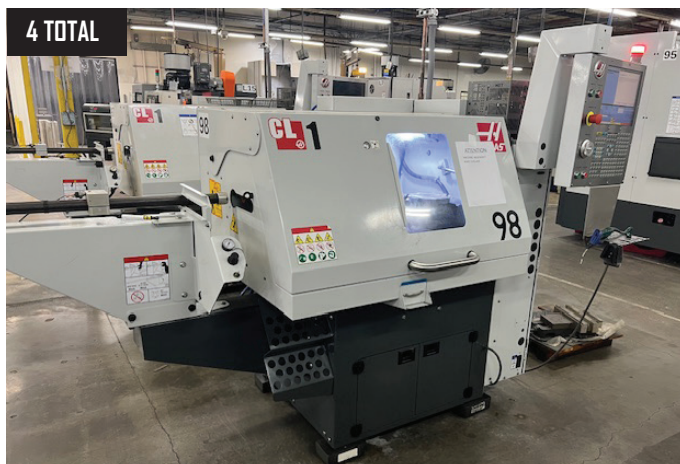
4 Total) 2018 HAAS CL-1 CNC Lathe, Equipped with HAAS CNC control, 6000 RPM/5 HP spindle, 8 station turret, gang-style tooling, bar feeder.
