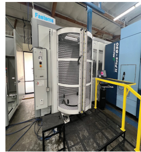
2/2012 Matsuura H-Plus 630 HMC's with 41.33"x,36.2"y,38.97"z travels, 630 mm pallets, CAT 50 spindle, 12,000 RPM speed, 4-axis, 150 tool ATC,. Equipped with FANUC 30i, w Fastems Model FPC-1500 10 Pallet Cell System.
