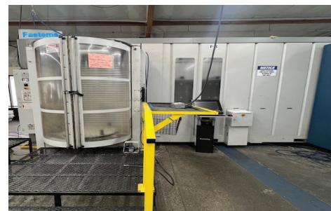
2/2012 Matsuura H-Plus 630 HMC's with 41.33"x,36.2"y,38.97"z travels, 630 mm pallets, CAT 50 spindle, 12,000 RPM speed, 4-axis, 150 tool ATC,. Equipped with FANUC 30i, w Fastems Model FPC-1500 10 Pallet Cell System.
