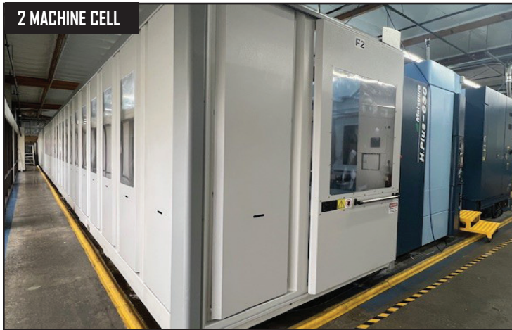
2013 & 2014 Matsuura H-Plus 630 HMC's with 41.33"x,36.2"y,38.97"z travels, 630 mm pallets, CAT 50 spindle, 12,000 RPM speed, 4-axis, 120 tool ATC and 150 tool ATC, dual 24.8" pallets. Equipped with FANUC 30i, high-speed options, w Fastems Model FPC-1500 20 Pallet Cell System.
