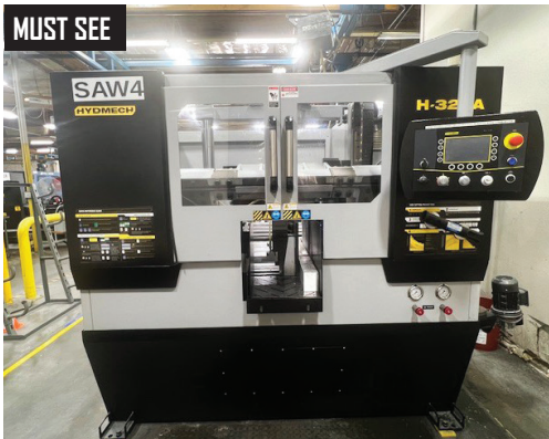
HYD MECH HA-320 Automatic Horizontal Band Saw, with CNC Controls.
