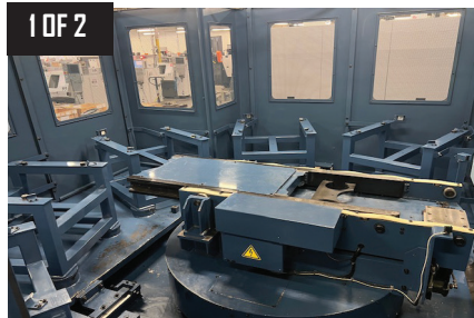
1 Of 2) 2008 & 2006 Matsuura H. Plus 630 PC-6 HMC's w/ 6 Pallet System, 41.33" x, 36.27" y, 38.97" z, 630 mm pallets, CAT 50 spindle, 12,000 RPM speed, 4-axis, dual 24.8" pallets. Equipped with G Tech 30i Controls, High Pressure Coolant.
