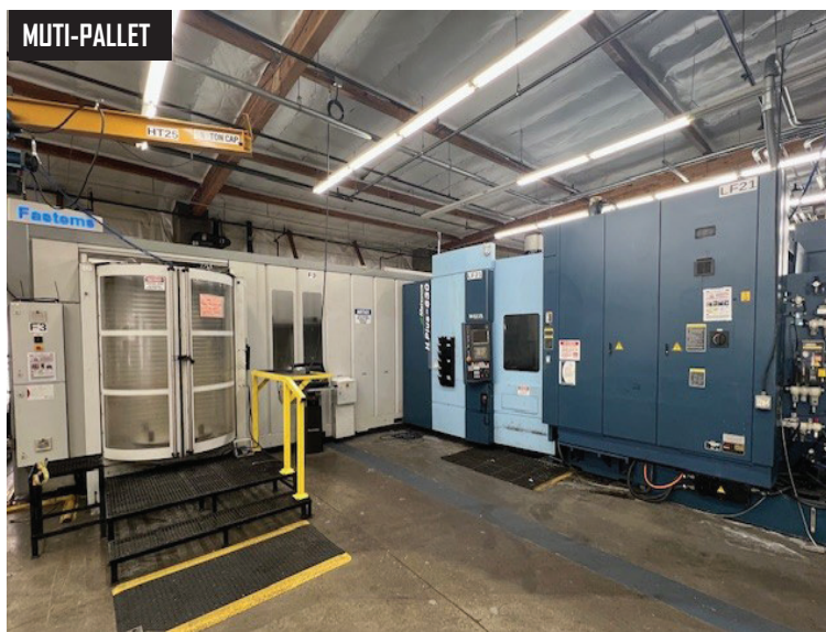
2014 Matsuura H-Plus 630 HMC's with 41.33"x,36.2"y,38.97"z travels, 630 mm pallets, CAT 50 spindle, 12,000 RPM speed, 4-axis, 150 tool ATC, dual 24.8"pallets.
