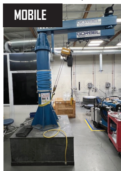
Gorbelt 1000 lb Capacity Mobile Crane System.
