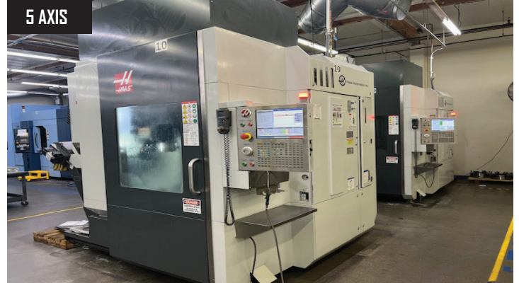
2 of 4) 2016 2017 Haas UMC-750 SS 5 Axis CNC VMC w/ 12,000 RPM, CT 40 Taper.
