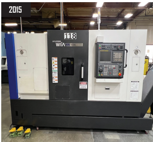
2015 HYUNDAI WIA L300A CNC Lathe Swing: 27.725" Machining Length: 28.35" 30 hp, Max RPM: 3600. Equipped with FANUC i-SERIES Control.
