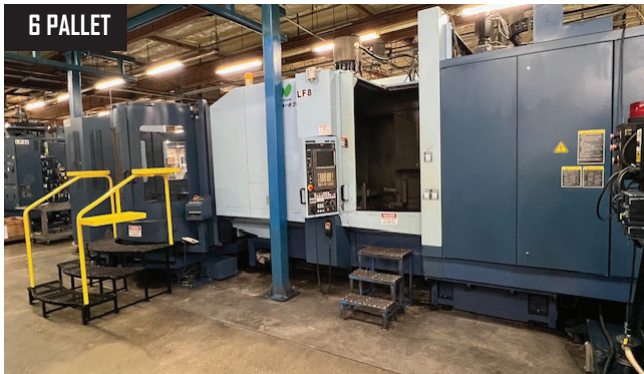
1 Of 2) 2008 & 2006 Matsuura H. Plus 630 PC-6 HMC's w/ 6 Pallet System, 41.33" x, 36.27" y, 38.97" z, 630 mm pallets, CAT 50 spindle, 12,000 RPM speed, 4-axis, dual 24.8" pallets. Equipped with G Tech 30i Controls, High Pressure Coolant.
