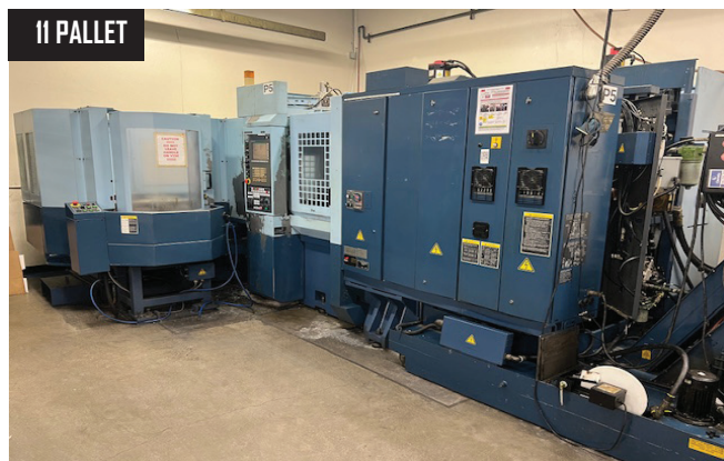
Matsuura H. Plus 300 PC 11 CNC HMC w/ 11 Pallet System, 300 mm Pallets, 240 ATC, CT 40, Matsuura G Tech 30i Control, 4 Axis.
