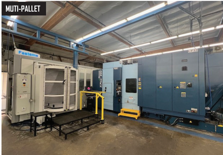
2/2012 Matsuura H-Plus 630 HMC's with 41.33"x,36.2"y,38.97"z travels, 630 mm pallets, CAT 50 spindle, 12,000 RPM speed, 4-axis, 150 tool ATC,. Equipped with FANUC 30i, w Fastems Model FPC-1500 10 Pallet Cell System.
