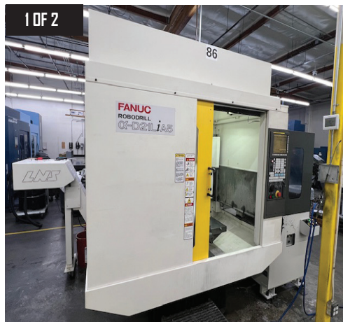
1 of 2) 2016 FANUC ROBODRILL a-D21LiA5, equipped with FANUC 31i-B5, 2 pallet system, tool presetter, MistBuster, LNS chip conveyor. 20,000 RPM, 24 ATC, and tool probe.
