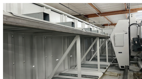
2014 Matsuura H-Plus 630 HMC's with 41.33"x,36.2"y,38.97"z travels, 630 mm pallets, CAT 50 spindle, 12,000 RPM speed, 4-axis, 150 tool ATC, dual 24.8"pallets.
