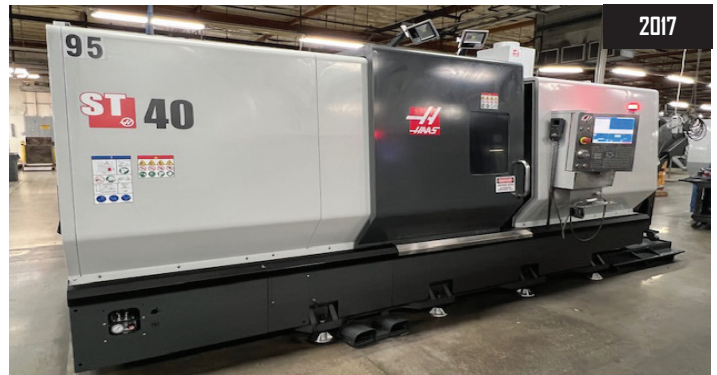
12/2017 Haas ST-40 CNCLathe, 15" chuck, 34.5" Swing, 40 hp, 240 RPM. 4.0" Spindle Bore, 44" Machining Length, Includes HAAS CNC Control, s/n 3109357.
