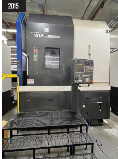
2015 Hyundai WIA LV1100R VTL Vertical CNC with 39.5" chuck. Features 60 hp main motor, 800 RPM speed, 12 station ATC, FANUC 32i control, tool presetter, part probe, and chip conveyor.
