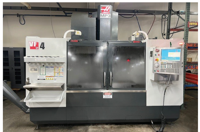
2011 HAAS VF-4, VMC, w/ 50"x20"x25" (XYZ) in travel, 40-ATC, 10,000 RPM spindle, CT 40 Taper, HAAS CNC control, wireless probing.
