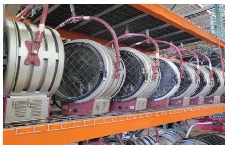
Mole-Richardson mdl. 8331 5000 Watt 24" Molebeam
