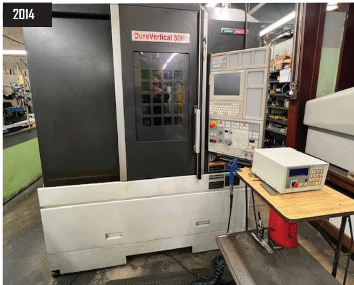
2014 Mori Seiki Dura Vertical 5060 CNC VMC, BT 40 Taper, 4 Axis Ready, 12,000 rpm, Fanuc OiMD Controls, 30 ATC, 23.6" x 20.9" x 201.1" (XYZ), Chip Auger, s/n DV005131205.
