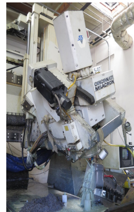
Cincinnati Milacron 30V Bridge Profiler 5-Axis CNC Bridge Mill w/ Siemens Acromatic 950 Controls, 50-Taper Spindle, 30Hp
