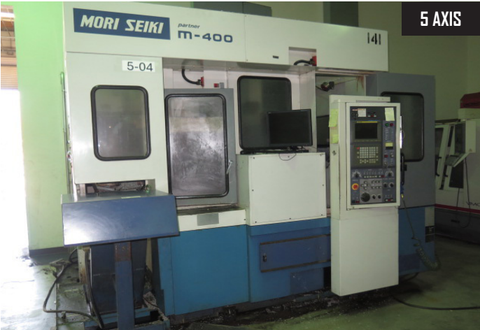
Mori Seiki Partner M-400 2-Pallet 5-Axis CNC VMC w/ Fanuc MF-M6 Controls, 60-ATC, HSK63 Spindle, 15,000 RPM
