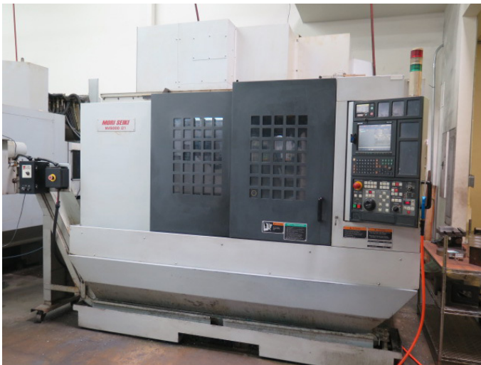
Mori Seiki NV50001 CNC VMC w/ MSX-501 Controls, 24-ATC, CAT-40, Renishaw Wireless System
