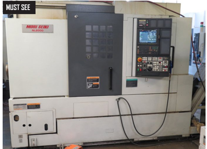
Mori Seiki NL2000 CNC Turning Center w/ Mori MSX-850 Controls, Tool Presetter, 5000 RPM, 12-Station Turret, Tailstock, 8" Chuck
