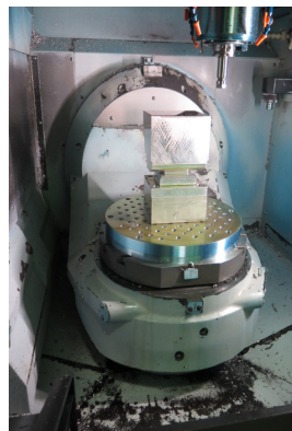
2008 Mori Seiki NMV-5000 DCG 5-Axis CNC Vertical Machining Center s/n NM501HA0119 w/ DMG Mori MSX-711 III Controls, Hand Wheel, 60-Station ATC, HSK63 Spindle, Tool Presetter, Renishaw Wireless System, 20" Rotary, 12,000 RPM, 4th Axis +160 Deg to -180 Deg, 5th Axis 360 Deg, Coolant.
