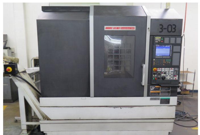
Mori Seiki Dura Vertical 5080 CNC VMC w/ MSC-504 III Controls, 30-ATC, CAT-40, 10,000 RPM, Renishaw Wireless System
