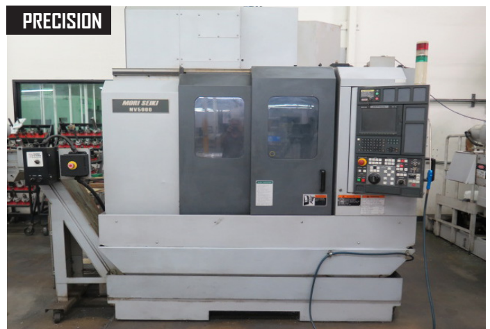
Mori Seiki NV5000 CNC VMC w/ Mori MSG-501 Controls, 24-ATC, CAT-40, Renishaw System, Renishaw Touch Probe
