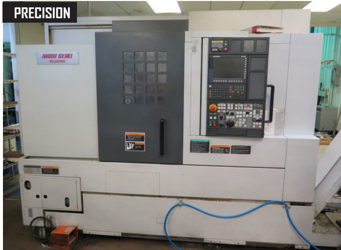
Mori Seiki NL2000 CNC Turning Center w/ DMG Mori MSX-850 III Controls, Tool Presetter, 5000 RPM, 12-Station Turret, Tailstock, 8" Chuck
