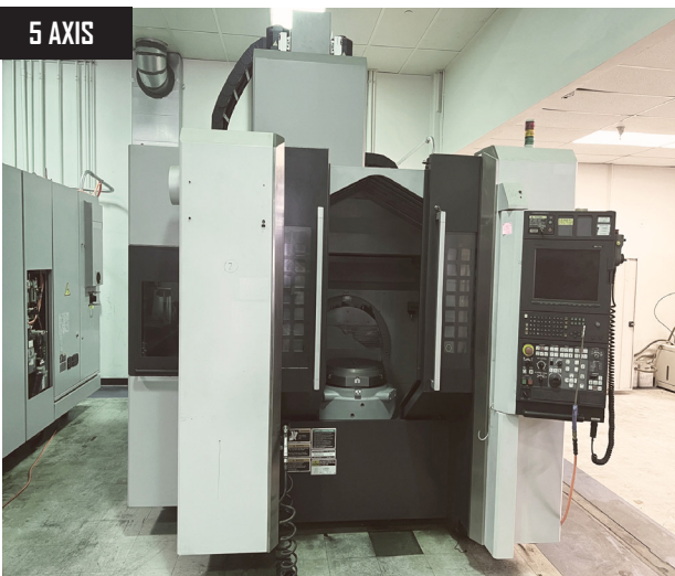
2008 Mori Seiki NMV-5000 DCG 5-Axis CNC Vertical Machining Center s/n NM501HA0119 w/ DMG Mori MSX-711 III Controls, Hand Wheel, 60-Station ATC, HSK63 Spindle, Tool Presetter, Renishaw Wireless System, 20" Rotary, 12,000 RPM, 4th Axis +160 Deg to -180 Deg, 5th Axis 360 Deg, Coolant.
