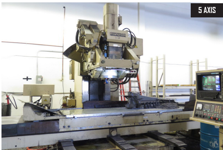
Cincinnati Milacron 5-Axis CNC VMC w/ Cincinnati Milacron Acromatic 950 Controls, 50-Taper Spindle, 20Hp, 20-3600 RPM
