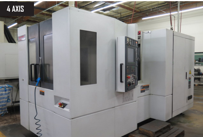
Mori Seiki NH-4000 CD 2-Pallet 4-Axis CNC HMC w/ Mori MSX-701 III Controls, Tool Presetter, 40-ATC, CAT-40, Renishaw System, Renishaw CAT-40 Probe
