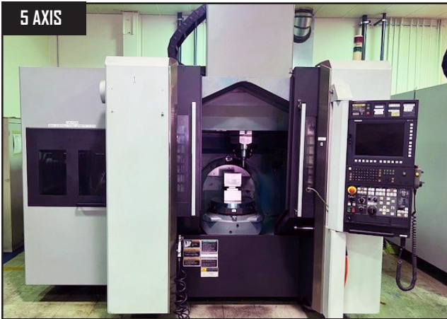
2008 Mori Seiki NMV-5000 DCG 5-Axis CNC Vertical Machining Center s/n NM501HH0340 w/ DMG Mori MSX-711 III Controls, Hand Wheel, 120-Station ATC, HSK63 Spindle, Tool Presetter, Renishaw Wireless System, 20" Rotary, 12,000 RPM, 4th Axis +160 Deg to -180 Deg, 5th Axis 360 Deg, Coolant.
