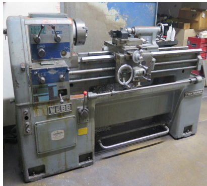
Takisawa Webb TSL-1000D 14" x 40" Geared Head - Gap Bed Lathe
