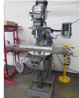
Bridgeport Vertical Mill w/ Newall C80 3-Axis DRO
