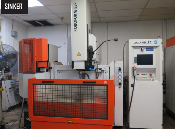
Charmilles RoboForm 55P Die Sinker EDM w/ Charmilles Controls, System 3R 12-Station Tool Changer, System 3R Tooling Head
