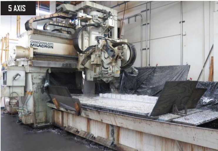
Cincinnati Milacron 30V Bridge Profiler 5-Axis CNC Bridge Mill w/ Siemens Acromatic 950 Controls, 50-Taper Spindle, 30Hp
