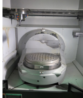
2008 Mori Seiki NMV-5000 DCG 5-Axis CNC Vertical Machining Center s/n NM501HH0340 w/ DMG Mori MSX-711 III Controls, Hand Wheel, 120-Station ATC, HSK63 Spindle, Tool Presetter, Renishaw Wireless System, 20" Rotary, 12,000 RPM, 4th Axis +160 Deg to -180 Deg, 5th Axis 360 Deg, Coolant.
