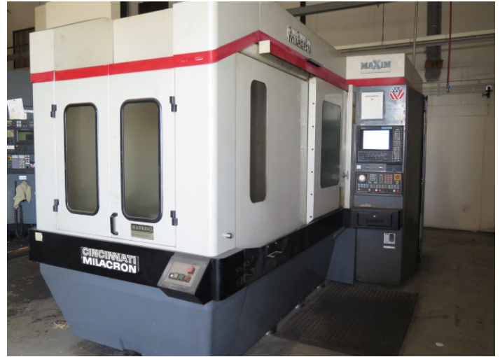
Cincinnati Milacron "Maxim Five Hundred" 2-Pallet CNC HMC w/ Acramatic 950 Controls, Tool Presetter, 80-ATC, CAT-50, 19 3/4" x 19 3/4" Pallets
