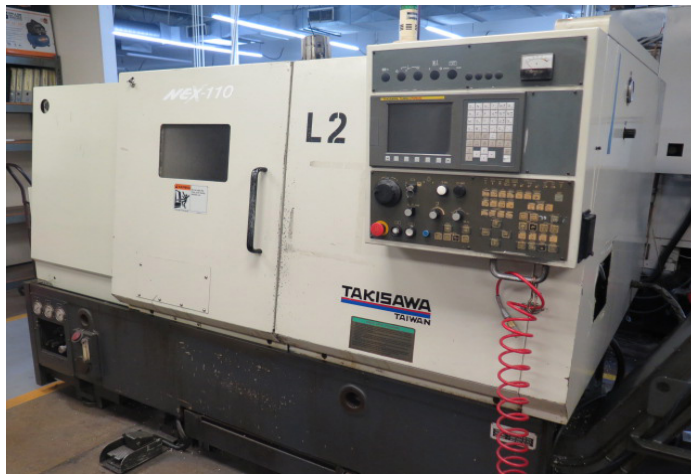
Takisawa NEX-110 CNC Turning Center w/ Takisawa Turn - i Fanuc Controls, 10-Station Turret, Tailstock, 12" Chuck
