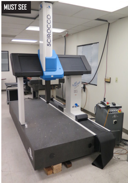
DEA Scirocco Slant Bridge CMM Machine w/ Renishaw PH10MQ Motorized Probe, PHC10B Controller, Joystick Controls
