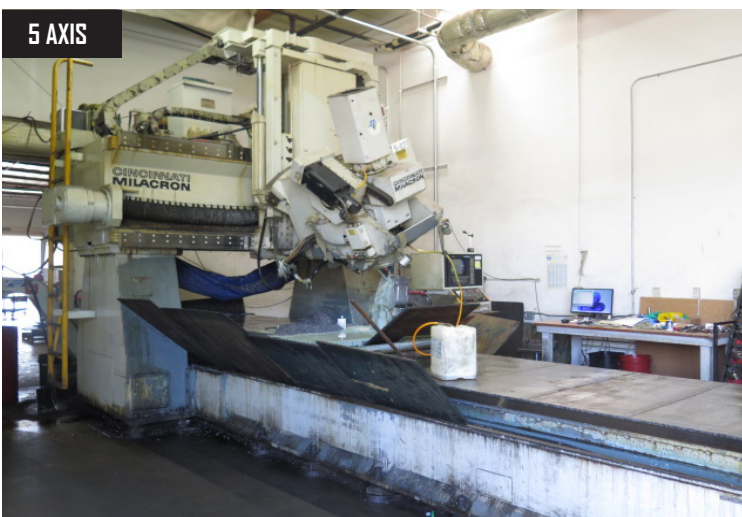
Cincinnati Milacron 30V Bridge Profiler 5-Axis CNC Bridge Mill w/ Siemens Acromatic 950 Controls, 50-Taper Spindle, 30Hp
