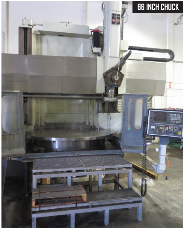
Bullard 66" CNC VTL w/ Fanuc 18-T Controls, 5-Station Turret, 66" Chuck, 80" Top Plate
