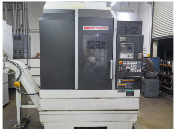
Mori Seiki Dura Vertical 5068 CNC VMC w/ MSC-504 Controls, 30-ATC, CAT-40, 10,000 RPM, Renishaw Wireless System, Renishaw Probe
