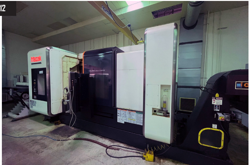
2012 Mazak Integrex i-300S Intelligent /Multi-Tasking Twin Spindle CNC Turning Center w/ Mazatrol Matrix 2 Controls, 120-ATC, Capto C6, "Y" Axis, "B" Axis Live Tooling, 4000 Main and Sub Spindle RPM, 12,000 Milling RPM
