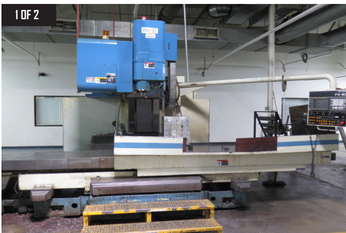
Kafo / Femtec FV-80 CNC VMC w/ Fanuc 18-M Controls, 30-ATC, CAT-50
