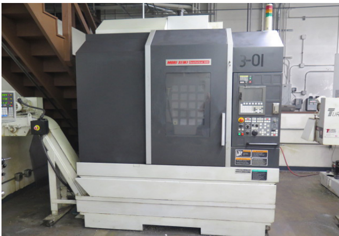
Mori Seiki Dura Vertical 5080 CNC VMC w/ MSC-504 III Controls, 30-ATC, CAT-40, 10,000 RPM, Renishaw Wireless System
