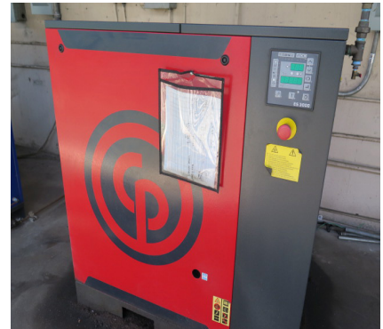
2015 Chicago Pneumatic CP QRS30 30Hp Rotary Air Compressor
