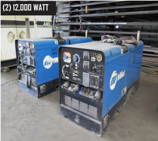
(2) Miller Trailblazer Pro 350D Diesel CC/CV-DC Welder – 12,000 Watt Generators.
