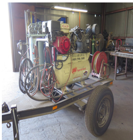
Ingersoll Rand Towable Gas Powered Air Compressor.
