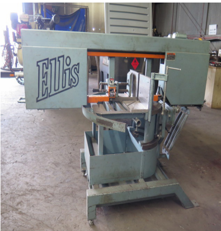
Ellis mdl. 2000 11" Horizontal Miter Band Saw s/n 2060191057 w/ Manual Clamping.
