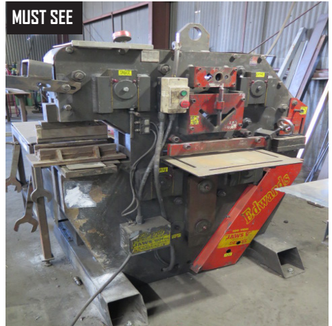
Edwards 100 Ton Deluxe Iron Worker s/n 11410103 w/ Punch Head with 12" Brake Attachment, 6" x 5" Angle Shear, 1" Square and Round Bar Shears, 18" Flat Shear, Coping Notcher.
