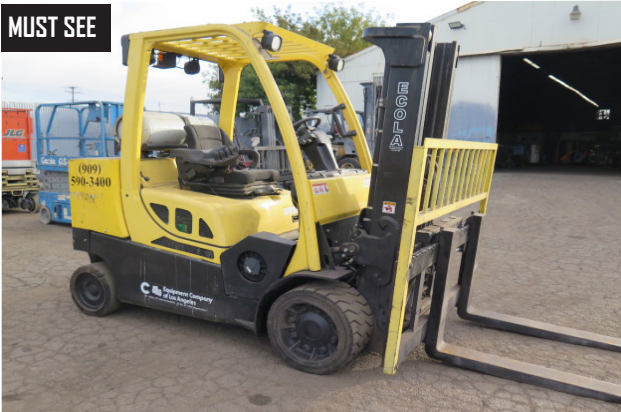
MUST SEE Hyster S120FTS 12,000 Lb Cap LPG Forklift s/n J004V03026 w/ Finger-Tip Controls, Monotro Trans, 2-Stage Mast, 111" Lift Height, Hydra-Smooth Cushioner, Side lift, 6' Fork Width, Cushion Tires, 3853 Hours.
