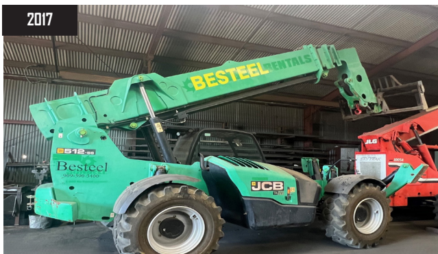
2017 2017 JCB 512-56F 12,000 Lb Cap Telehandler VIN#1CB5CH2GKH2502888 w/ Diesel Engine, 52' Boom Height, 42' Reach, Crab Steering, Outriggers, Boom Attachment.
