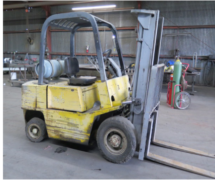
Yale GLF050ROJUA080 5000 Lb Cap LPG Forklift s/n Y427795 w/ 2-Stage Mast, Solid Yard Tires.
