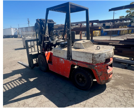
Nissan 8750 Lb Cap LPG Forklift w/ 3-Stage Mast, 6' Fork Width, Side Shift, Solid Yard Tires.
