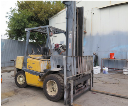
Yale GLP080LFNSBV110 8000 Lb Cap LPG Forklift s/n D970259 w/ 2-Stage Mast, 170" Lift Height, Side Shift, 6' Fork Width, Yard Tires.
