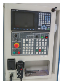
2008 Akira Seiki Performa V4 CNC VMC w/ Akira Seiki Mi645 Controls, 20-Station ATC, CAT-40 Spindle
