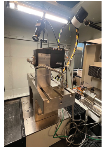
2023 Ametek Nanoform 700 Ultra A21200-01 REV. H Multi Axis Precision Machining System, For Production of Optical lenses, Mirrors and Mechanical Components, 80,000 RPM Spindle Head, 700mm Swing and 170kg Load Capacity, Video System, Surface Finish of 1nm Ra, 350x mm and 300z Travel Oil Hydrostatic Machine Slides, Ametek Cooling System, FTS5000 Diamond Holder.
