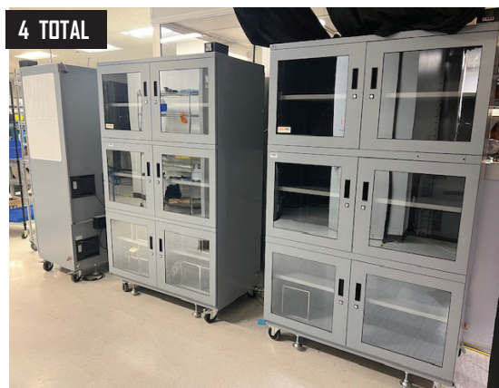
4) Stat Pro CPDC-60-NS, 6 Door Automatic Desiccant Dehumidifiers w/ Nitrogen Controlled.
