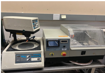
Buehler Ecomet 4 Var Speed Grinder/Polisher w/ Automated Powerhead and MTI SYJ-200 Precision Saw w/ PLC Controls.
