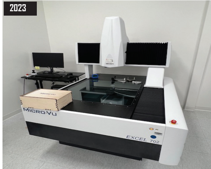
2023 Micro-Vu Model Excel 702 Non Contact and Multisensor Measuring Machine, 660 x700 x 250 mm Measuring Volume, 500 mm/s x and y Max Speed, 250 mm/s z Max Speed, 100Kg Capacity, s/n EC70201100.
