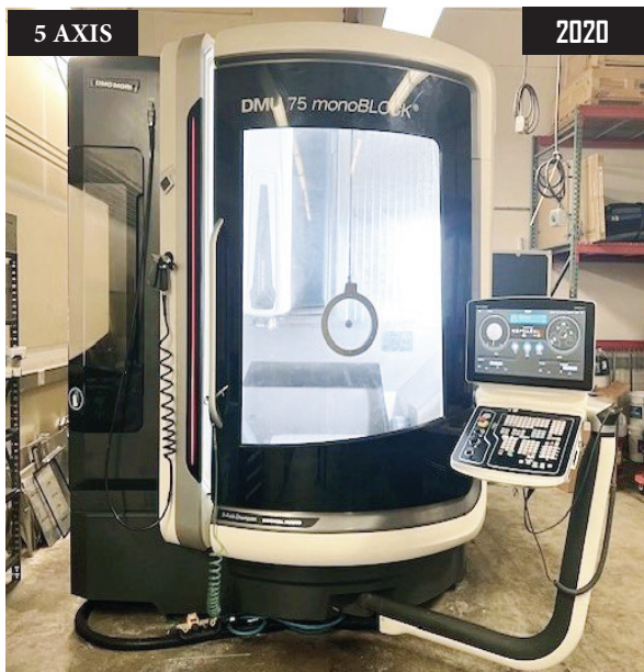
2020 DMG MORI DMU 75 Mono Block 5 Axis Simultaneous Vertical Machining Center, 750mm x 650mm x 560mm (XYZ), 600Kg Max Workpiece Weight, Siemens ERGoline Controls, 60 ATC, HSK 63 Tool, s/n 12430015053.6359.
