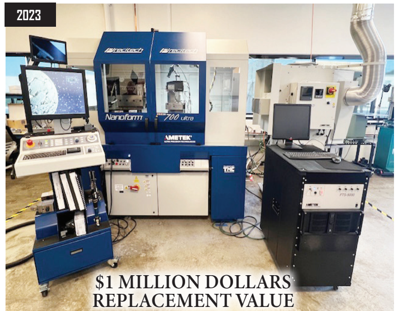
2023 Ametek Nanoform 700 Ultra A21200-01 REV. H Multi Axis Precision Machining System, For Production of Optical lenses, Mirrors and Mechanical Components, 80,000 RPM Spindle Head, 700mm Swing and 170kg Load Capacity, Video System, Surface Finish of 1nm Ra, 350x mm and 300z Travel Oil Hydrostatic Machine Slides, Ametek Cooling System, FTS5000 Diamond Holder.
