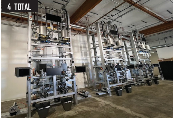
View of Adventek Engineering Twin Fiber Optics Draw Towers.
