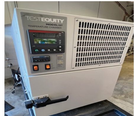
Testequity Model 107 Temperature Chamber, -42c to 130c Range.
