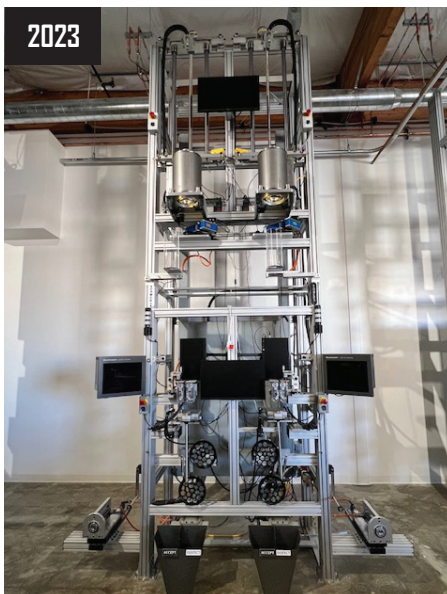
1 of 3) Advantek Engineering Twin Fiber Optic Draw Tower Extruders, w/ Two Stations, s/n A42018-1, A42018-2, A42018-3, w/ Zumbach USYS Touch Controls, Dual Zone,
