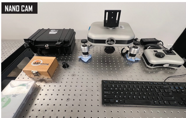
Nano Cam 4D HD Dynamic Optical Profiler for Measurement of Surface Roughness for Coated and Uncoated Optics, Metals, Plastics and Other Polished Specular Surfaces, 5MP, 12-bit Camera, 4Sights Focus Software, Pulsed LED at 460nm, 100 usec Acquisition Time.
