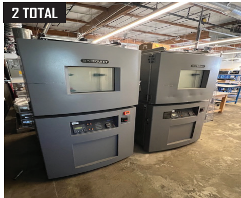
2) Testequity 1000 Series Temperature Chamber, -75c to 175c range, model 1007C.
