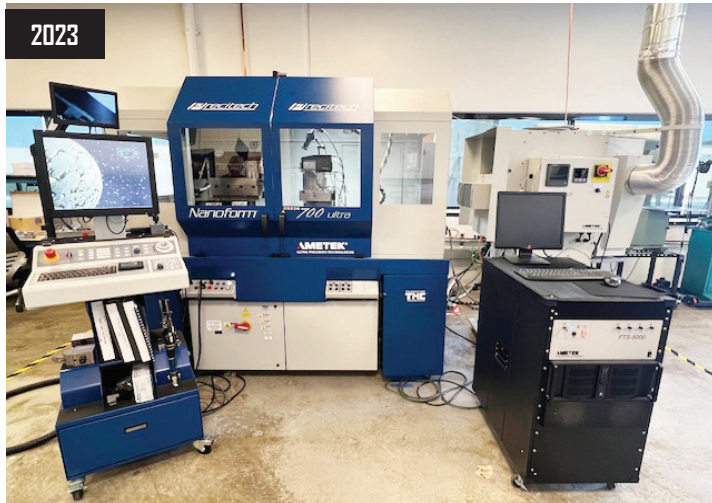
2023 Ametek Nanoform 700 Ultra A21200-01 REV. H Multi Axis Precision Machining System, For Production of Optical lenses, Mirrors and Mechanical Components, 80,000 RPM Spindle Head, 700mm Swing and 170kg Load Capacity, Video System, Surface Finish of 1nm Ra, 350x mm and 300z Travel Oil Hydrostatic Machine Slides, Ametek Cooling System, FTS5000 Diamond Holder.
