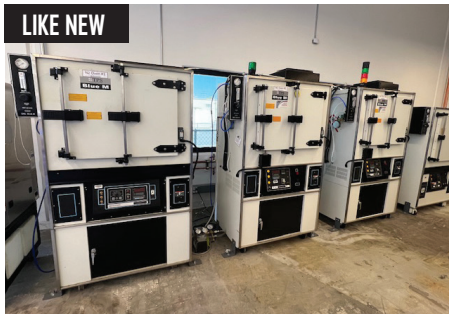
3) Blue M Inert Gas Ovens, Model DCI-296-6-F4T-ETO, 662F Max Temperature.
