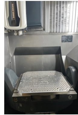
2020 DMG MORI DMU 75 Mono Block 5 Axis Simultaneous Vertical Machining Center, 750mm x 650mm x 560mm (XYZ), 600Kg Max Workpiece Weight, Siemens ERGOline Controls, 60 ATC, HSK 63 Tool, s/n 12430015053.6359
