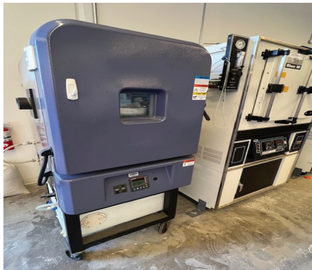
Espec BTX-475 Thermal Test Chamber / Temp & Humidity Chmber-70c to 180c.
