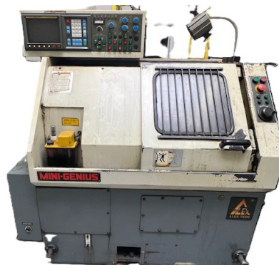
Alex Tech Mini Genius CNC Gang Tool Lathe, w/ Fanuc O-T Controls.
