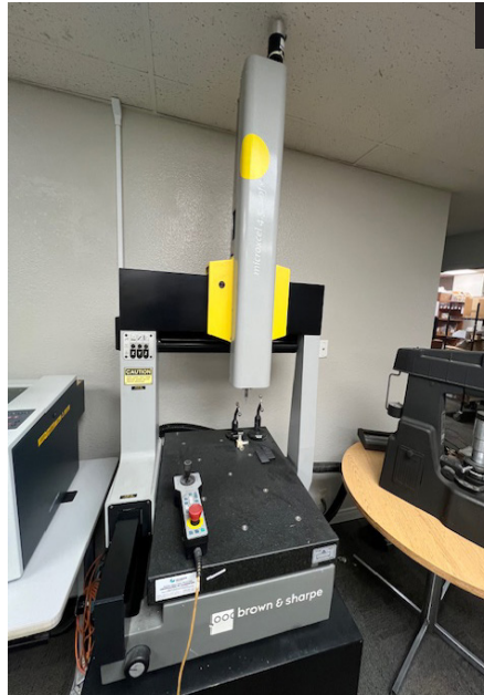
Brown & Sharpe Microxcel 4.5 4 PFX CMM, Manual XYZ, and Renishaw PH9 Probe.
