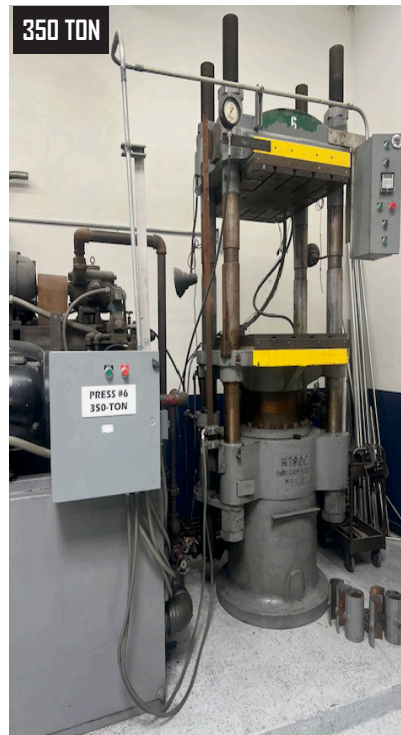
Hysco Hydraulic 4 Post 350 Ton Compression Molding Press.
