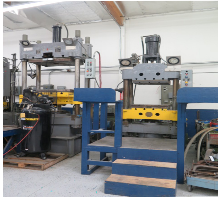
Standard Machinery FJ. Stokes 300 Ton Hydraulic Molding Press and Williams White 100 Ton Hydraulic Molding Press
