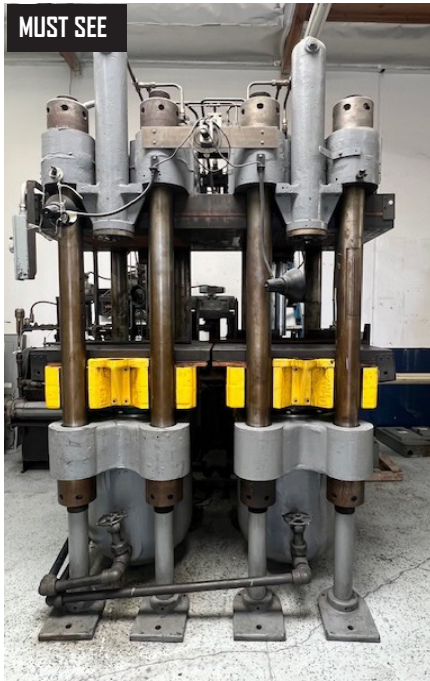
Commercial Iron Works 2) 250 Ton 4 Post Hydraulic Compression Molding Presses w/ 17.75" Piston, 22" Stroke.
