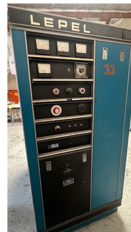
Lepel T-10-3-KC-TL36 Induction Heater.
