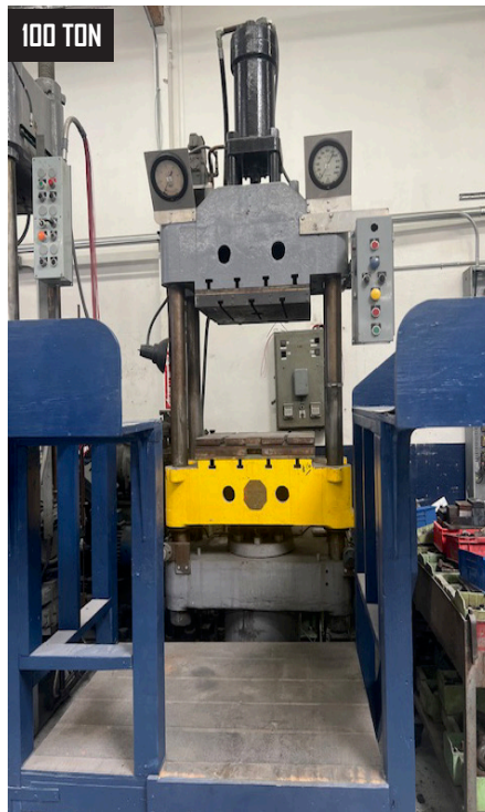
Williams-White & Co Hydraulic 4 Post 100 Ton Compression Molding Press, s/n C-3556.
