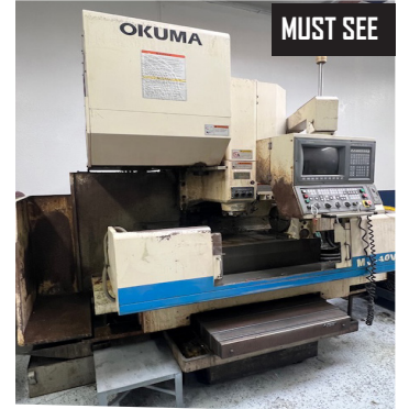
Okuma MC-40VA CNC VMC w/ OSP 7000M Control, 4 th Axis Rotary Table, S/N 0683.
