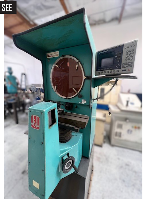
J & L TEC-14, 14" Optical Comparator w/ Quadra Chek 200 Controls.
