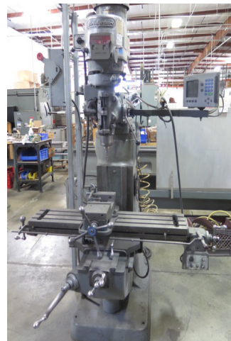
Bridgeport Series 1 - 2Hp Vertical Mill w/ 60-4200 Dial RPM, Power Feed
