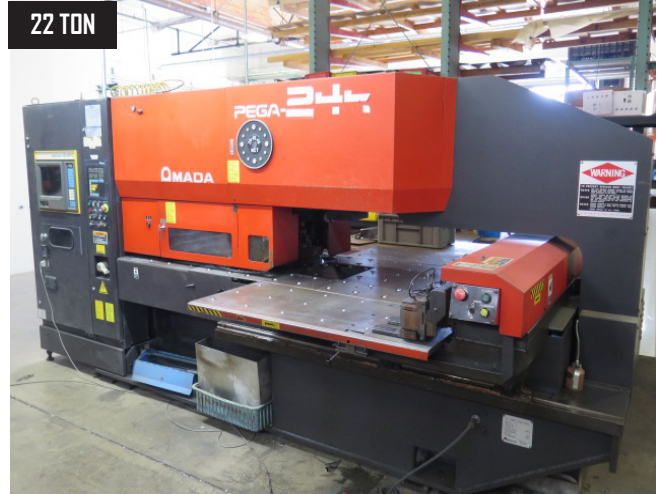
Amada PEGA-244 20 Ton – 24-Station CNC Turret Punch Press w/ Amadan O4P-C Controls
