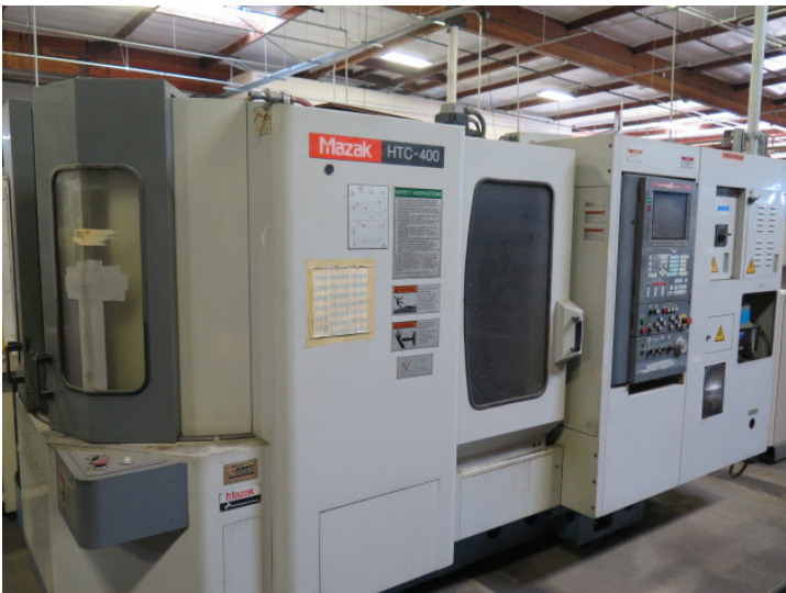
Mazak HTC-400 2-Pallet CNC HMC w/ Mazatrol M-Plus Controls, 30-ATC, CAT-40 Spindle, Tool Presetter, 4th Axis Thru Pallets
