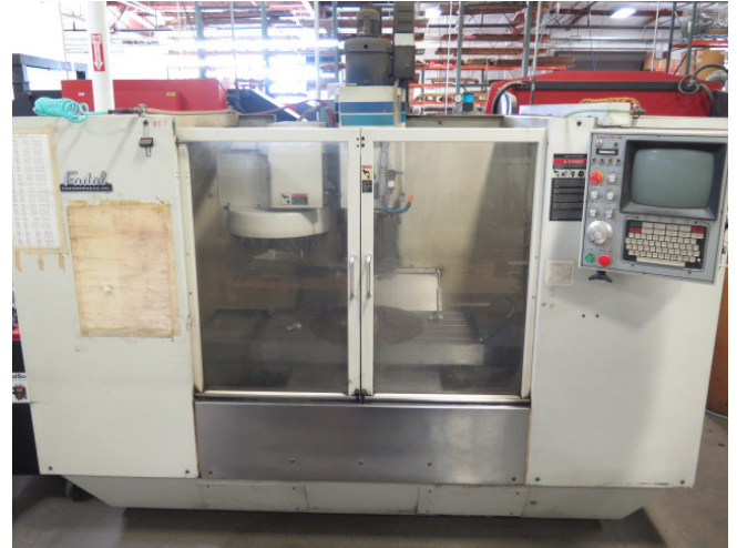
Fadal VMC4020 4-Axis CNC VMC w/ CNC88 Controls, 21-ATC, CAT-40 Spindle, 7500 RPM, Rigid Tapping
