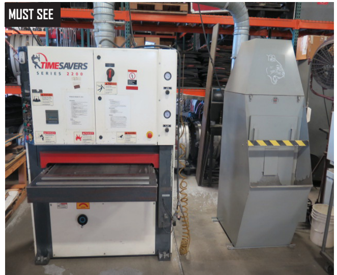
Timesavers 2211-23-0 36" Belt Grainer and CAT C-5 Water-Filtered Dust Collector
