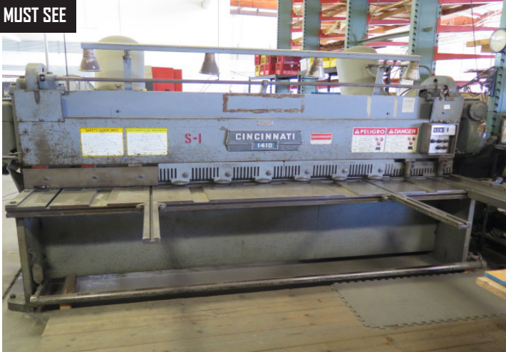
Cincinnati mdl. 1410 3/16" x 10' Power Shear
