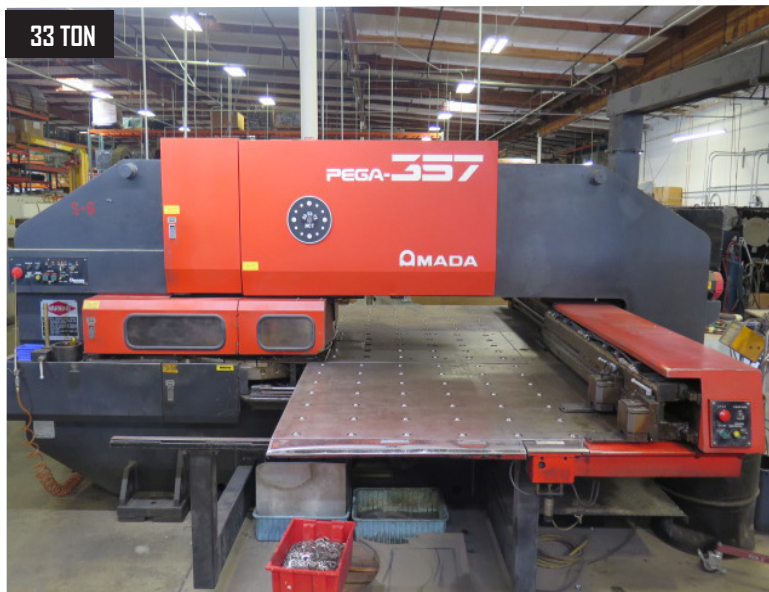
Amada PEGA-357 30 Ton – 58-Station CNC Turret Punch Press w/ Amadan O4P-C Controls
