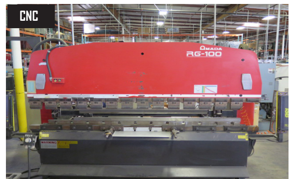
Amada RG-100 100-Ton x 10' CNC Press Brake w/ NC9-EX II Controls
