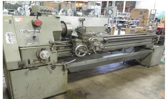
South Bend 17" Turn-Nado 17" x 84" Lathe w/ 30-1580 RPM, Inch Threading, Tailstock, Steady Rest, Trava-Dial, 12" Chuck
