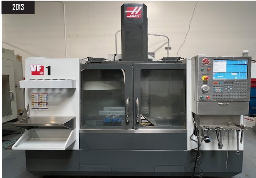
2013 Haas VF-1 CNC Vertical Machining Center s/n 1107168 w/ Has Controls, 20-Station ATC, CAT-40 Taper Spindle, 8100 RPM, Rigid Tapping, Quick Code, Haas Vector Drive, Advanced Tool Management, Coolant.
