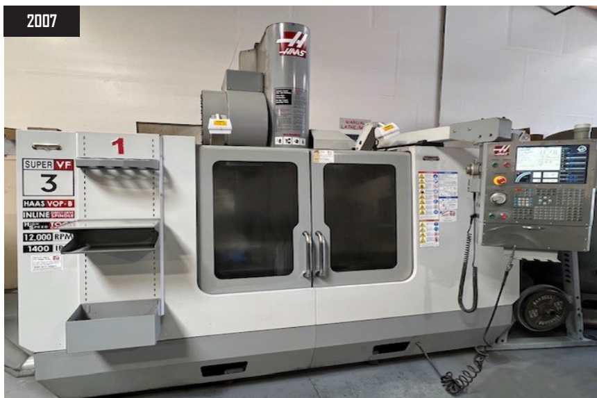
2007 Haas Super VF-3SS 4-Axis CNC Vertical Machining Center s/n 1061846 w/ Haas Controls, Hand Wheel, 24-Station Side-Mount ATC, CAT-40 Taper Spindle, 12,000 RPM, Rigid Tapping, Coord Rotation and Scaling, Macros, Quick Code, High Speed Machining, Advanced Tool Management, Extended Memory, Haas VOP-B, Inline Direct Drive Spindle, High Speed Tool Changer, 1400 IPM, Chip Auger, Coolant.
