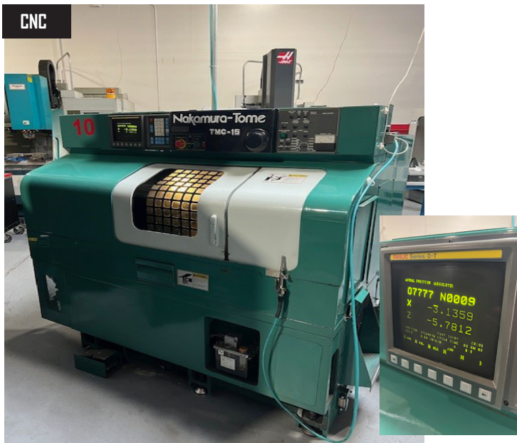
Nakamura-Tome TMC-15 CNC Turning Center s/n E04604 w/ Fanuc Series 0-TControls, 10-Station Turret, 6000 RPM, Coolant.
