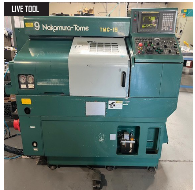
Nakamura-Tome TMC-15M Live Turret CNC Turning Center s/n R12206 w/ Fanuc Series 18-T Controls, 8/16-Station Live Turret, 6000 RPM, Coolant.
