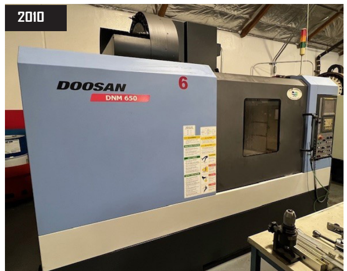
2010 Doosan DNM650 CNC Vertical Machining Center s/n DVM6500133 w/ Doosan-Fanuc I Series Controls, Hand Wheel, 30-Station Side-Mount ATC, CAT-40 TaperSpindle, 12,000 RPM, Thru Spindle Coolant, Kaukin Oil Cooler, Travels X=50", Y=26.3", X=24.6", Chip Auger, Coolant.
