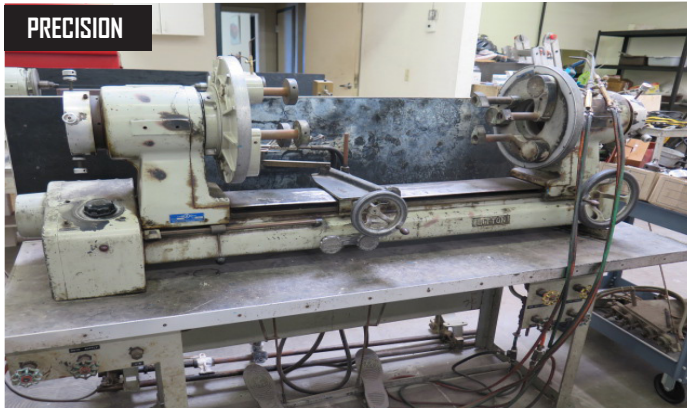
Litton mdl. HSJ 114mm (4 1/2") Glass Lathe w/ Unidrive Variable Speed, 10-240 RPM, 36 1/2" Between Nose and Spindle, Fire Carriage
