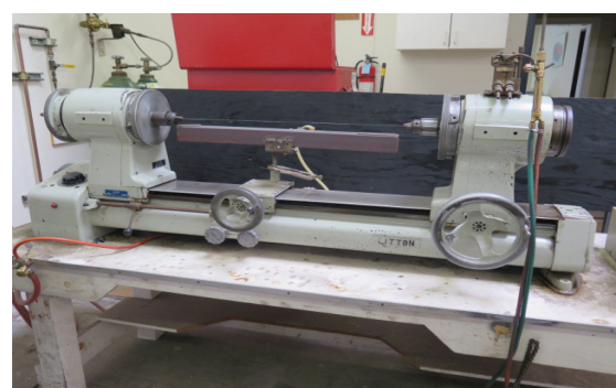
Litton mdl. HSJ 114mm (4 1/2") Glass Lathe w/ Unidrive Variable Speed, 10-240 RPM, 36 1/2" Between Nose and Spindle, Fire Carriage
