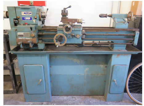
Rutland Type 2649-1190 12" x 36" Lathe w/ 6-Speeds, Inch Threading, Tailstock, Steady Rest, Tool Post, 5C
