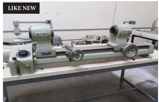
Litton mdl. U 79mm (3 1/8") Glass Lathe w/ Variable Speed, 10-300 RPM, 20 3/4" Between Nose and Spindle, Fire Carriage
