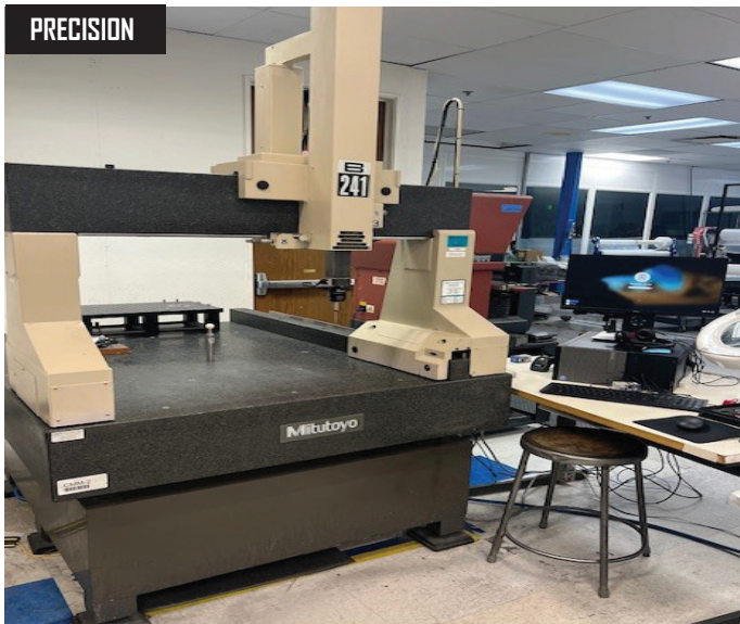
Mitutoyo B241 CMM Machine s/n 8709497 w/ Renishaw MH8 Probe Head, 28" x40" x 18" Work Envelope.
