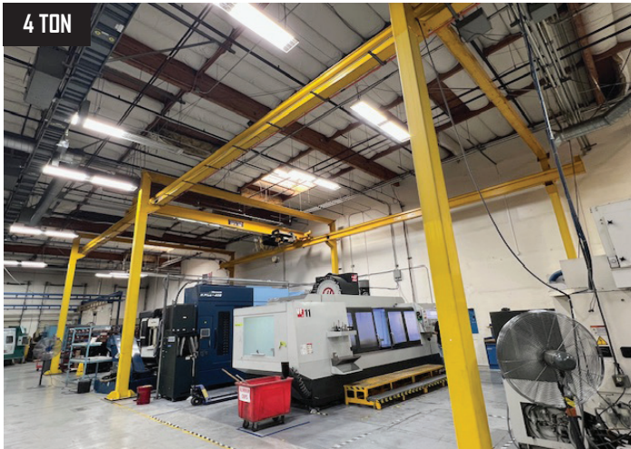
Crane-Veyor 4 Ton Free Standing Overhead Crane System.
