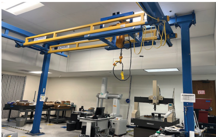
Gorbel 1 Ton Free Standing 4-Post Gantry Crane w/ Coffing Electric Hoist.
