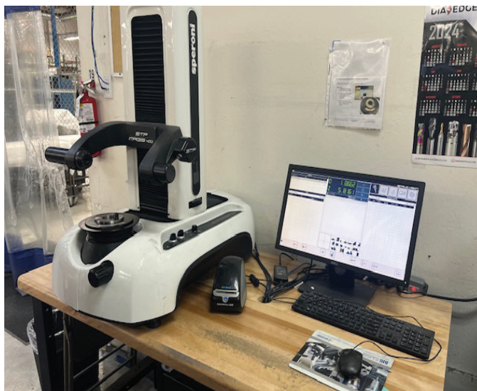
Speroni mdl. 46STP STP Magis 400 Tool Presetter w/ SimpleVision Software, 40-Taper and 50-Taper Adaptors.
