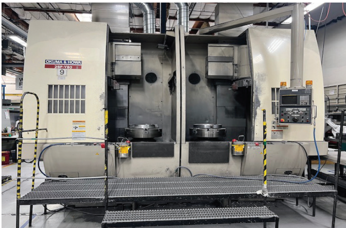
Okuma & Howa 2SP-V80 Twin Spindle, CNC Vertical Lathe s/n 9008 w/ Fanuc Series 18-T Controls, Dual 12-Station Turrets, Dual 24" 3-Jaw Chucks, Chip Conveyors, Coolant.
