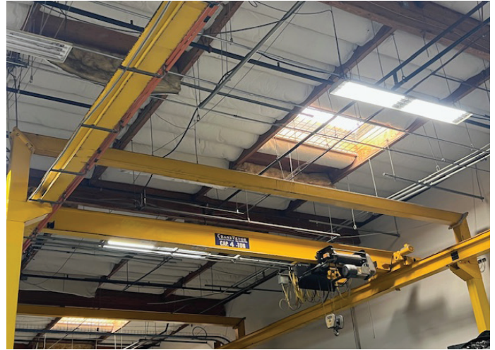
Crane-Veyor 4 Ton Free Standing Overhead Crane System.
