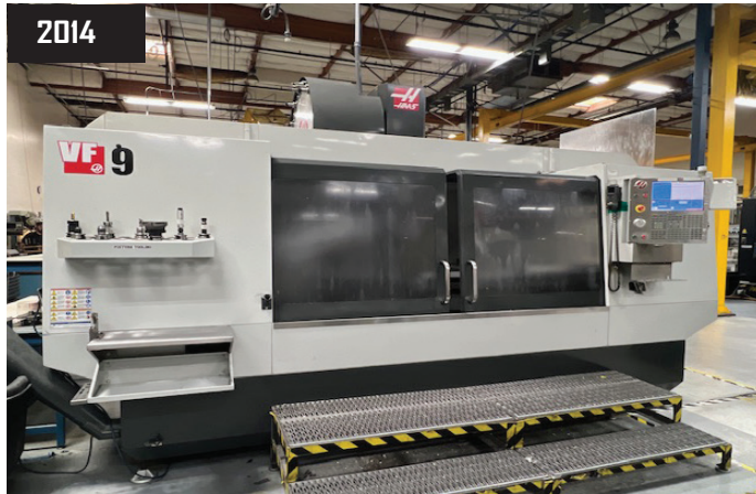
2014 Haas VF-9/40 CNC Vertical Machining Center s/n 118670 w/ Haas Controls, Digital Hand Wheel, 40-Station Side-Mount ATC, BT-40 Taper Spindle, 10,000 RPM, Renishaw Wireless System, Renishaw OTS Tool Touch Probe, Rigid Tapping, Coordinate Rotation and Scaling, M19 Spindle Orientation, Quick Code, Thru Spindle Coolant, Haas Vector Drive, High Speed Machining, Advanced Tool Management, Intuitive Programming System, Programmable Coolant Nozzle, Chip Auger, Coolant.
