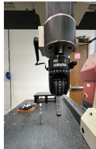
Mitutoyo B241 CMM Machine s/n 8709497 w/ Renishaw MH8 Probe Head, 28" x40" x 18" Work Envelope.
