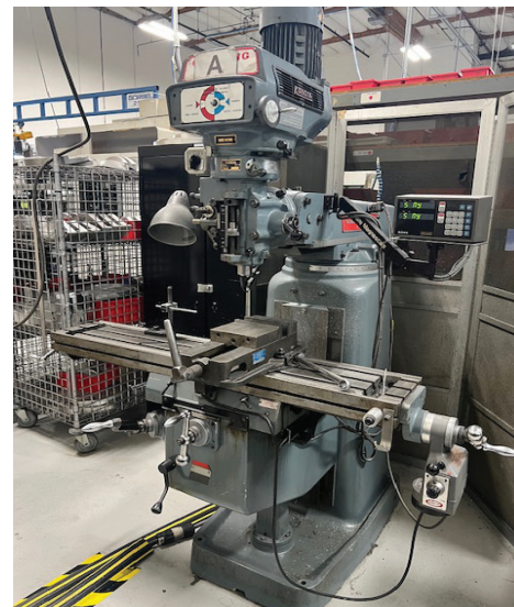
Kondia Vertical Milling Machine, w/ Power Feed and DRO, Variable Speed.
