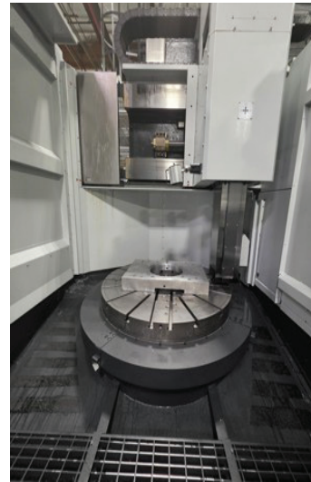
2021 Yama Seiki GV-1200 CNC Vertical Boring Mill w/ 49.1" Chuck, 53.15" Maximum Turning Diameter, Fanuc Oi-TD Control, 25 HP, 50 Taper, 16 Station ATC, s/n 97G044.
