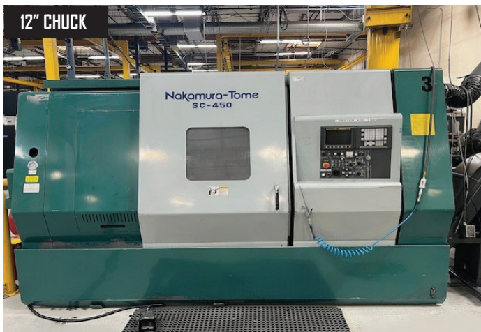
Nakamura-Tome SC-450 CNC Turning Center s/n S450703 w/ Fanuc Series 21-T Controls, 12-Station Turret, Hydraulic Tailstock, 12" 3-Jaw Power Chuck, Chip Conveyor, Coolant.
