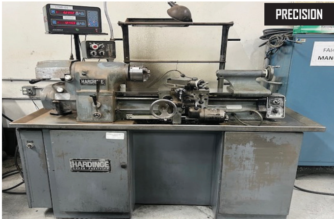
Hardinge HLV-H Wide-Bed Tool Room Lathe s/n HLV-H-12366-T w/Acu-Rite IIIDRO, 120-3000 RPM, Inch Threading, Tailstock, Power Feeds, 6" 3-Jaw and 6" 4-Jaw Chucks.
