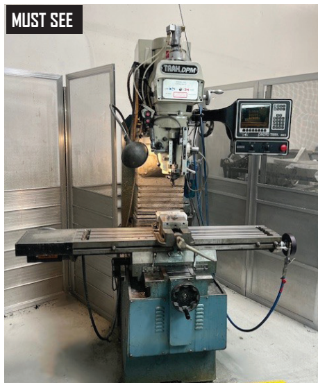
Trak DPM 2-Axis CNC Vertical Mill w/ Proto Trak MX3 Controls, 70-4200 Dial Change RPM, Power Draw-Bar, 40-Taper Spindle, Chrome Box Ways, 10" x 50" Table, Tool Mist.
