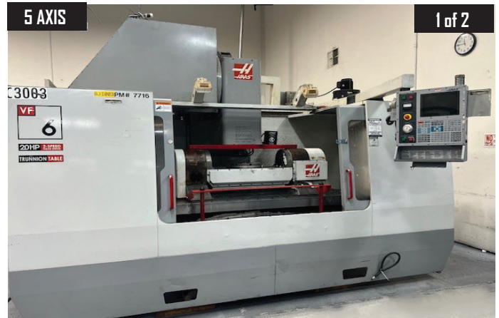
1 of 2 Haas VF-6B/40 TR 5-Axis CNC Vertical Machining Center s/n 27716 w/ Haas Controls, Hand Wheel, Haas 12" Trunnion Table, 24-Station ATC, BT-40 Taper Spindle, 7500 RPM, 20Hp 2-Speed Gear Drive, Rigid Tapping, Programmable Coolant Nozzle, Brushless Servos, 8mb Extended Memory, HSM, Quick Code, Macro Code, Chip Auger, Royal Filtermist Mist Collector, Coolant.
