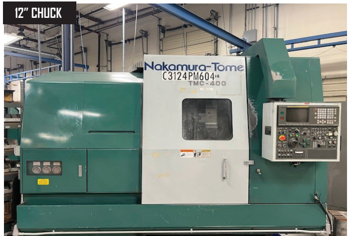
Nakamura-Tome TMC-400 CNC Turning Center s/n C400604 w/ Fanuc Series 16-T Controls, 12-Station Turret, Hydraulic Tailstock, 3" Thru Spindle Bore, Chip Conveyor, 12" 3-Jaw Power Chuck, Coolant.
