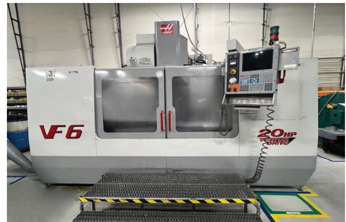
Haas VF-6 4-Axis CNC Vertical Machining Center s/n 24443 w/ Haas Controls, Hand Wheel, 24-Station Side-Mount ATC, BT-40 Taper Spindle, Programmable Coolant Nozzle, Chip Auger, Coolant.
