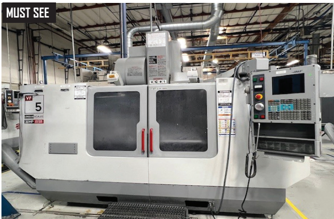
2004 Haas VF-5D/40 CNC Vertical Machining Center s/n 34682 w/ Haas Controls, Hand Wheel, 24-Station Side Mount ATC, BT-40 Taper Spindle, Renishaw Wireless System, Renishaw OTS Tool Touch Probe, 7500 RPM, Rigid Tapping, Coordinate Rotation and Scaling, M19 Spindle Orientation, Macros, Quick Code, Haas Vector Drive, Haas RKH, Chip Auger, Coolant.
