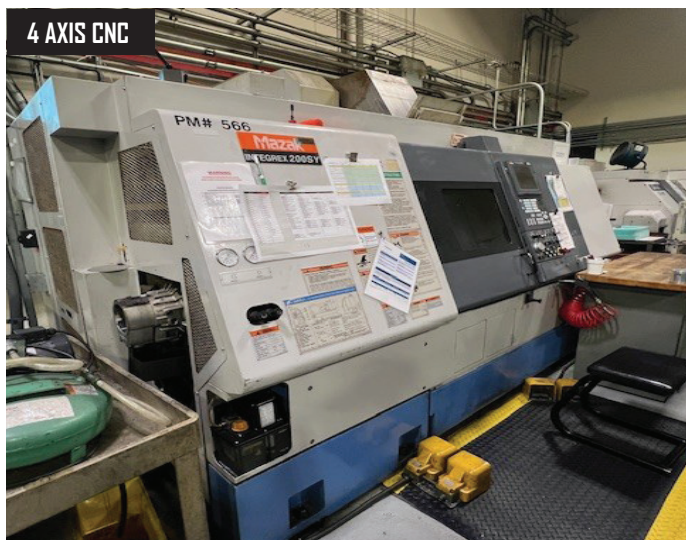
1999 Mazak Inregrex 200SY Twin Spindle "Y" Axis CNC Turning Center s/n 144566 w/ Mazatrol PC Fusion 640MT Controls, Tool Presetter, 8" 3-Jaw Power Chucks on Main and Sub Spindles @ 5000 RPM, Full "C" Axis @ 0.001 Deg, "Y" Axis with 40-Station ATC, HSK Tool Spindle @ 6000 RPM, Coolant.
