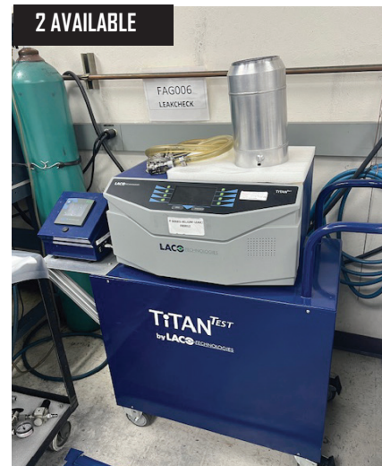
(2) Laco TiTAN-Test P-Series Helium Leak detectors w/ TCM Digital Controllers.
