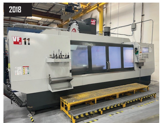
2018 Haas VF-11/40 4-Axis CNC Vertical Machining Center s/n 1148361 w/ Haas Controls, Digital Hand Wheel, 40-Syation ATC, BT-40 Taper Spindle, 15,000 RPM, Renishaw Wireless System, Programmable Coolant Nozzle, M19 Spindle Orientation, High Speed Machining, VPS Editing, 1GB Memory Expansion, Compensation Tables, Thru Spindle Coolant, Royal Filtermist Mist Collector, Coolant, 6637 RUN Hours.
