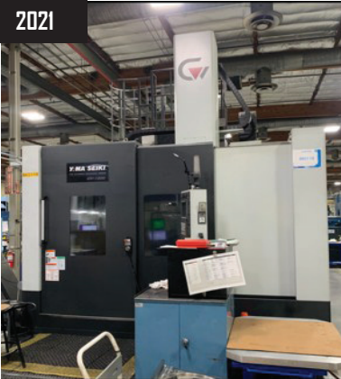
2021 Yama Seiki GV-1200 CNC Vertical Boring Mill w/ 49.1" Chuck.
