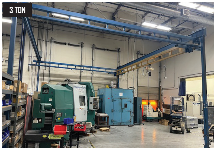
Gorbel Free Standing 4-Post Gantry Crane w/ Harrington Electric Hoist.
