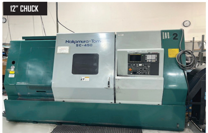
Nakamura-Tome SC-450 CNC Turning Center s/n S450804 w/ Nakamura-Tome Fanuc Controls, 12-Station Turret, Hydraulic Tailstock, 3 1/8" Thru Spindle Bore, 12" 3-Jaw Power Chuck, Chip Conveyor, Coolant.
