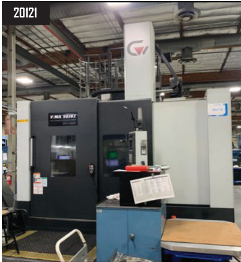
2021 Yama Seiki GV-1200 CNC Vertical Boring Mill w/ 49.1" Chuck, 53.15" Maximum Turning Diameter, Fanuc Oi-TD Control, 25 HP, 50 Taper, 16 Station ATC, s/n 97G044.
