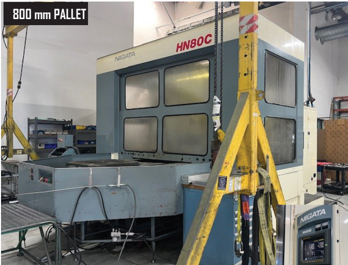
Nigata HN80C 2-Pallet CNC Horizontal Machining Center w/ Fanuc Series 15-MG/S Controls, Hand Wheel, 160-Station ATC, CAT-50 Taper Spindle, 4th Axis Thru Pallets, (2) 31 1/2" x 31 1/2" Pallets, Thru Spindle Coolant, Daikin Oil Cooler, Chip Augers, Chip Conveyor, Coolant.
