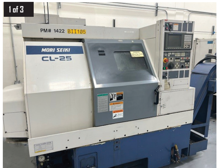
1997 Mori Seiki CL-25A CNC Turning Center s/n 1456 w/ Mori Seiki MSC-521 Controls, Tool Presetter, 10-Station Turret, 12" 3-Jaw Power Chuck, Chip Conveyor, Coolant.
