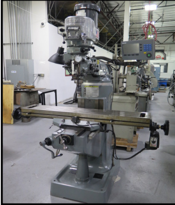
Bridgeport Vertical Mill s/n HDNG8025M w/ Acu-Rite Programmable DRO, 60-4200 Dial-Change RPM, Chrome Ways, Power Feed, 9" x 49" Table.
