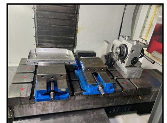
2015 Haas VM-2 CNC Vertical Machining Center, s/n 1119634, w/ Haas Controls, 24-Station Side Mount ATC, 40 Taper, Renishaw Probe System w/ Touch Probe, Royal Filtermist, 12,000 RPM Spindle, Mold Makers Option.
