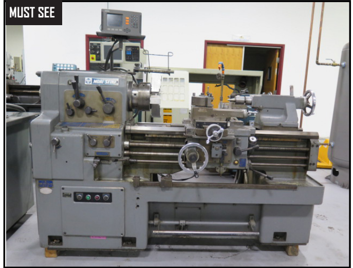
Mori Seiki MS-850G 17" x 36" Geared Head Gap Bed Lathe s/n 17393 w/ Heidenhain DRO, 32-1800 RPM, Inch Threading, Tailstock, Tool Post, 5C Collet Closer, 8" 3-Jaw Chuck, Coolant.
