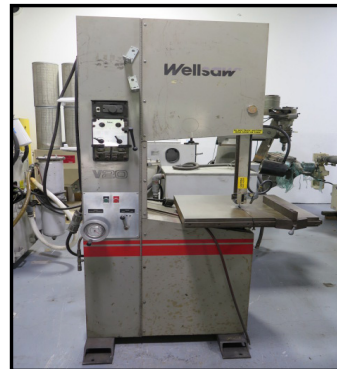
Wellsaw V20 20" Vertical Band Saw w/ Dial Speed Change, Blade Welder, 26" x 26" Table, Fence.
