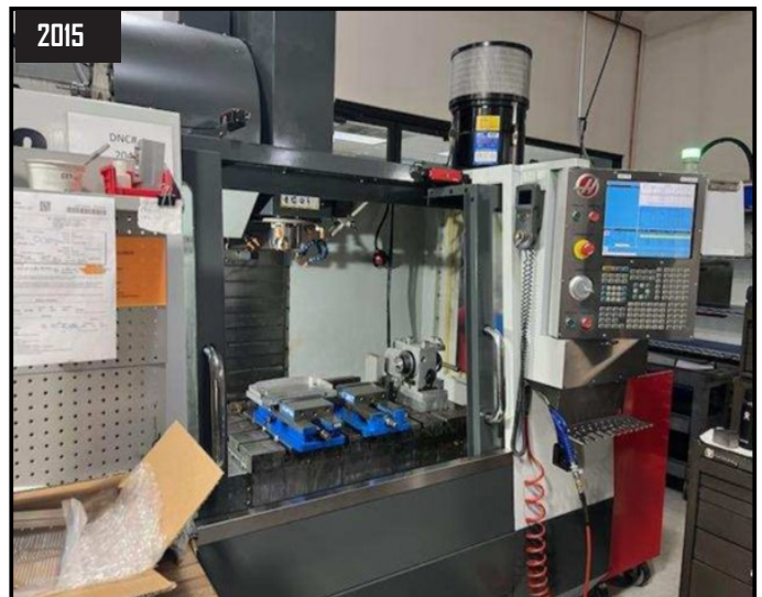
2015 Haas VM-2 CNC Vertical Machining Center, s/n 1119634, w/ Haas Controls, 24-Station Side Mount ATC, 40 Taper, Renishaw Probe System w/ Touch Probe, Royal Filtermist, 12,000 RPM Spindle, Mold Makers Option.
