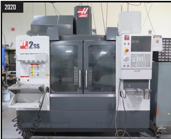
2020 Haas VF-2SS 4-Axis CNC Vertical Machining Center s/n 1172404 w/ Haas Controls, 30-Station Side-Mount ATC, HSK63A Taper Spindle, Renishaw Wireless System, Renishaw OTS Tool Touch Probe, Programmable Coolant Nozzle, Chip Auger, Coolant.
