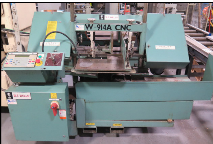
W.F. Wells W914ACNC 9" CNC Horizontal Band Saw s/n A3330WA08112 w/ Wells CNC Controls, Pneumatic Clamping and Feed, Coolant.
