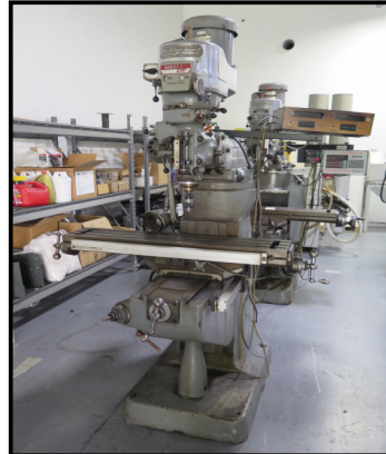
Bridgeport Series 1 - 2Hp Vertical Mill s/n 195368 w/ Pos-Econ DRO, 60-4200 Dial-Change RPM, Chrome Ways, 9" x 42" Table.
