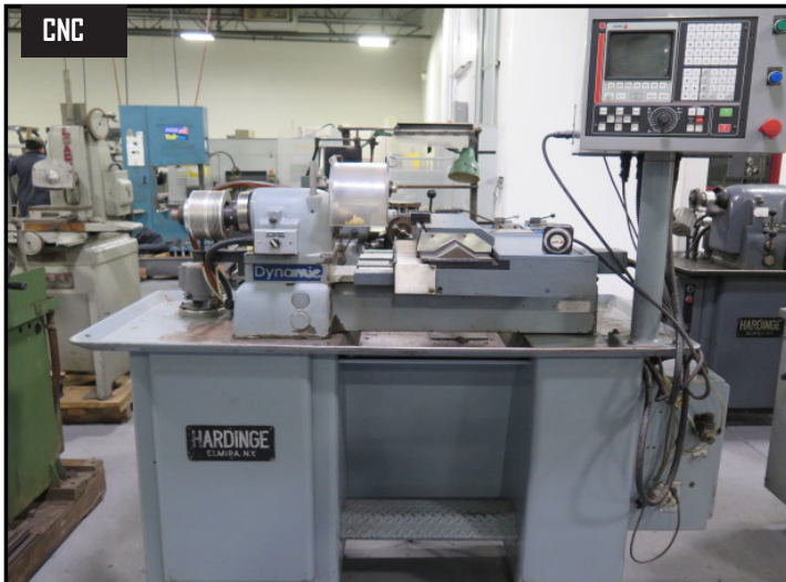
Hardinge / Dynamic CNC Cross Slide Lathe w/ Fagor CNC Controls, Pneumatic 5C Collet Closer, 2 1/2" x 20" Cross-Slide Table, Coolant.
