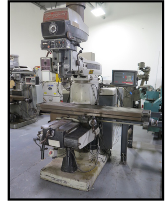
Bridgeport Series II Vertical Mill s/n 6190 w/ Newall DP7 Programmable DRO, 50-3500 Dial-Change RPM, 40-Taper Spindle, Chrome Box Ways, Power Quill Feed, 11" x 58" Table.
