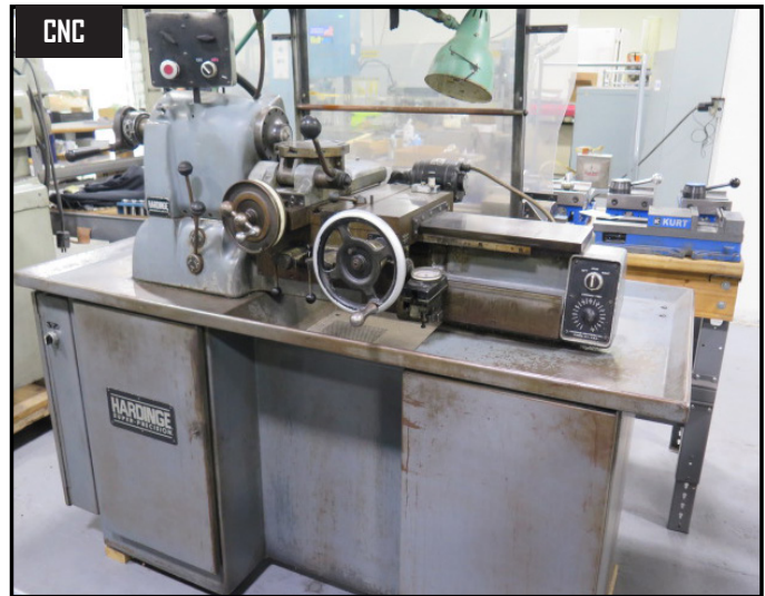
Hardinge TFB-H Wide-Bed Second OP Lathe s/n HLV-H-3222 w/ 125-3000 RPM, Tailstock, Power Feeds, 5C Collet Closer, Coolant.
