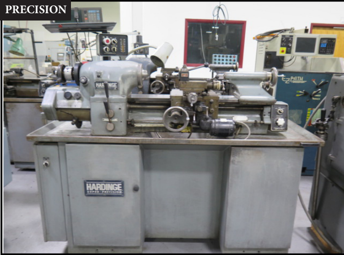
Hardinge HC Hand Chucker s/n HC-8242-T w/ 125-3000 RPM, 8-Station Turret, Power Feeds, Trava-Dial, 5C Collet Closer, Coolant.
