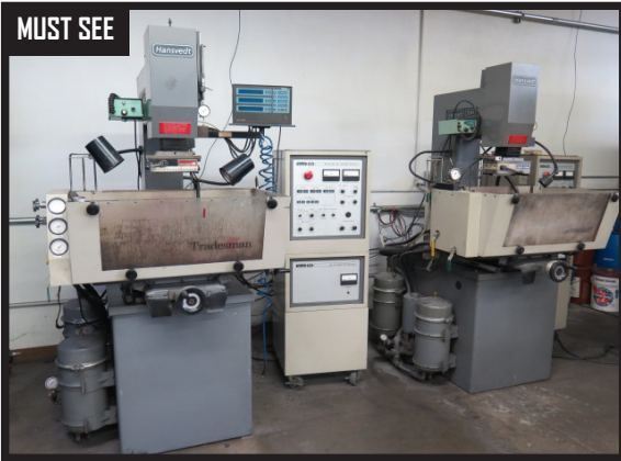
Hansvedt "Tradesman" Die Sinker EDM Machine w/ H-Pulse 201 Power Source, SM-155 Booster Module, Acu-Rite "Qwikcount" DRO, 12" x 20" Table, Walker 6" x 12" Magnetic Chucks (ON TABLE AND RAM), Coolant System.
