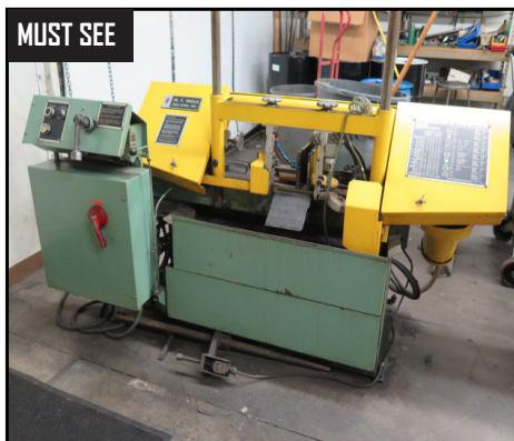
W.F. Wells 9" Horizontal Band Saw w/ Manual Clamping, Coolant.
