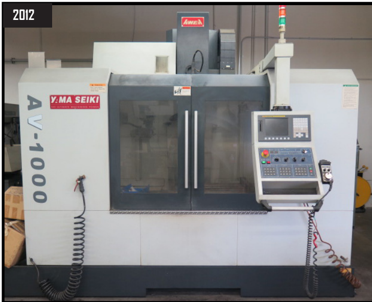
2012 Yama-Seiki Awea AV-1000 CNC Vertical Machining Center s/n 1000-12021 w/ Fanuc Series 0i-MB Controls, Hand Wheel, 24-Station ATC, CAT-40 Taper Spindle, Renishaw Wireless System, Renishaw OTS Tool Touch Probe, Renishaw CAT-40 Taper Probe Head, 10,000 RPM, Chip Augers, Coolant.
