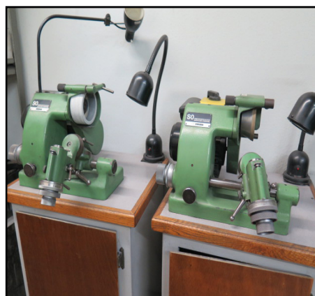
Deckel SO Single-Lip Tool Grinder s/n 98-26449 w/ Collet Set and Cabinet.
