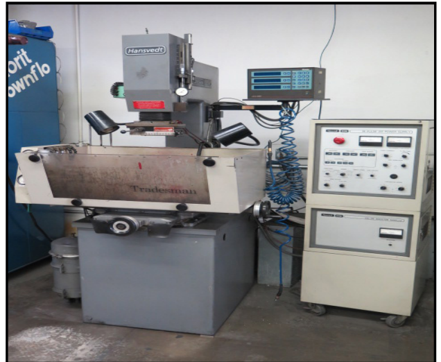
Hansvedt "Tradesman" Die Sinker EDM Machine w/ H-Pulse 201 Power Source, SM-155 Booster Module, Acu-Rite "Master" 3-Axis Programmable DRO, 12" x 20" Table, Walker 10" x 15" Magnetic Chuck, Ceramax 4" x 8" Magnetic Chuck (ON RAM), Coolant System.
