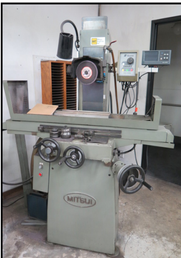
2000 MHT Mitsui High-Tec MSG-205MH 6" x 18" Surface Grinder s/n 2001063538 w/ Acu-Rite "Qwikcount" DRO, 6" x 18" Electromagnetic Chuck, Coolant.
