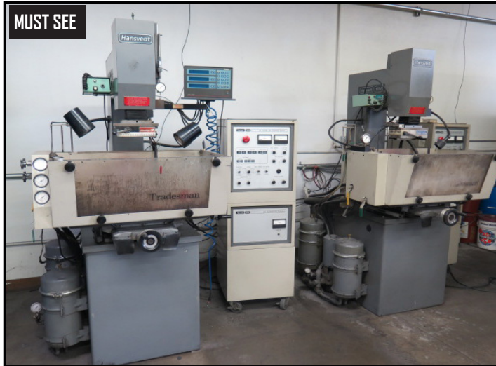
Hansvedt "Tradesman" Die Sinker DM Machine w/ H-Pulse 201 Power Source, SM-155 Booster Module, Acu-Rite "Qwikcount" DRO, 12" x 20" Table, Walker 6" x 12" Magnetic Chucks (ON TABLE AND RAM), Coolant System.
