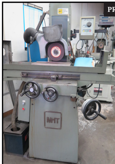
MHT Mitsui High-Tec MSG-205MH 6" x 18" Surface Grinder s/n 97043294 w/ Acu-Rite "Qwikcount" DRO, 6" x 18" Electromagnetic Chuck, Coolant.
