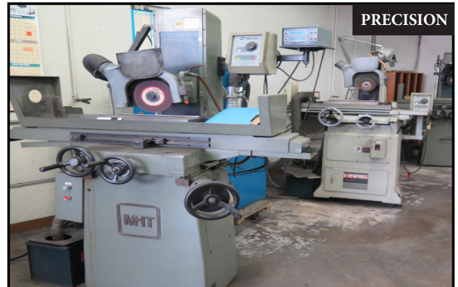
2000 MHT Mitsui High-Tec MSG-205MH 6" x 18" Surface Grinder s/n 2001063538 w/ Acu-Rite "Qwikcount" DRO, 6" x 18" Electromagnetic Chuck, Coolant.
