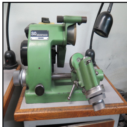
Deckel SO Single-Lip Tool Grinder s/n 98-26449 w/ Collet Set and Cabinet.
