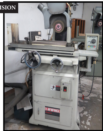
Harig 618 Ballway 6" x 18" Surface Grinder w/ 6" x 18" Magnetic Chuck.
