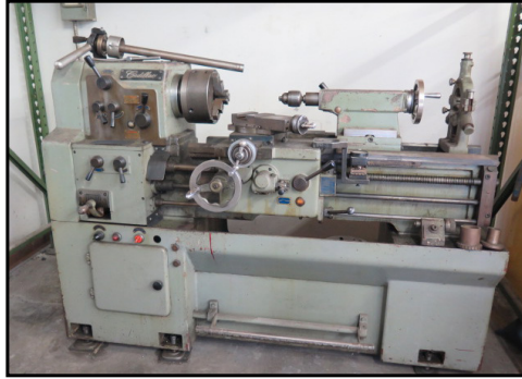
Cadillac 1428G 14" x 28" Gap Bed Lathe s/n 059371 w/ 83-1800 RPM, Inch Threading, Tailstock, Trava-Dial, Nix Tool Post, 5C Collet Closer, 8" 3-Jaw Chuck.
