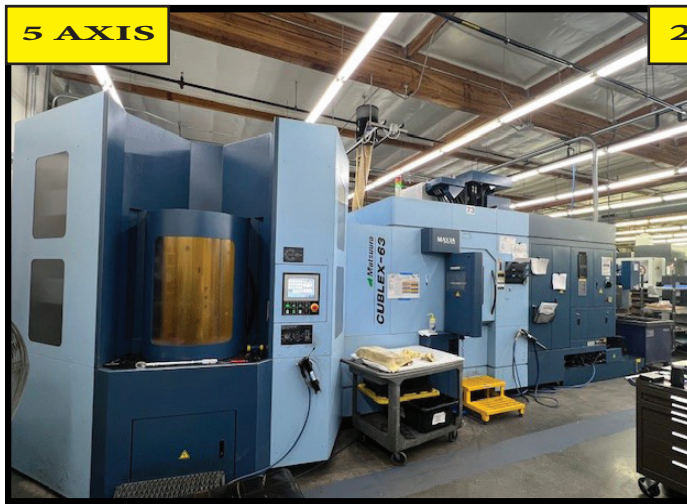
2015 MATSUURA CUBLEX 63V 5- axis vertical machining center, 240-tool ATC, 12,000RPM spindle, Matsuura G-TECH 30i Controls, HSK-A63 and w/ 16 Automatic Pallet Changer.
