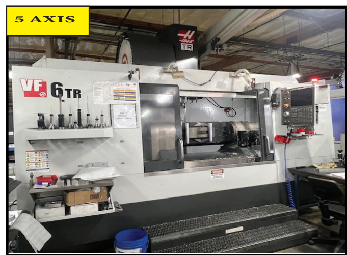
2012 Haas VF-6/40TR 5-Axis Vertical Machining Center, 64"x 32" x 30" (1626 x 813 x 762 mm), with integrated 12.2 (310 mm) 2-axis trunnion rotary table, 40 taper, 30 hp (22.4 kW) vector drive, 8100 rpm, inline direct-drive.
