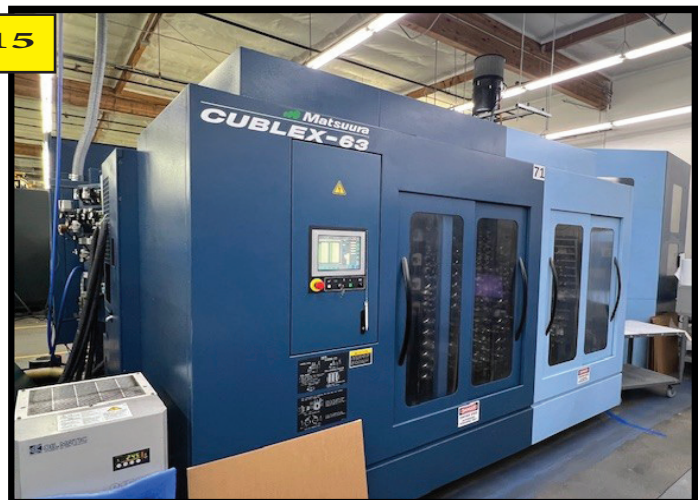
2015 MATSUURA CUBLEX-63V, 5-Axis Vertical Machining Center, 12,000 RPM spindle, 240-tool ATC, High-Pressure Coolant, Matsuura PC-18 Tower Pallet System.
