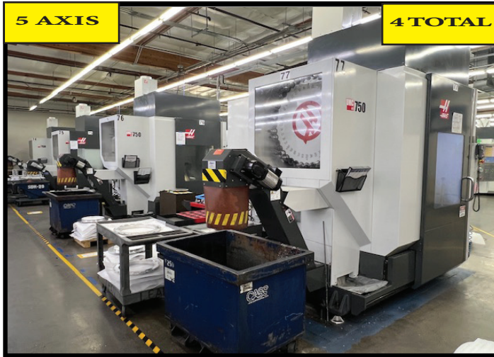
4 TOTAL) 2014 HAAS UMC-750, used vertical machining center, features X/Y/Z travels: 30/20/20 spindle speed: 12,000 RPM, 41-tool capacity, 30 hp motor, CAT 40 taper, 300 psi coolant. Includes HAAS CNC, probing systems.
