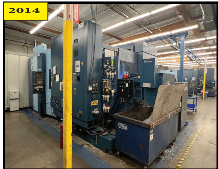
2014 MATSUURA H-PLUS 630, 4-Axis Horizontal Machining Center, 120-tool ATC, Dual Pallets (24.8"x24.8" FANUC 30i Control, W/ FASTEMS AUTO PALLET SYSTEM.
