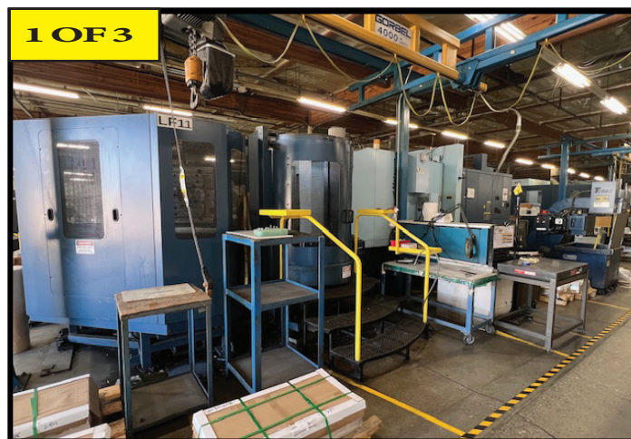
1 OF 3) MATSUURA H-PLUS 630, 4-Axis Horizontal Machining Center, Cat 50 Taper, PC- 6 Multi Pallet System, (24.8"x 24.8") Pallets, Matsuura Fanuc G-Tech 30i Control, Chip Conveyor.
