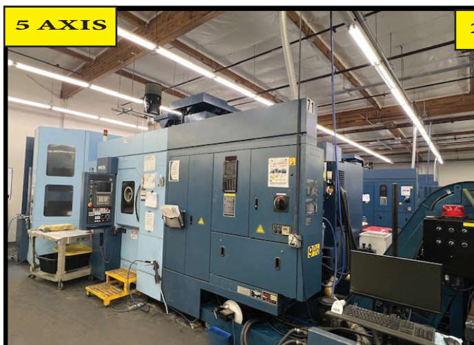
2015 MATSUURA CUBLEX-63V, 5-Axis Vertical Machining Center, 12,000 RPM spindle, 240-tool ATC, High-Pressure Coolant, Matsuura PC-18 Tower Pallet System.
