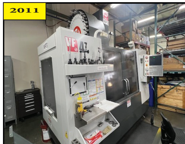
2011 HAAS VF-4D, used vertical machining center, featuring 50"x 20"x 25" in travel, 40-tool capacity, 10,000 RPM spindle, HAAS CNC control, wireless probing.
