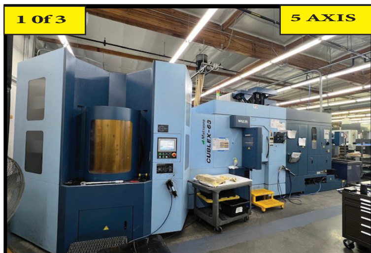
2015 MATSUURA CUBLEX 63V 5- axis vertical machining center, 240-tool ATC, 12,000RPM spindle, Matsuura G-TECH 30i Controls, HSK-A63 and w/ 16 Automatic Pallet Changer.
