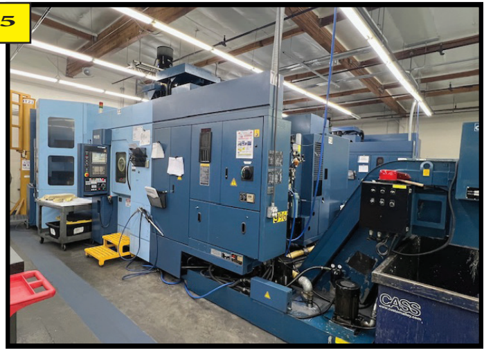
2015 MATSUURA CUBLEX 63V 5- Axis vertical machining center, 240-tool ATC, 12,000RPM spindle, Matsuura G-TECH 30i Controls, HSK-A63 and w/ 16 Automatic Pallet Changer.
