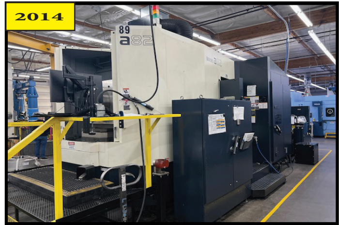
2) 2014 MAKINO A82 Horizontal Machining Center, featuring X-Y-Z travel of 43.3" X 32.3" X 40.1 CAT 50 spindle taper, 47 hp, 20,000 RPM, 241-tool ATC, 4-axis, hi-pressure coolant. Includes MAKINO Pro 5 Control, tool perester, part probe.
