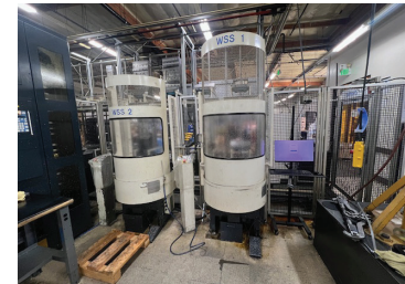
Makino A66E Horizontal Machining Center Cell System, 4 Axis, 20,000 RPM, Cat 50 Taper, 28.7" x 28.7" x 31.4" (XYZ Travel), Cell System.
