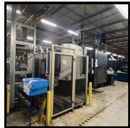
Makino 2 Machine Cell System w/ A61 Horizontal Machining Centers, 4 Axis, 20,000 RPM, Cat 50 Taper, 19.7" x 19.7" Pallets, 28.7" x 25.6" x 28.7" (XYZ Travels), Tower Style Auto Pallet System.
