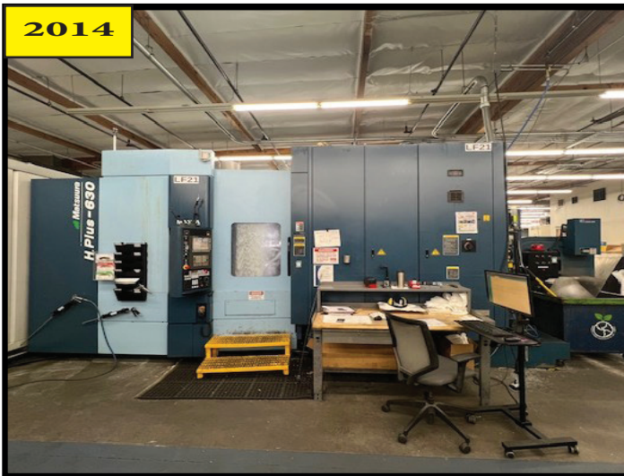
2014 MATSUURA H.PLUS-630, Horizontal Machining Center with 41.33 x, 36.2 38.97 z travels, CAT 50 spindle, 12,000 RPM, 4-axis, 120 tool ATC, dual 24.8 x pallets. Equipped with FANUC 30i.
