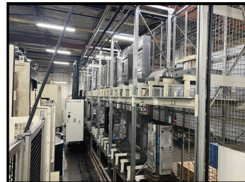
Makino A66E Horizontal Machining Center Cell System, 4 Axis, 20,000 RPM, Cat 50 Taper, 28.7" x 28.7" x 31.4" (XYZ Travel), Cell System.
