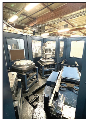
1 OF 3) MATSUURA H-PLUS 630, 4-Axis Horizontal Machining Center, Cat 50 Taper, PC- 6 Multi Pallet System, (24.8"x 24.8") Pallets, Matsuura Fanuc G-Tech 30i Control, Chip Conveyor.
