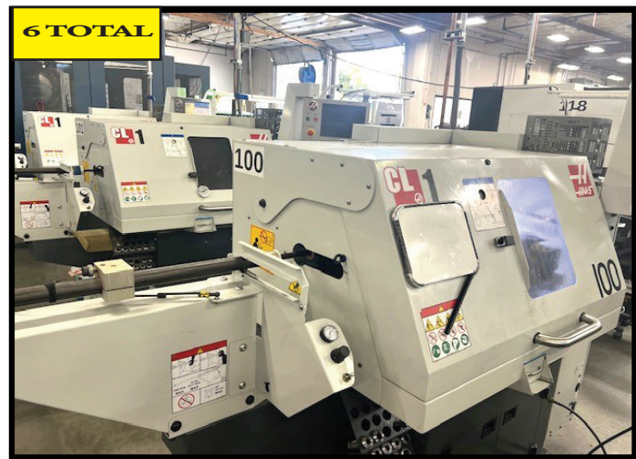
6 TOTAL) 2018 HAAS CL-1 CNC Lathe, must move! Features 11" swing, 4 chuck, 5 HP spindle up to 8,000 RPM, 12 5Axis travel, 8" Z-axis travel, and 2 axis. Equipped with HAAS CNC control, 8-station turret, gang-style tooling kit.
