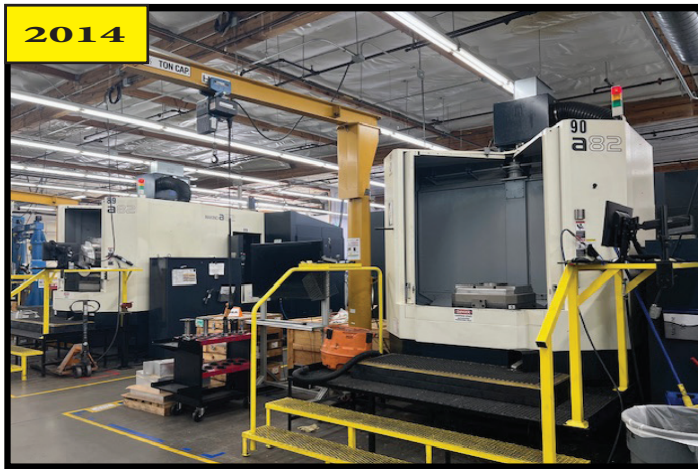
2) 2014 MAKINO A82 Horizontal Machining Center, featuring X-Y-Z travel of 43.3" X 32.3" X 40.1 CAT 50 spindle taper, 47 hp, 20,000 RPM, 241-tool ATC, 4-axis, hi-pressure coolant. Includes MAKINO Pro 5 Control, tool perester, part probe.
