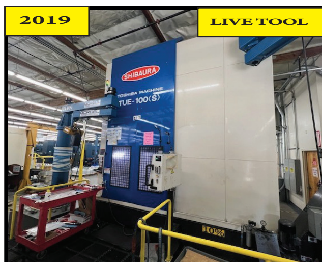
2019 TOSHIBA TUE 100S Boring Mill, Features a 40” table, Live Spindle, AC motors (60/50 HP, 25/20 HP), 15-3,000 RPM spindle speed, and FANUC Oi-TF. Includes tool perester, probe, and chip conveyor, 7752 cut Hours.
