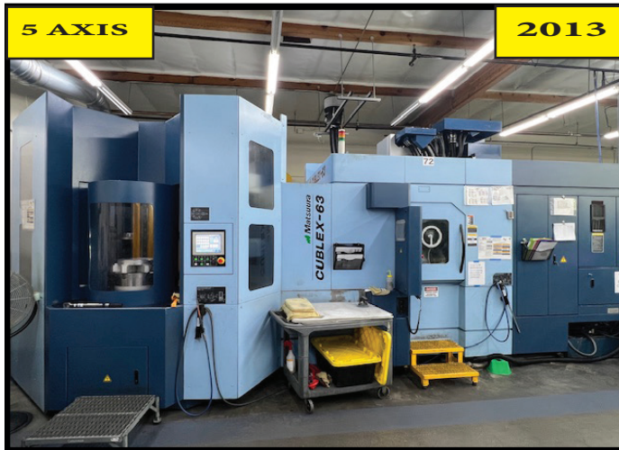
2013 MATSUURA CUBLEX-63V 5-Axis Vertical Machining Center w/ 29.92"Y x 33.267" Y 25.98" Z travel, 12,000 RPM, 320-tool ATC, and HSK-63 spindle, high-pressure coolant, and 18-Auto Pallet System, MATSUURA G-TECH 30i Control, Tail Stock.
