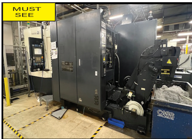
Makino 2 Machine Cell System w/ A61 Horizontal Machining Centers, 4 Axis, 20,000 RPM, Cat 50 Taper, 19.7" x 19.7" Pallets, 28.7" x 25.6" x 28.7" (XYZ Travels), Tower Style Auto Pallet System.
