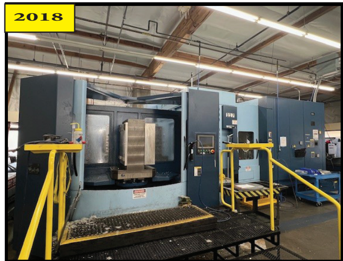
2018 MATSUURA H-PLUS-630 - PC-6, Horizontal Machining Center, 4-axis, CAT 50 taper, 12,000 RPM, 40 hp, 245 tools, 6 pallets, chip conveyor, G-TECH 31i control.
