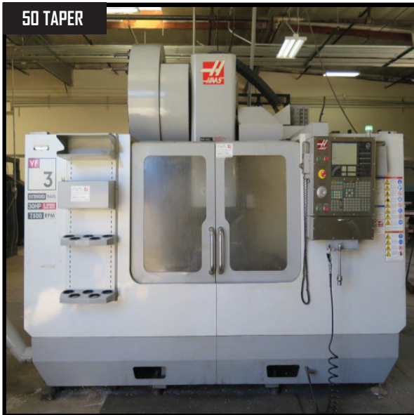
50 TAPER 12/2007 Haas VF-3YT/50 CNC Vertical Machining Center s/n 1062967 w/ Haas Controls, Digital Hand Wheel, 30-Station ATC, CAT-50 Taper Spindle, 7500 RPM, RigidTapping, Extended Travel, 30Hp 2-Speed Gear Drive, Quick Code, Haas Vector Drive, Advanced Tool Management, Programmable Coolant Nozzle, Coolant.
