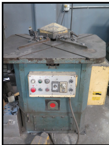
Amada CS-220 10-Ton 8 5/8" x 8 5/8" Hydraulic Corner Notcher s/n 543414.
