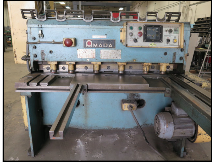
Amada M-1232 1/8" x 48" Power Shear s/n 1230928 w/ Amada Controls and Back Gauging, 75 Strokes/Min, 44" Squaring Arm, Front Support.
