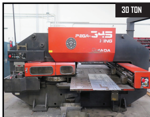
30 TON 1990 Amada PEGA-345 KING PEGA304050 30- Ton 58-Station CNC Pneumatic Turret Punch Press s/n AK450214 w/ Amadan 04P-C Controls, 58-Station Turret, (2) Indexable Stations, Sheet Repositioner, Ball- Top Table.
