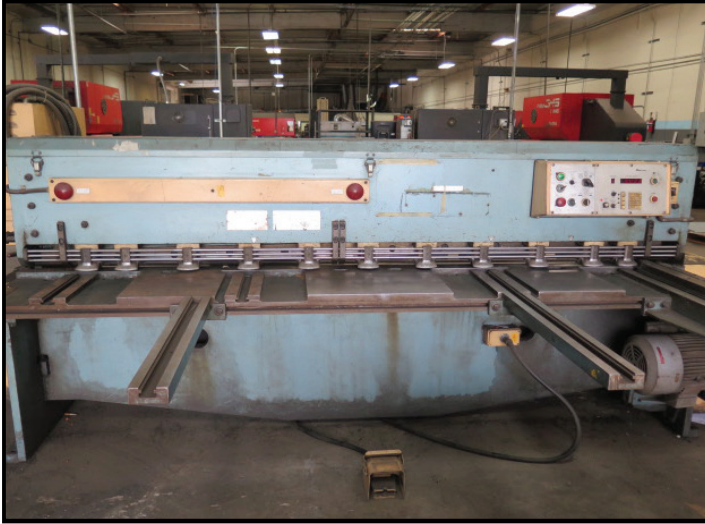
Amada M-2545 3/16" x 98" Power Shear s/n 2502471 w/ Amada Controls and Back Gauging, 60 Strokes/Min, 100" Squaring Arm, Front Supports,
