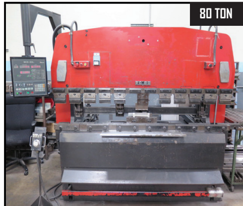
80 TON Amada RG-80 80-Ton x 94" CNC Press Brake s/m 808866 w/ Maada NC9-EX II Controls, 3.94" Stroke, 16" Throat
