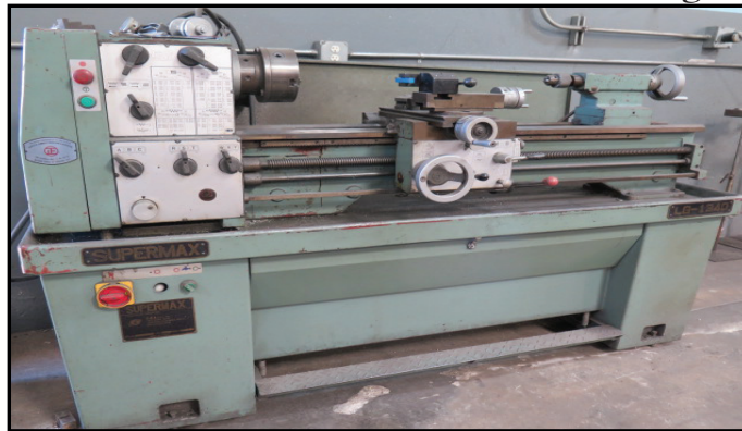
Supermax LG-1340 13" x 40" Geared Head Lathe w/ 40-2500 RPM, Inch/mm Threading, Tailstock, KDK Tool Post, 6" 3-Jaw chuck.
