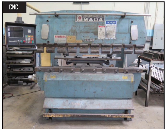
Amada RG-50 50-Ton x 78" CNC Press Brake (NEEDS WORK) w/ Hurco Auto-bend 5C Controls, 82.1" Max Bend Length, 59.9" Between Uprights, 15.76" Throat, 3.94" Stroke, 13.79" Open Height
