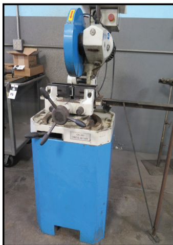
KBC CS-350 Miter Cold Saw w/ 2-Speeds, Speed lamping, Coolant.
