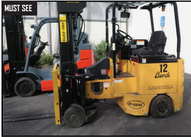
Landoll Bendi B30/42E 180D 3000 Pb Cap Articulating Electric Forklift
