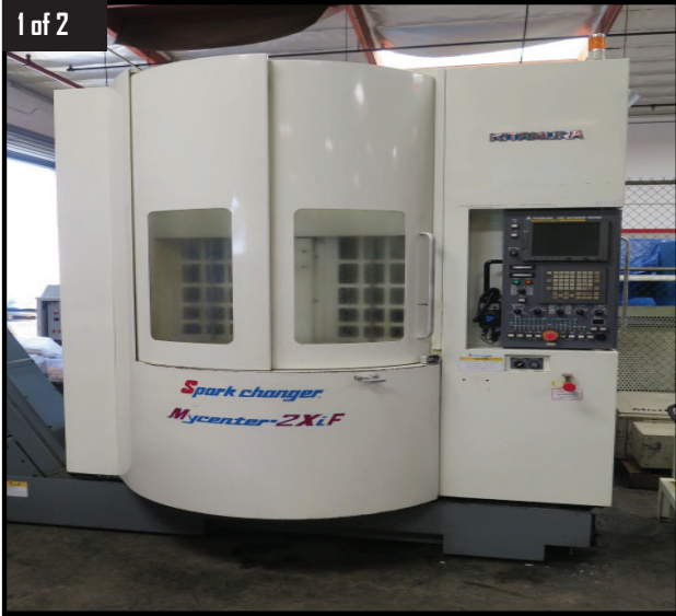
Kitamura Spark Changer Mycenter-2XiF 2-Pallet CNC VMC w/ Fanuc 16i-MB Controls, 24-ATC, CAT-40, 20,000 RPM, Renishaw TRS2 Wireless System, Broken Tool Detection, Fire Suppression **2-AVAILABLE**
