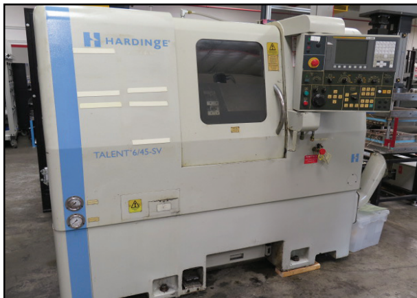
Hardinge Talent 6/45-SV CNC Turning Center w/ Hardinge/ Fanuc SV Controls, 12-Station Turret, Renishaw Wireless System, Renishaw Touch Probe
