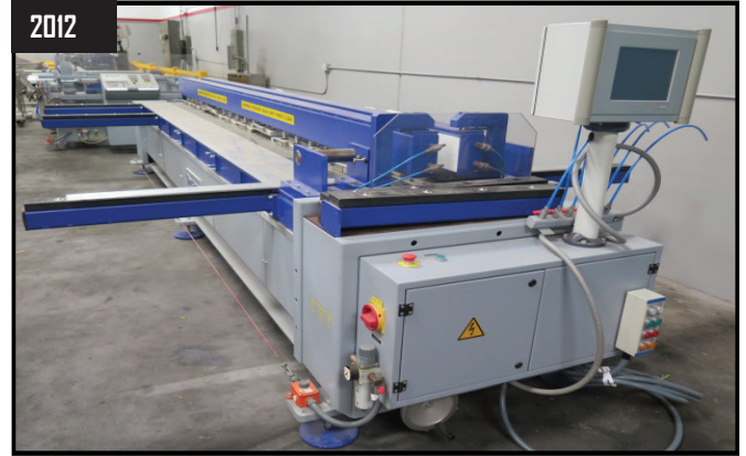
2012 Wegener SM440TPQ Plastics Sheet Butt Welder w/ Sutron TP31 Touch Screen Controls
