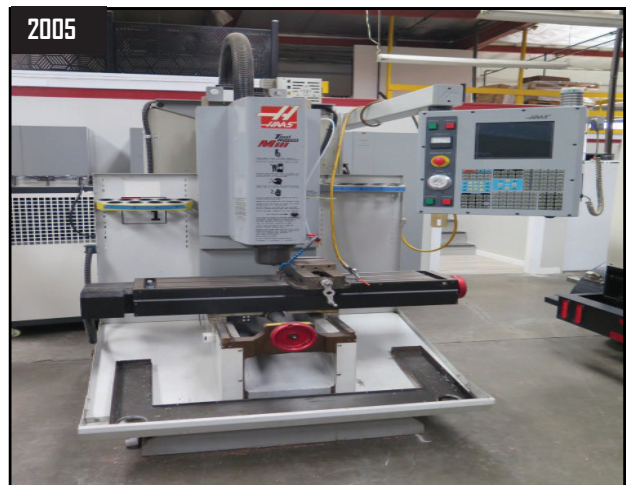
2005 Haas TM-1 CNC Tool Room Mill w/ Haas Controls, CAT-40 Taper Spindle
