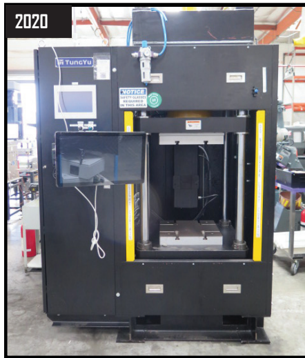
11/2020 Tong Yu TYC-50-E-PCD-UP 50-Ton Servo Driven Compression Molding Press w/ Monitouch Touch Screen Controls
