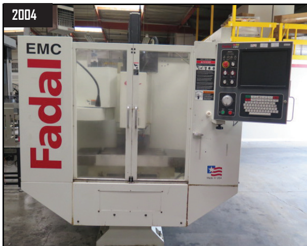
2004 Fadal EMC CNC VMC w/ Multi Processor Controls, 16-Station ATC, 40-Taper Spindle, 7500 RPM
