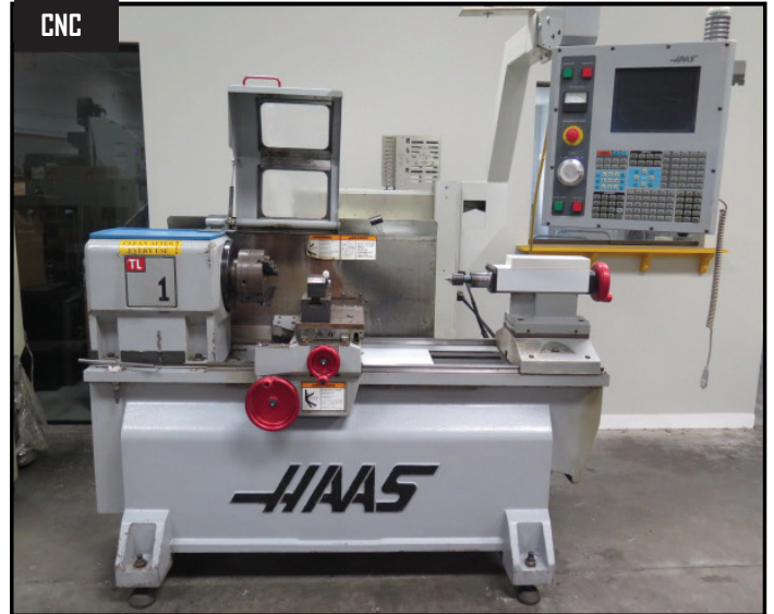
2005 Haas TL-1 CNC Tool Room Lathe w/ Haas Controls, 4000 RPM, Tailstock, KDK Tool Post, 8" Chuck, Intuitive Programming System
