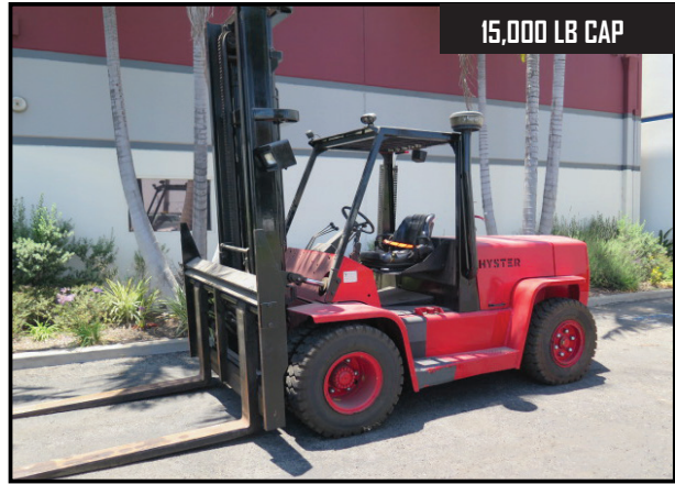
Hyster H155XL2 15,500 Lb Cap Diesel Forklift w/ 2-Stage Mast, 175" Lift Height, Controlled Forks
