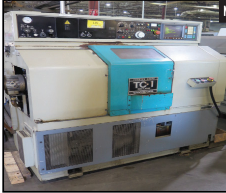
Takisawa TC-1 CNC Turning Center w/ Fanuc Controls, 12-Station Turret, Tailstock, 7" Power Chuck
