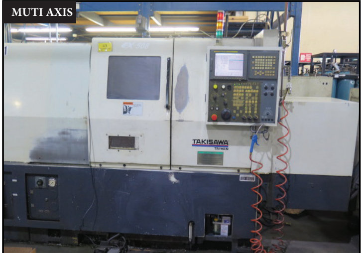
Takisawa EX-508 Twin Spindle CNC Turning Center w/ Fanuc 18i-TB Controls, 12-Station Turret, 8" Power Chucks (Main and Sub Spindles), New "X" Axis Ball Screw (1 Month)
