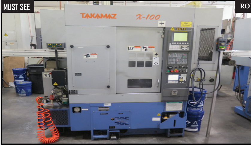
Takamatsu X-100 Robotic CNC Turning Center w/ Fanuc Oi-TC Controls, 8-Station Turret, Robotic Loader / Parts Turner, 6 1/2" 3-Jaw Chuck
