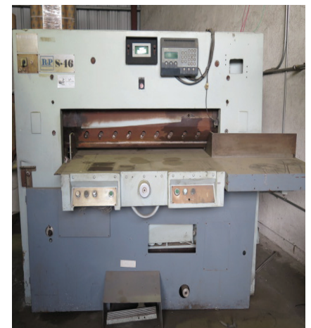
R&P Roberts & Porter mdl. S-46 46" Guillotine Shear w/ Minicut Digital Controls
