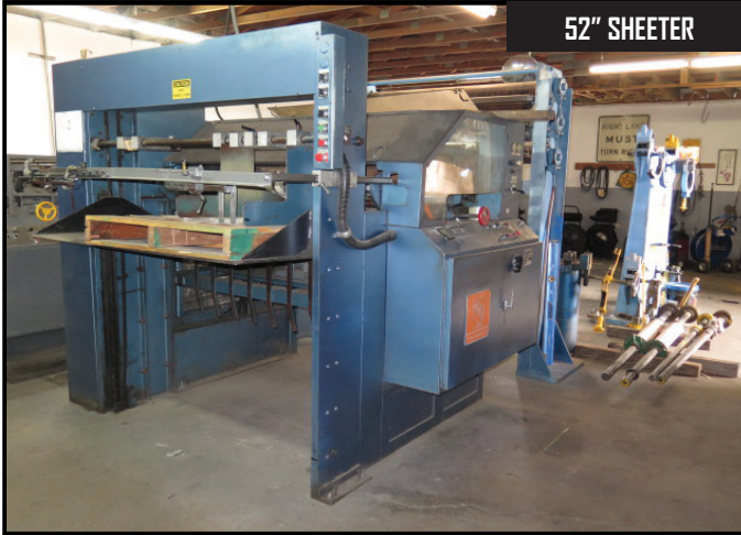
Mamco / Maxon 52" Sheeter w/ M-Line Slitting, (2) Knives, Clark-Aiken Feeder, Decurler, 5-Roll Back-Stand
