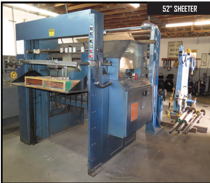
Mamco / Maxon 52" Sheeter w/ M-Line Slitting, (2) Knives, Clark-Aiken Feeder, Decurler, 5-Roll Back-Stand
