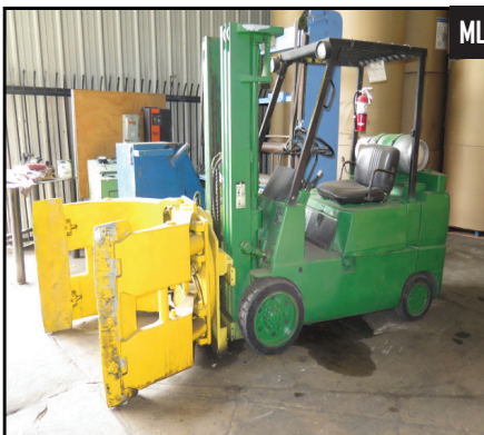
Mitsubishi FGC30 6000 Lb Cap LPG Forklift w/ 2-Stage Mast, 130" Lift Height, Solid Tires, Paper Clamp / Turner
