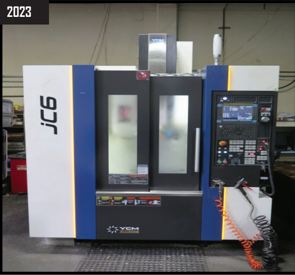
2023 YCM JC6 4-Axis CNC VMC w/ TCM-Fanuc MXP-200 FB Controls, 24- ATC, CAT-40, Marposh Wireless Probe System, Rigid Tapping
