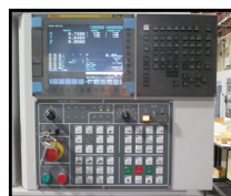
9/2022 Akira Seiki Performa SR3 CNC VMC w/ Fanuc 0i-MF Plus Controls, 20-ATC, CAT-40 Spindle, 11,000 RPM
