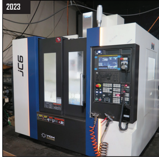
2023 YCM JC6 4-Axis CNC VMC w/ TCM-Fanuc MXP-200 FB Controls, 24- ATC, CAT-40, Marposh Wireless Probe System, Rigid Tapping
