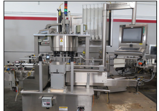
2005 Aylward Dry Tablet High Speed Bottle Lining Machine s/n 133631 w/ Xycon ProFace Touch Screen Controls, "On The Fly" Rejections.
