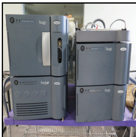
Waters Acquity UPLC System w/ (186015017) Sample Manager - FTN s/n L12SDI 429G, (186015017) UPLC Quaternary Solvent Manager, (186015043) UPLC Column Manager, (186015032) UPLC PDA Detector, Tray Top.
