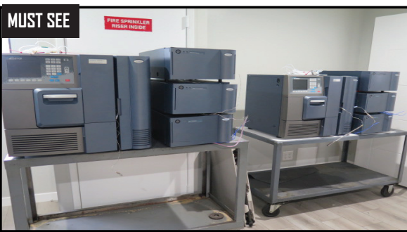
Waters Alliance e2695 HPLC / Sampler Managers. Waters Acquity UPLC System w/ (186015017) Sample Manager - FTN s/n L12SDI 462G, (186015017) UPLC Quaternary Solvent Manager, (186015043) UPLC Column Manager, (186015032) UPLC PDA Detector, Tray Top.
