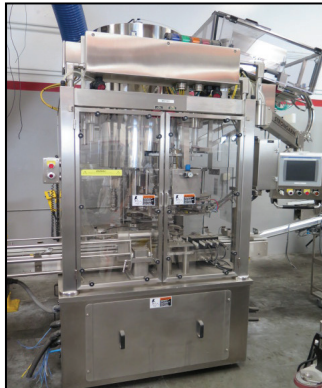
2005 Aylward Dry Tablet High Speed Bottle Lining Machine s/n 133631 w/ Xycon ProFace Touch Screen Controls, "On The Fly" Rejections.
