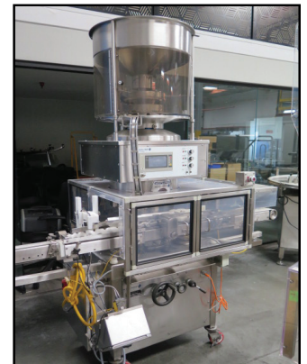
IMA "Flexa AL" 542 Cartoner w/ Allen Bradley PanelView Plus 1250 Controls, (2) ideojet S25 Laser Printers, Video Inspection System, Carton Feeder.
