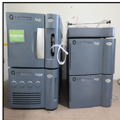
Waters Acquity UPLC System w/ (186015017) Sample Manager - FTN s/n L12SDI 429G, (186015017) UPLC Quaternary Solvent Manager, (186015043) UPLC Column Manager, (186015032) UPLC PDA Detector, Tray Top.
