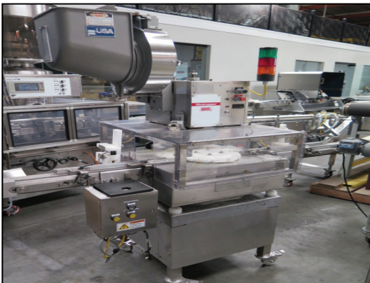
IMA "Flexa AL" 542 Cartoner w/ Allen Bradley PanelView Plus 1250 Controls, (2) ideojet S25 Laser Printers, Video Inspection System, Carton Feeder.
