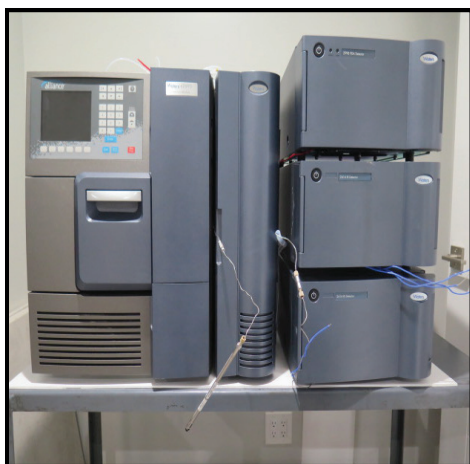
Waters Alliance e2695 HPLC System w/ (186269506) e2695 Separations Module s/n D14SM4113A, (186179100) Column Heater - Cooler, (186299800) 2988 PADetector, (186248900) 2489 UV / Vis Detector, (186241401) 2414 RI Detector.
