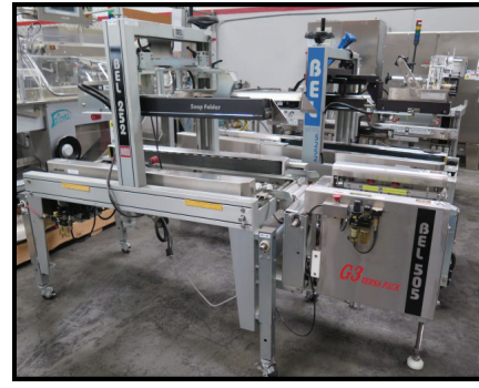
Belcor Carton Erector w/ GS Versa Pack 505 Carton Feeder, Bel 252 Erector, SE-22 Dekka Taping Head.
