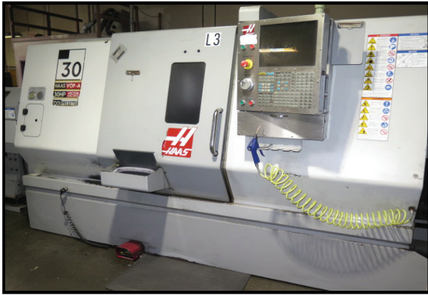
2007 Haas SL-30 CNC Turning Center w/ Tool Presetter, 12-Station Turret, Haas VOP-A, 30Hp, Parts Catcher, 10” Power Chuck
