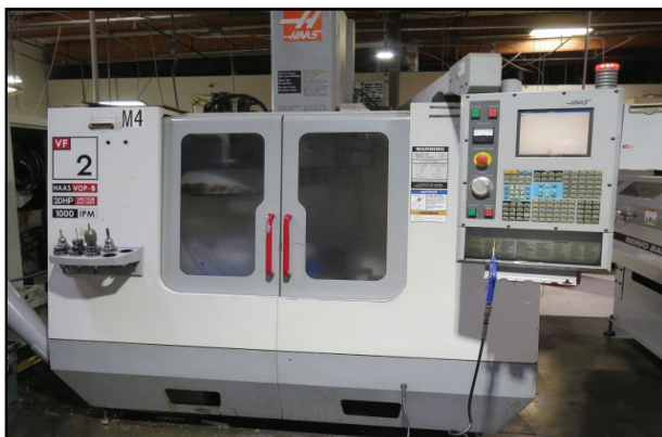
2004 Haas VF-2D 4-Axis CNC VMC w/ 20-Station ATC, CAT-40, 7500 RPM, Rigid Tapping, Haas VOP-B, 20Hp, 1000 IPM
