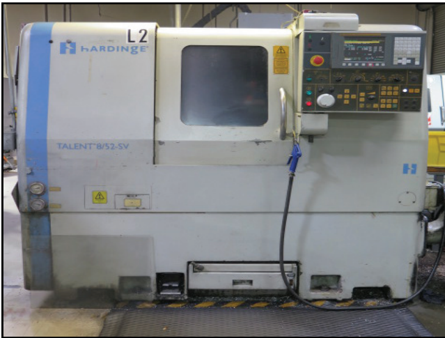
Hardinge Talent 8/52-SV CNC Turning Center w/ Fanuc Controls, 12-Station Turret, 8" Power Chuck
