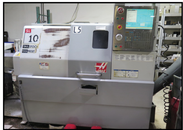
2010 Haas SL-10 CNC Turning Center w/ Tool Presetter, 12-Station Turret, Hydraulic Tailstock, Parts Catcher, 7” Power Chuck
