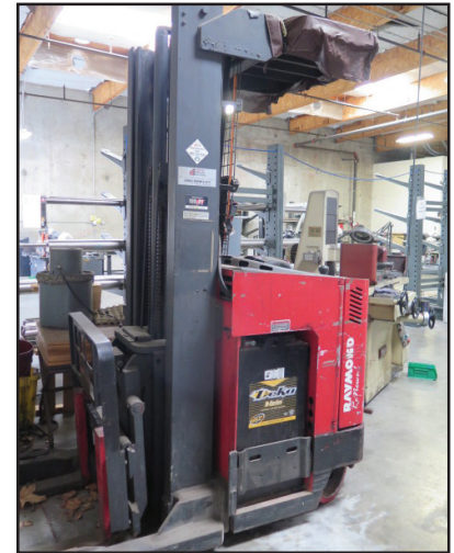
Raymond EASI R 10TT 4500 Lb Cap Stand-In Electric Pallet Mover w/ 188" Lift Height, Extendable Forks, Charger
