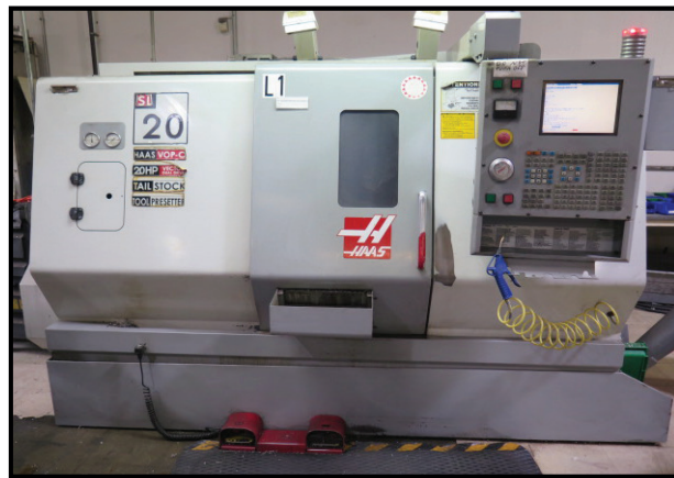
2003 Haas SL-20T CNC Turning Center w/ Tool Presetter, 10-Station Turret, Tailstock, Parts Catcher, Haas VOP-C, 20Hp, 8” Power Chuck
