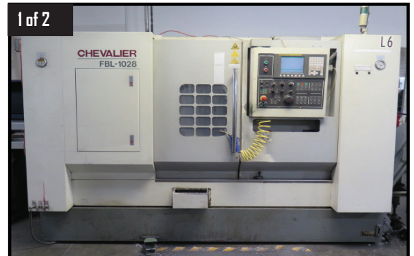
2011 Falcon Chevalier FBL-1028 CNC Turning Center w/ Fanuc 0i-TD Controls, Tool Presetter, 12-Station Turret, Hydraulic Tailstock, 2500 RPM, 12" Power Chuck
