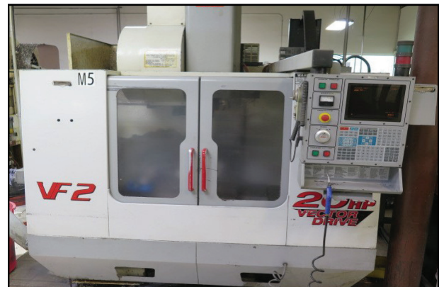
2000 Haas VF-2 4-Axis CNC VMC w/ 24-Station Side Mount ATC, CAT-40, 7500 RPM, Rigid Tapping, Rotation and Scaling, M19, Macros
