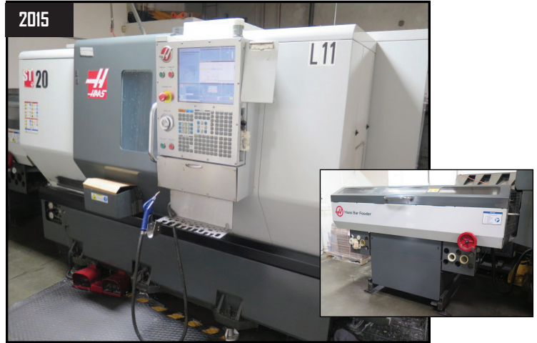
2015 Haas ST-20 CNC Turning Center w/ Tool Presetter, 12-Station Turret, 4000 RPM, Tailstock, Rigid Tapping, Parts Catcher
