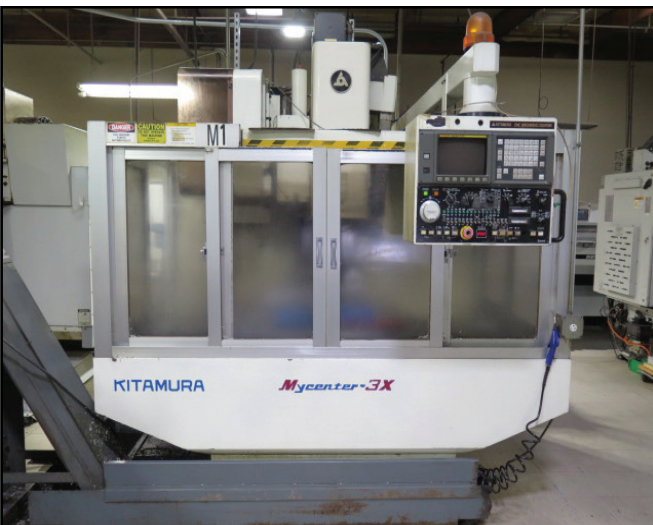
Kitamura Mycenter-3X CNC VMC w/ Fanuc 0-M Controls, 20-Station ATC, CAT-40, 10,000 RPM
