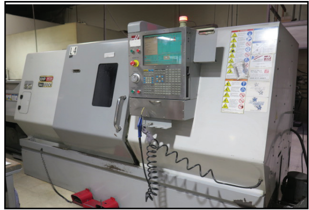
2009 Haas SL-30T CNC Turning Center w/ Tool Presetter, 12-Station Turret, Tailstock, 30Hp, 3400 RPM, Quick Code, 10” Power Chuck
