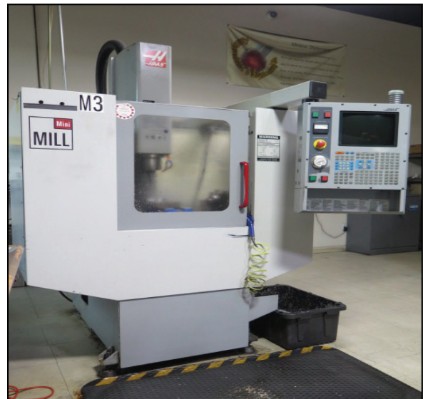
2002 Haas Mini Mill 4-Axis CNC VMC w/ 10-Station ATC, CAT-40, 6000 RPM, Rigid Tapping
