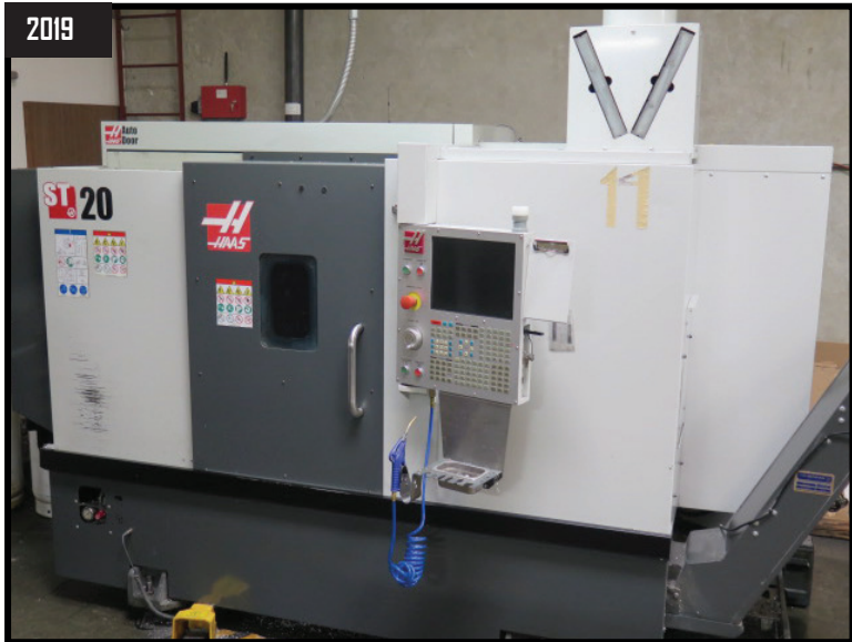
2019 Haas ST-20 CNC Turning Center w/ Tool Presetter, 12-Station Turret, 4000 RPM, Rigid Tapping, 2gb Extended Memory, Wireless Networking, Comp Tables, High Pressure Coolant
