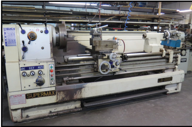
1996 Supermax LG-2680 26" x 80" Geared Head - Gap Bed Lathe s/b BC8509-008 w/ 20-1550 RPM, 4 1/8" Thru Spindle Bore, Inch/mm Threading, Tailstock, Indexing Tool Post, Trava-Dial. 16" 3-Jaw Chuck, Coolant.
