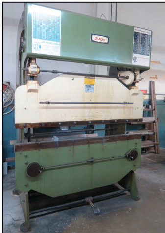
DiAcro 14-72 14GA x 72" Hydrapower Press Brake s/n 6601274122 w/ 72" Bed Length, Manual Back Gauging, 9 1/8" Throat, 62" Between Uprights.
