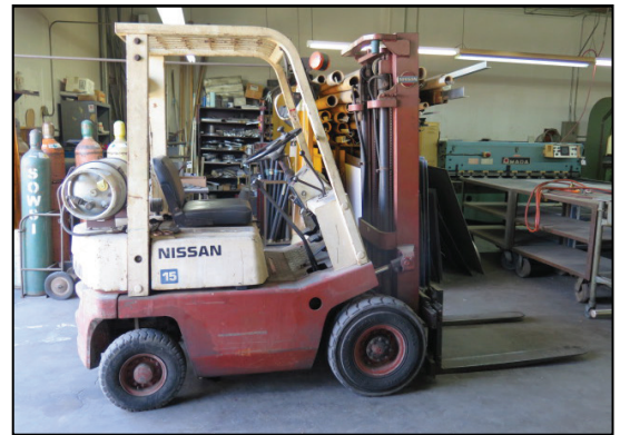
Nissan NF01M15 1500 Lb Cap LPG Forklift s/n NF01-024777 w/ 2-Stage Mast, Side-Shift, Pneumatic Yard Tires. 1500 Lb Cap Shipping Scale.
