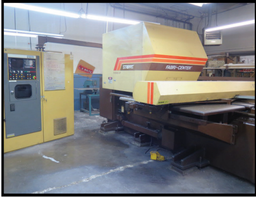
Strippit Fabri-Center FC1000XT 33 Ton 24-Station CNC Turret Punch Press s/n X9038113088C w/ Fanuc GN 6 Series Controls, 24-Station Turret, 29" x 78" Ball-Top Table.
