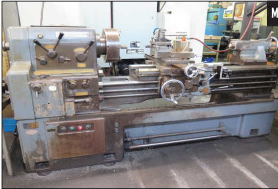
Mori Seiki MS-1250 17" x 52" Geared Head - Gap Bed Lathe s/n 12662 w/ 32-1800 RPM, Inch Threading, Tailstock, Steady and Follow Rests, Trava-Dials, 12" 3-Jaw Chuck, 5C Collet Closer.
