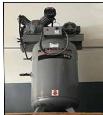
Ingersol Rand T30 Vertical Air Compressor, Piston Style.
