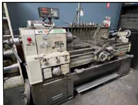
Victor 1640B 16" x 40" Engine Lathe, with Sony DRO, 5C Collet Closer, Tailstock.
