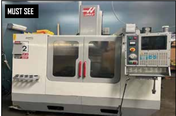
2002 Haas VF-2D CNC VMC, 40 Taper, 20 ATC, 20 HP Vector Dual Drive, Serial # 28476.
