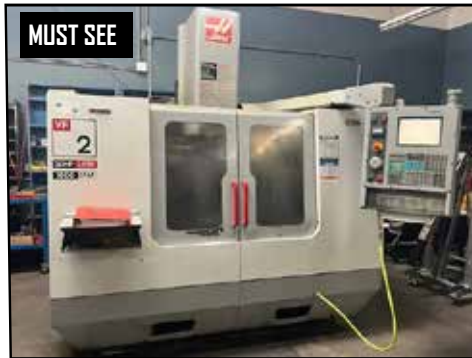
2004 Haas VF-2B CNC VMC, 40 Taper, 20 ATC, 20 HP, 2 Speed Gear Box, Serial #0712
