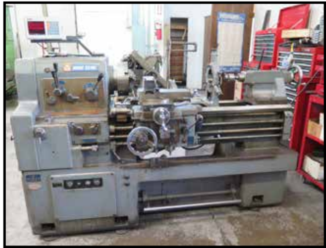
Mori Seiki MS-850G 17" x 36" Geared Head Gap Bed Lathe w/ Sargon MillPro DRO
