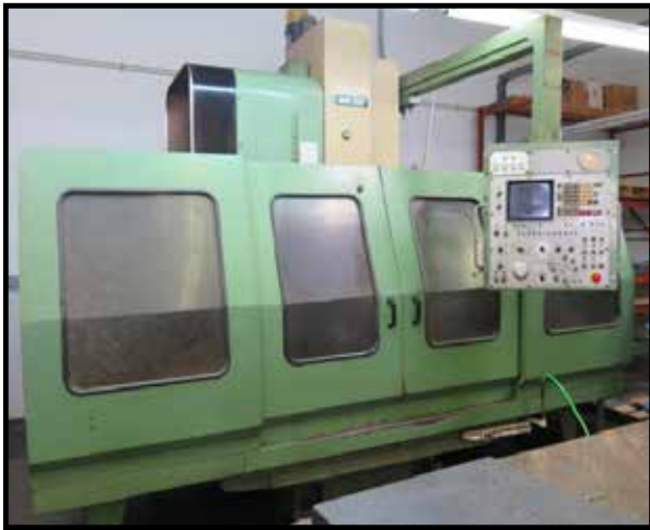
Mori Seiki MV-45 4-Axis CNC VMC w/ Fanuc 6M Controls, 20-ATC, CAT-45 Spindle
