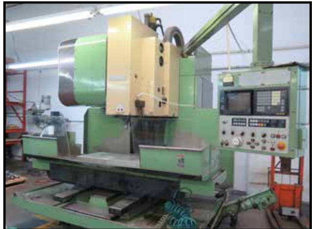
Mori Seiki MV-55 CNC VMC w/ Fanuc 11M Controls, 24-ATC, CAT-50 Spindle
