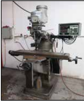
Bridgeport / Proto Trak 2-Axis CNC Vertical Mill w/ SWI Proto Trak Controls, 60-4200 RPM, R8 Spindle
