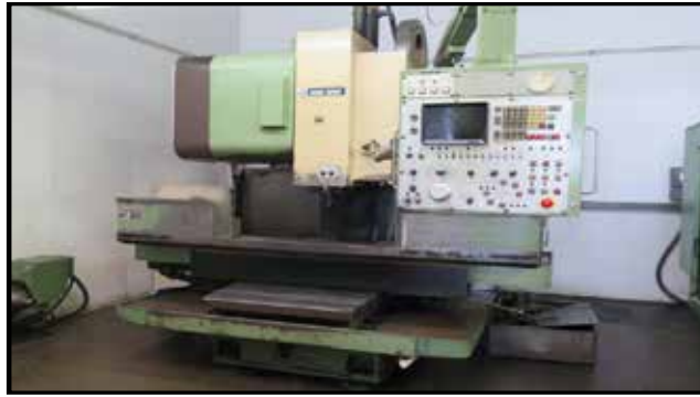
Mori Seiki MV-45 4-Axis CNC VMC w/ Fanuc 6M Controls, 20-ATC, CAT-45 Spindle
